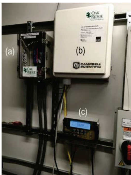
Fig. 11. Instrumentation: (a) power meter, (b) data acquisition system, (c) flow meter display/transmitter unit.
