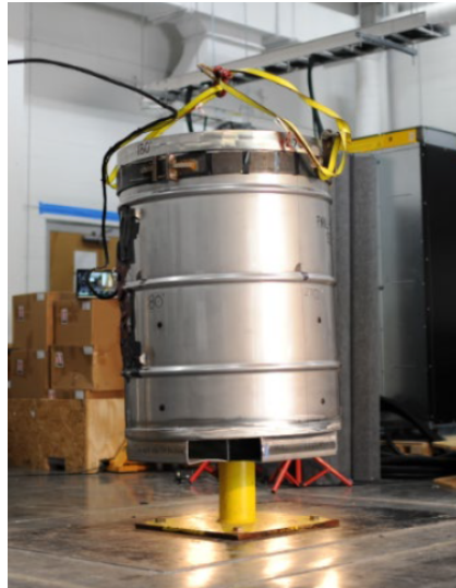
Figure 9. HAC puncture test bar.
