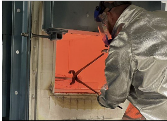
Figure 23. Special form heat test in a standard furnace.
