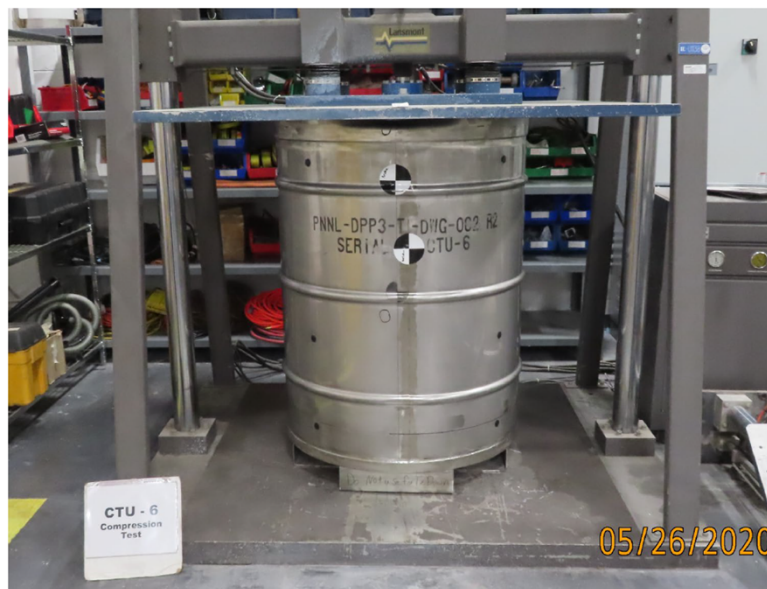
Figure 12. NCT Lansmont compression tester.
