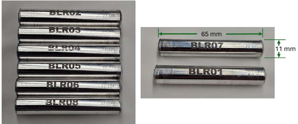
Figure 8. Six Pb rabbits delivered to HFIR that began irradiation in cycle 511 (left) and two rabbits that began in cycle 512 (right).
