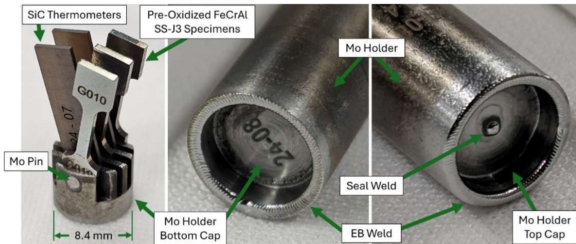
Figure 6. Capsule BLR04 holder bottom end cap assembly (left), EB weld on bottom Mo holder cap (center), and EB weld and seal weld on top Mo holder cap (right).
