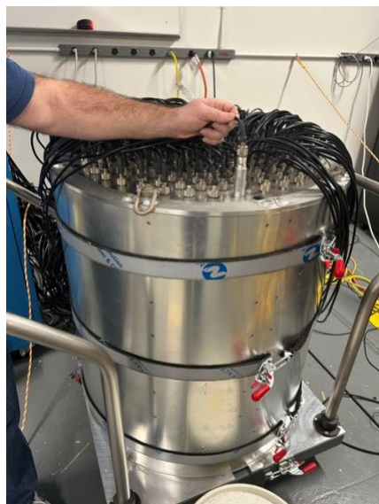
Figure 11. The VPMC detector used in this work to measure individual irradiated TRISO particles.
