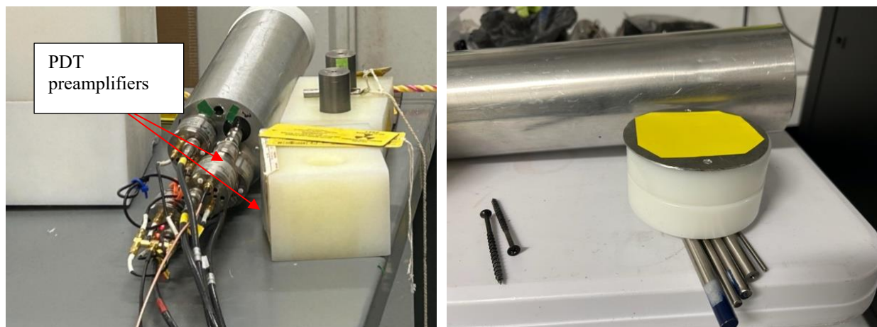
Figure 10. (Left) the neutron detector being tested at ORNL's Safeguards Extension Laboratory using a californium neutron source; (right) the two polyethene disks (1 in. thick each) and the cadmium disk (1 mm thick) added to the neutron detector for the December 2023 experiment.
