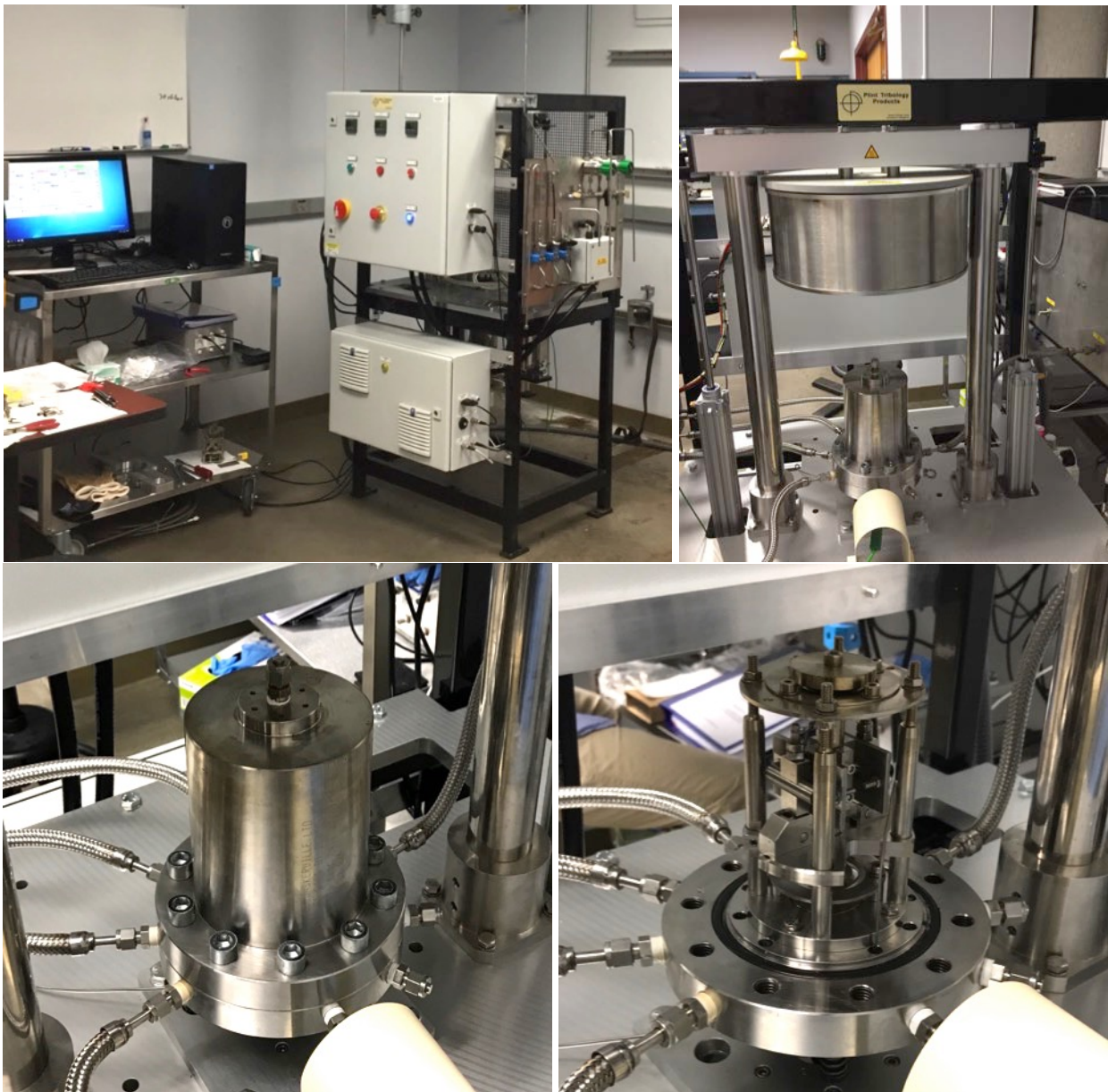
Figure 34. A newly-designed unique autoclave fretting-impact rig at ORNL. (top-left) The AFIR apparatus showing the control unit, power supply, and plumbing; (top-right) The furnace and test chamber behind the panels; (bottom-left) The autoclave vessel with and liquid and gas handling system; (bottom-right) The specimen assembly inside the autoclave chamber. Each run can test two separate grid/cladding pairs of different material and/or contact geometry combinations. A cladding tube frets against two grid dimples, thus producing a total of four wearing grid/clad contacts in each experiment.
