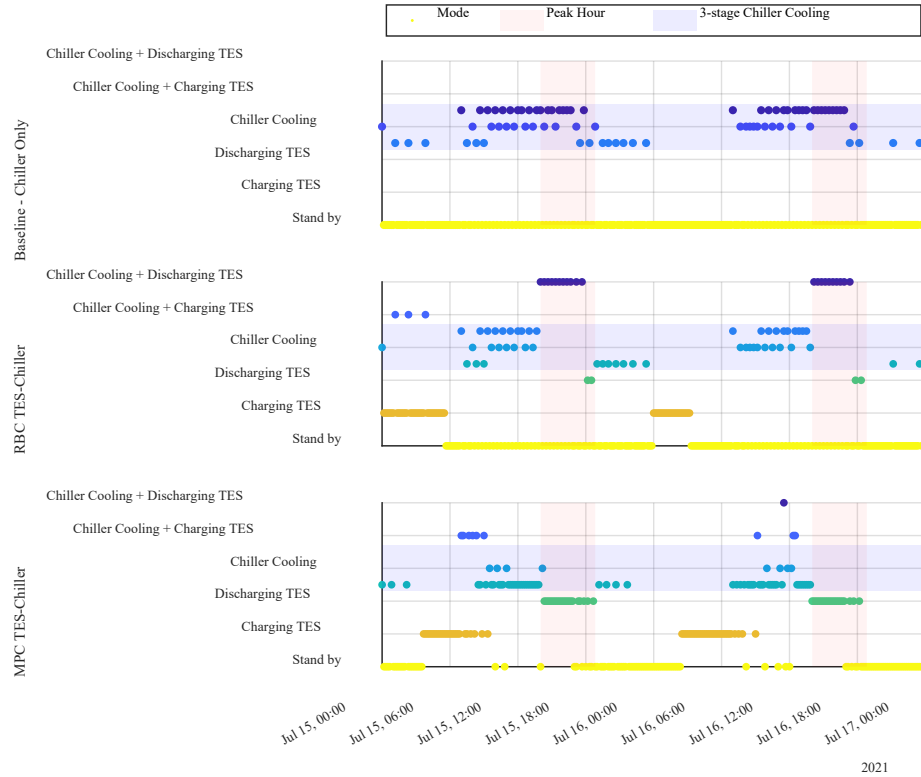
Figure 7: System operation mode of the baseline, RBC-TES system, and MPC-TES system.
