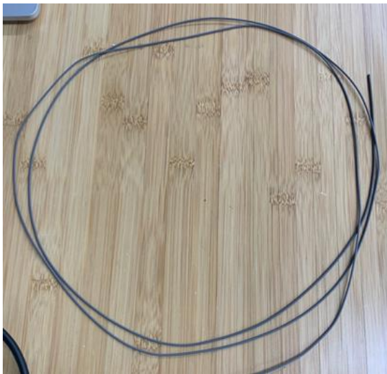
Figure 21. Filament loading 65% by volume fabricated from 14YWT 325 mesh spherical powder
