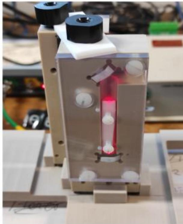
We have the possibility to acquire data with a different radial distance than the magical one, the second periscope is shifted 1.5 cm radial farther ( $R_1$ ) than the central one ( $R_0$ )
