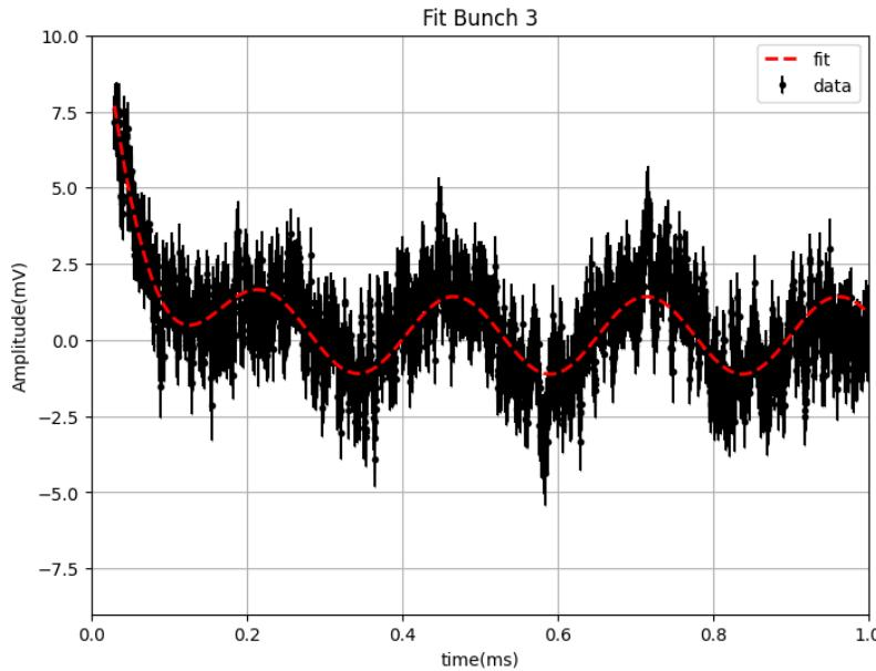
$\omega \approx 1.9 \text{ KHz}$ : **Detector Mechanical Noise**, probably generated by the breadboard vibrations since we see it in all the bunches
