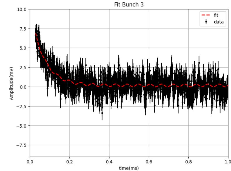
$\omega \approx 17 \text{ KHz}$ : **Kicker Field Oscillation**, causing changes that needs to be accounted for magnetic field. This frequency has been seen also by the UMass magnetometer team with a fiber magnetometer.
