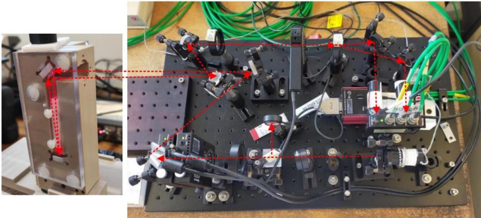
Laser beam path on the breadboard and into the periscope
