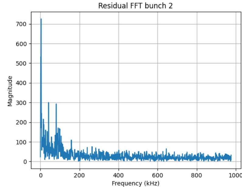
From the residual plot we see an oscillation and from the FFT plot we see at least three **oscillations** at frequencies of 3.8 KHz, 2.8 KHz and 17KHz probably generated by mechanical and electronical noise
