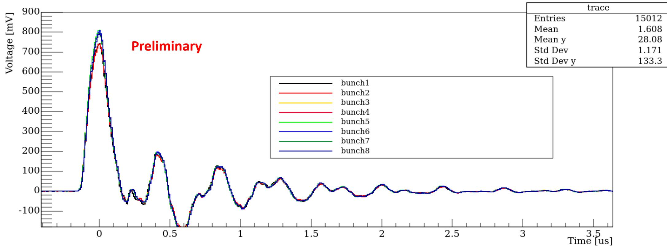
The strength of the kick in 1st and 2nd bunch appears to have a **lower amplitude** than the other ones of a  $\sim 10\%$  factor. ~~Still under investigation~~
