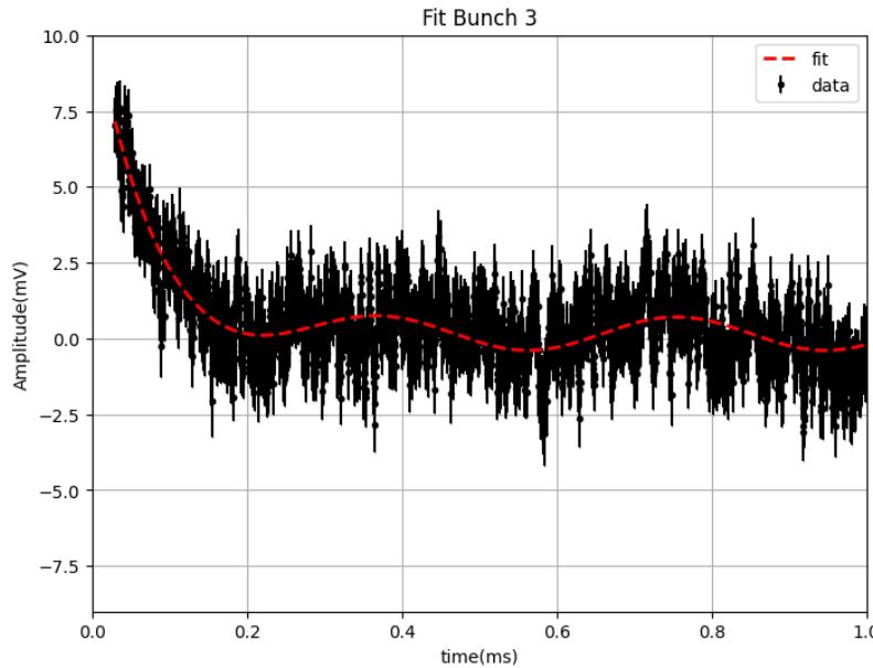
$\omega \approx 3.8 \text{ KHz}$ : **Mechanical Oscillation**, probably generated by periscope bridge vibration, caused by the previous kick arriving, since we do not see it in the first kick but in all the other ones
