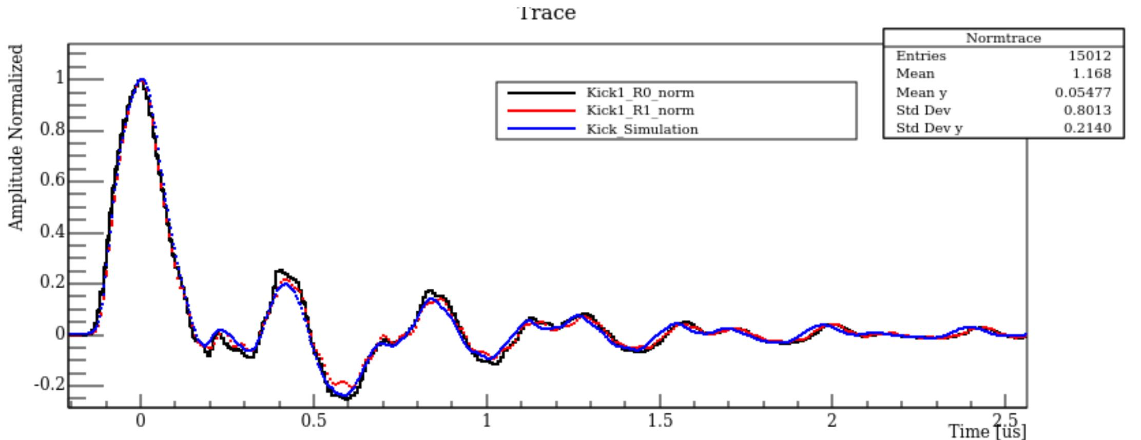
Both  $R_0$  and  $R_1$  normalized 1st kick have the same shape with the kick used in simulation. It confirms the pulse we are using in the simulation is corrected
