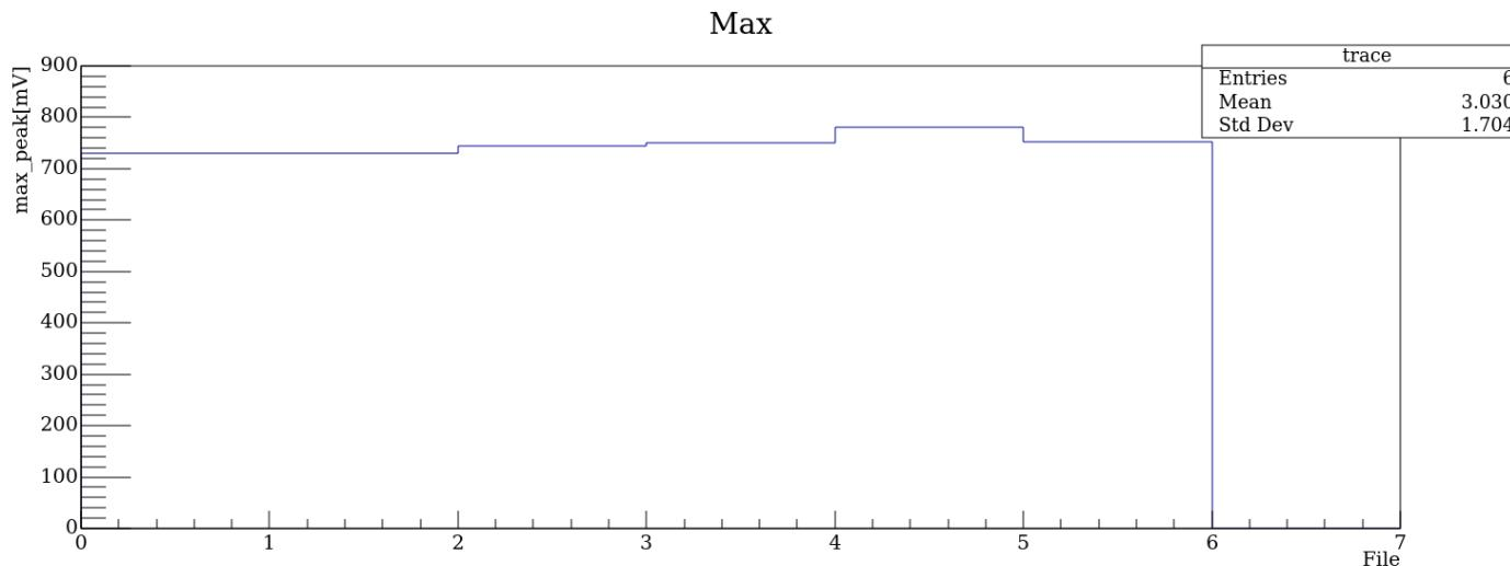
The reason for the lower amplitude of the first two kicks is probably the «heating time» of the kicker system. More statistic would be needed to complete the study
