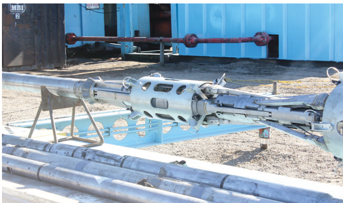
Specialized equipment travels the hole from bottom to top to collect data about the rock layers, their fluids, and their pressures in a technique called wireline logging.
