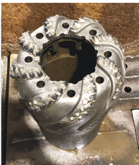
Multiple cylindrical rock samples called cores will be retrieved from three sections of the hole using a specialized coring drill bit.
