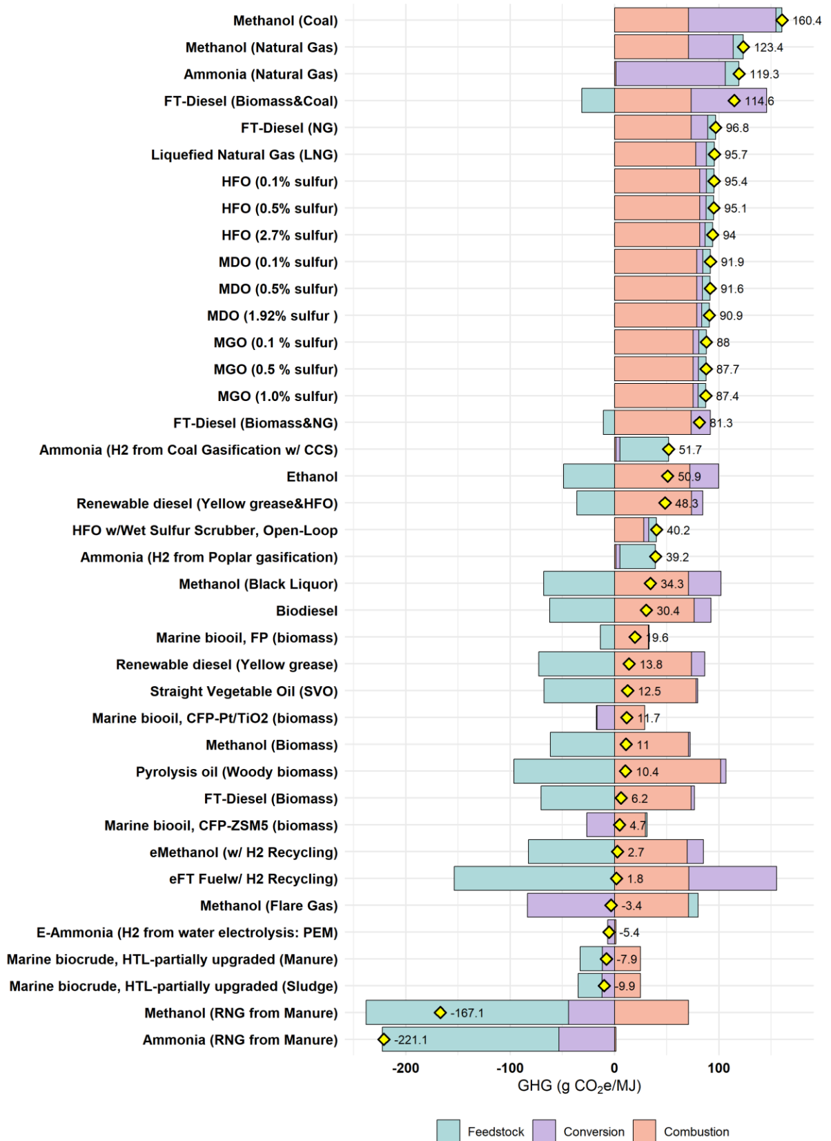
Figure A1. Greenhouse gas (GHG) emission of fuel pathways available in the Marine_Fuel tab; 3 when used in a slow-speed diesel main engine.
