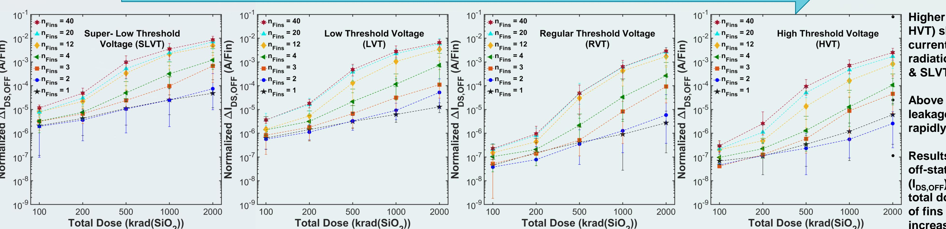
Average off-state drain-source leakage ( $I_{DS, OFF}$ ) current at 0, 100, 200, 500, 1000, and 2000 krad(SiO<sub>2</sub>) of individual n-type transistors with 1, 2, 3, 4, 12, 20, and 40 fins per transistor for SLVT, LVT, RVT, and HVT threshold voltages. Error bars represent the min and max values.
