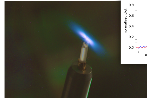
Plasma jets from a copper foil after being hit by Z-Petawatt: Generation of 8.048 keV X-rays.
