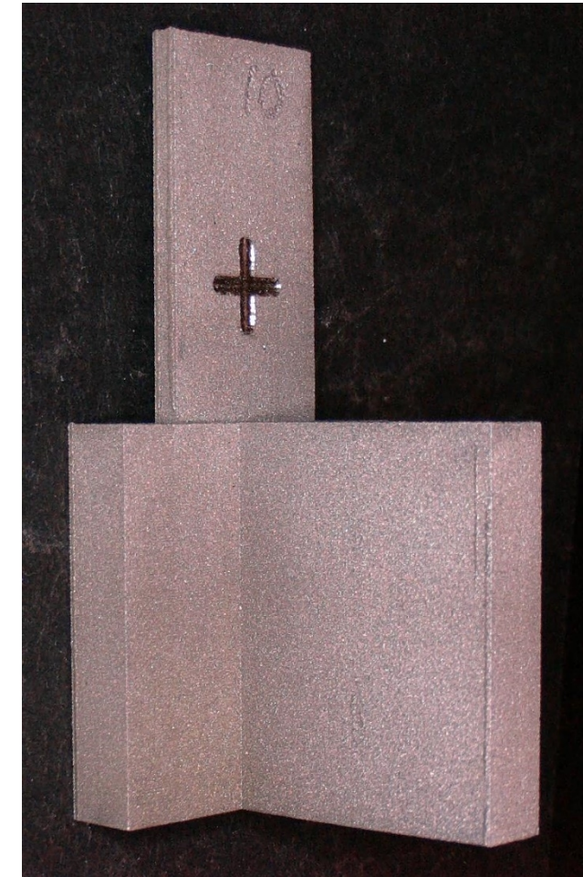
Optical images of T-shaped anodes in the as-printed state
