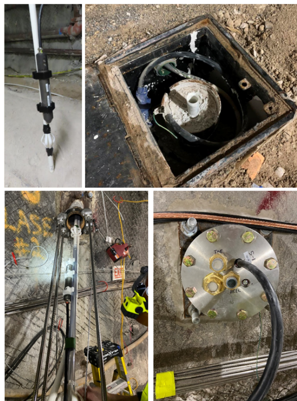
Figure 3-3. Typical: Instruments emplaced in drift vaults and rib collars.
