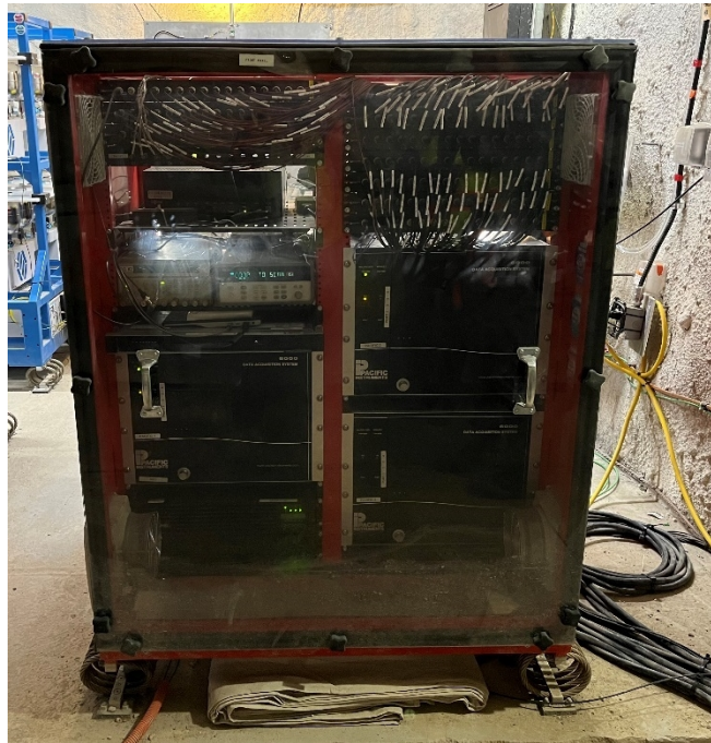
Figure 2-4. Accelerometer DAQ enclosure w/ shock isolators
