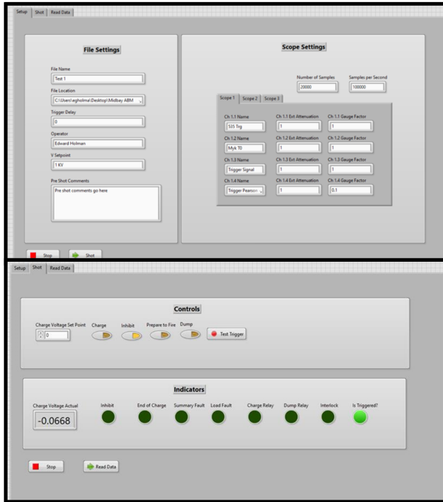
Figure 33: The LabVIEW VI for controlling the ABM system from the Mykonos control station.
