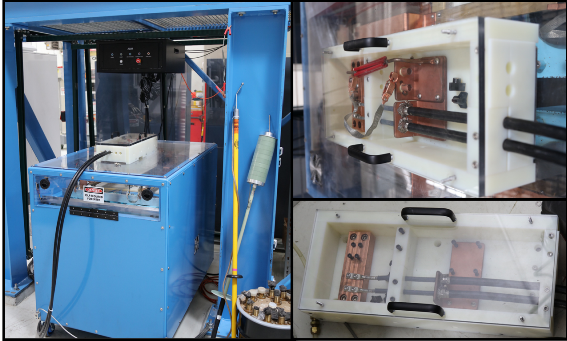
Figure 35: The ABM system deployed to Mykonos, with debris shielding and hard- and soft-grounding sticks (left). The ABM Junction Box for the two output cables (upper right) mounted atop the ABM bank. The Load Junction Box (lower right) in the Laser control room is shown with two input cables from the AJB, but without a connected coil load cable assembly.
