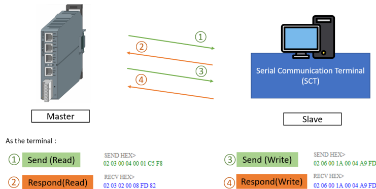
Fig.2-8 Communication between the Modbus RTU master (MGC) and Modbus RTU slave (SCT).
