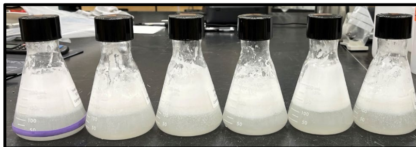
Figure 2-1 250-mL vessel after KTPB was added for shaker oven test. Flasks labeled from left to right: TK48-SH-25C-1-60C-2, TK48-SH-60C-33, TK48-SH-60C-111, TK48-SH-60C-9, TK48-SH-60C-BL, and TK48-SH-25C-3-60C-3.
