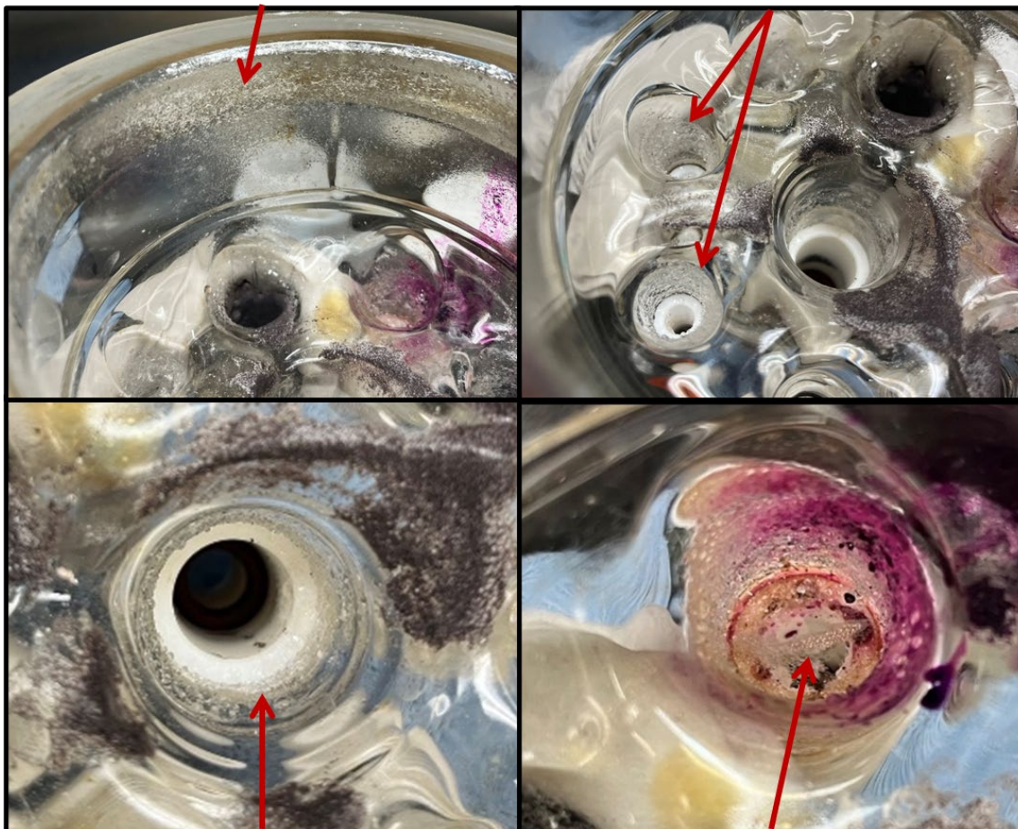
Figure 2-17 Visual observations, indicated by the red arrows, of crystals forming on the lid and vessel for TK48-2LV-60C-3. The permanganate was introduced through the port that is coated in purple.
