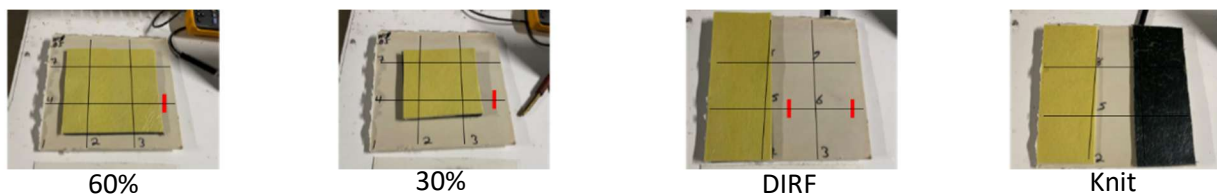
Figure 52. Microscopy Inspection Locations Shown in Red on Charge Placement Images
