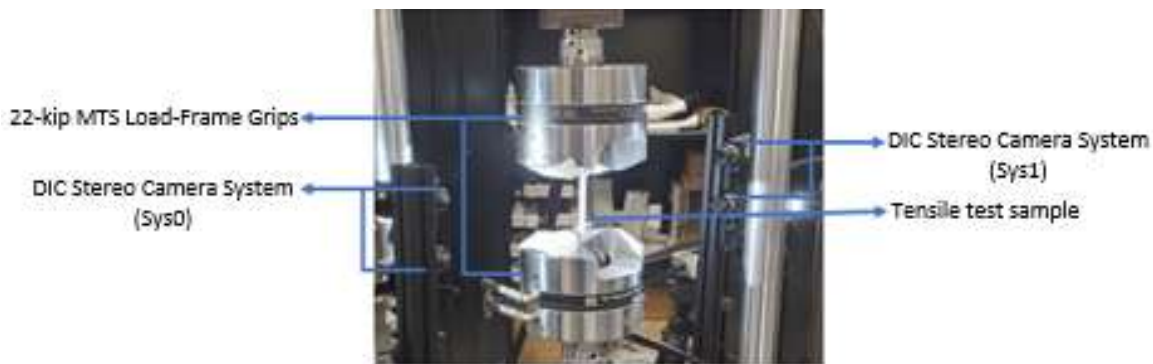
Figure 5. 23°C Tensile Test DIC Mechanism Set-Up
