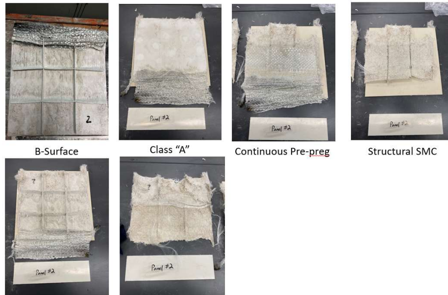
Figure 61. Highlights the material break-down of the 3A directional flow burn-off panel
