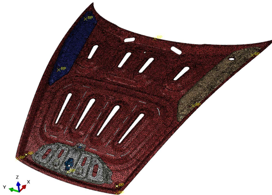
Figure 70. Meshed Aluminum Hood Geometry with All Components and Reference Points
