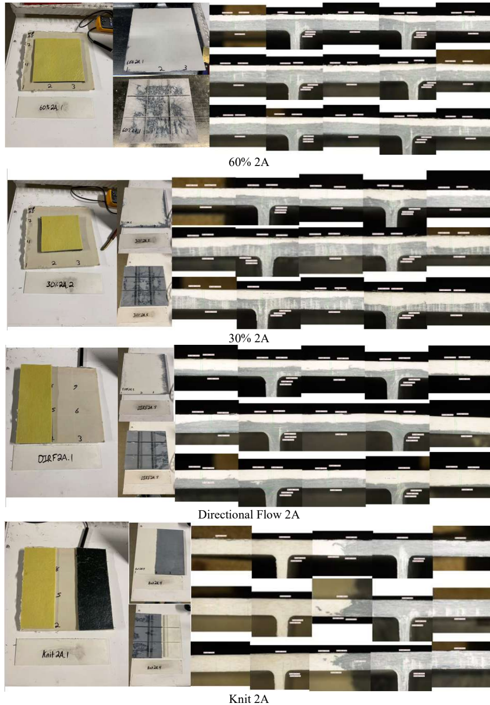
Figure 27 Shows actual 2 component charge patterns, resulting plaques and layer micrographs
