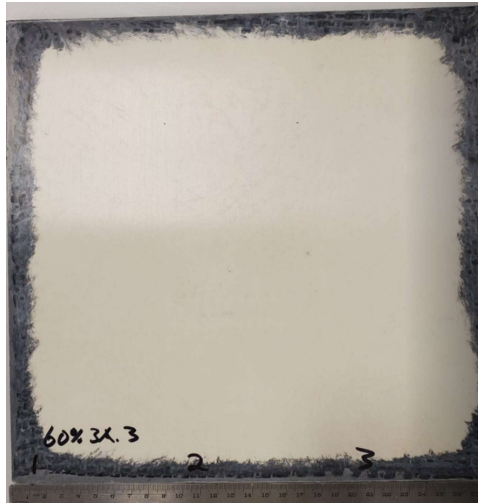
Figure 36. Top View of Ribbed Plate 60% Coverage with 3A Material Combination.
