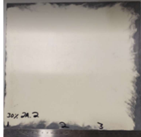
Figure 32. Ribbed Plate Molding Simulation Result for Class A + ½" Structural SMC and Photo of Actual Molded Plate. 30% Coverage. 2A Material Combination.
