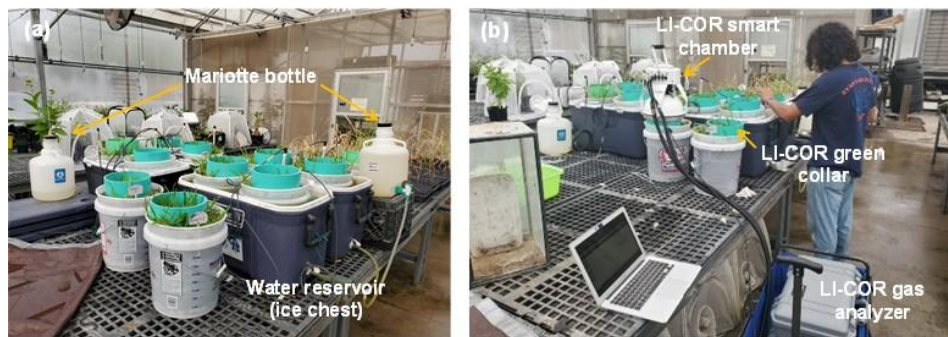
Figure 1. Experiment setup: (a) Water reservoir connected to Mariotte bottle and (b) GHG flux measurements using LI-COR instruments.
