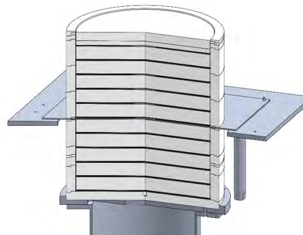
HEU-MET-INTER-013-05 Interstitial hafnium, 1.5 in moderator
