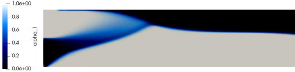
Figure 5.1: Heavy phase volume fraction \alpha_1 : lower-layer occupation and smooth stratified interface.
