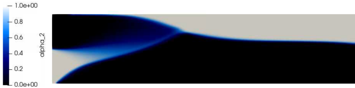
Figure 5.2: Light phase volume fraction \alpha_2 : upper-layer occupation; \alpha_1 + \alpha_2 = 1 everywhere.
