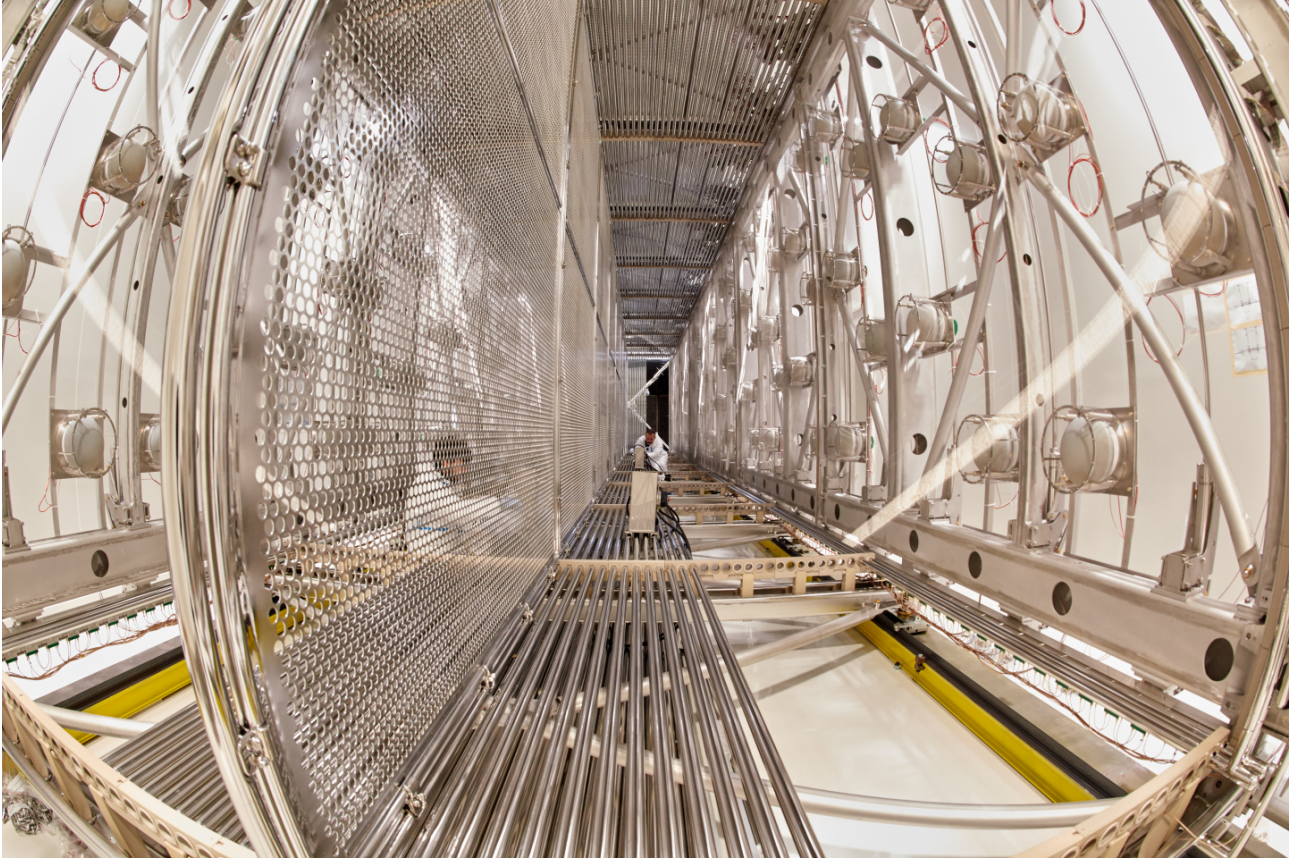
Figure 2.12: Internal view of an ICARUS-T300 module, during the refurbishing activities at CERN. The pierced cathode in the middle separates the two liquid Argon TPCs and the structures holding the 90 PMTs per TPC are visible. Taken from icarus.fnal.gov
