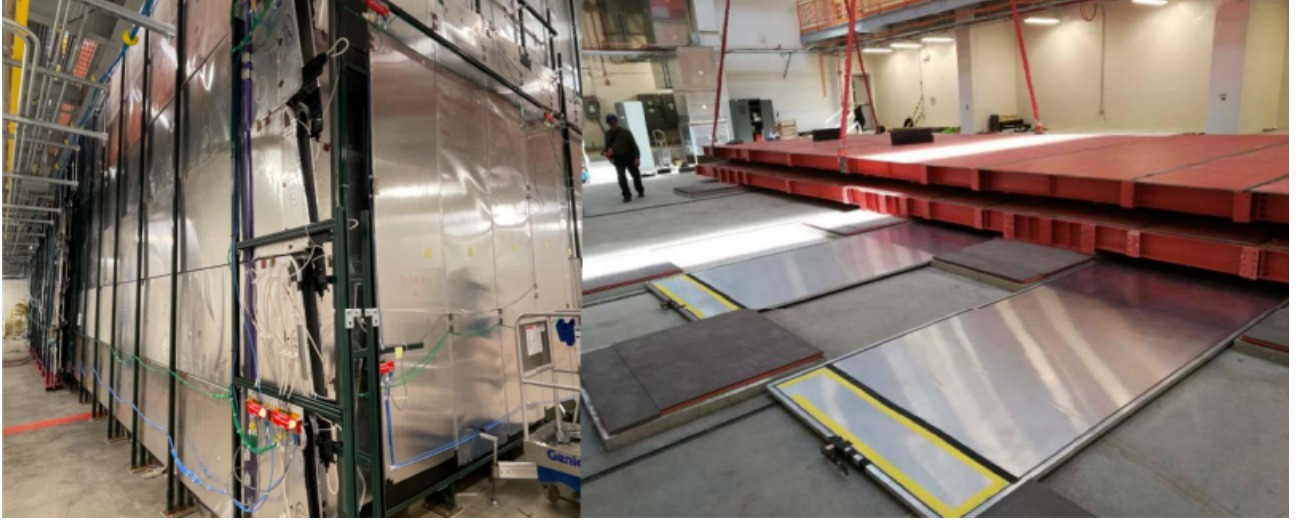
Figure 2.14: On the left, picture of the Side CRT south and west walls seen from the ICARUS building ground pit. On the right, the Bottom CRT module during the warm vessel deployment. From [89].
