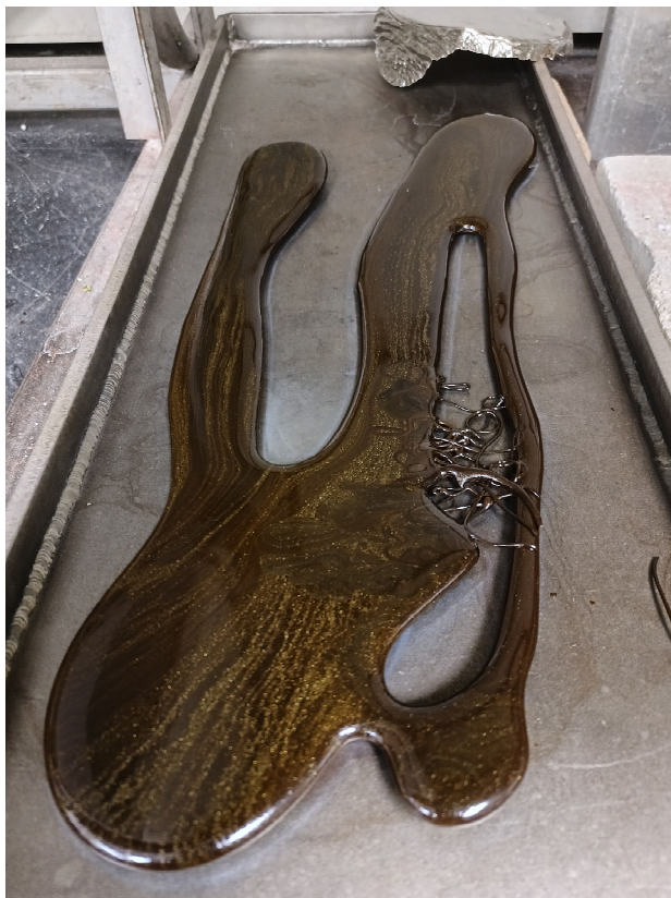
Figure A.16. Photo of Glass HAIG-16 Morphology of Second Melt Stirred at 1400 °C for 1 h
