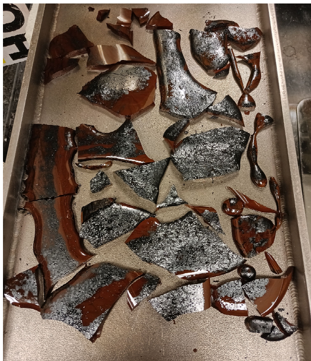
Figure A.10. Photo of Glass HAIG-10 Morphology of Second Melt at 1300 °C for 1 h
