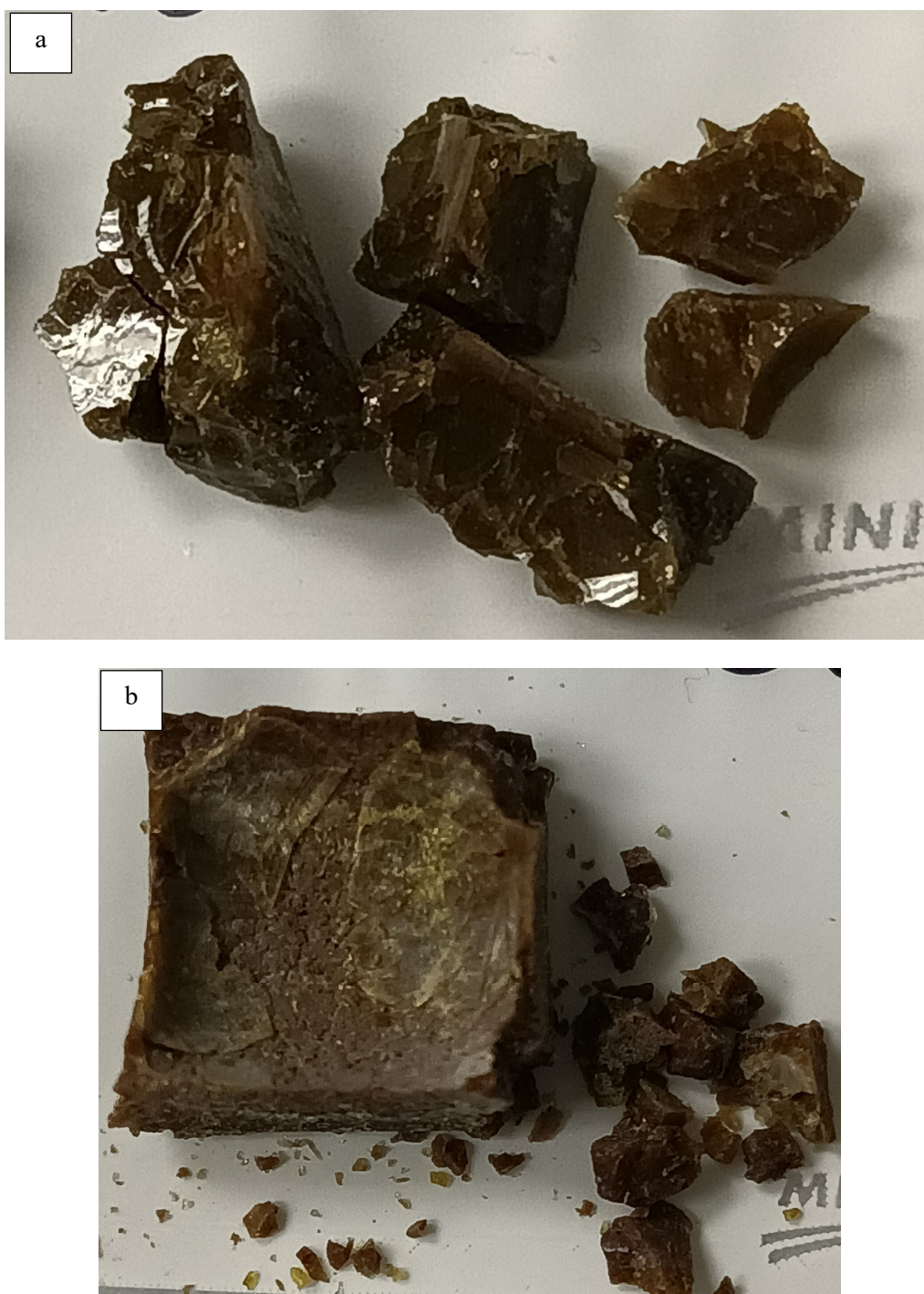
Figure H.17. Glass HAIG-18 after CF Heat Treatment at a) 950 °C for 24 h and b) 850 °C for 48 h
