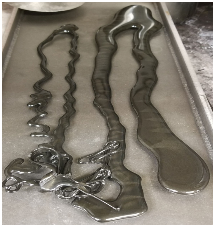
Figure A.8. Photo of Glass HAIG-08 Morphology of Second Melt at 1150 °C for 1 h
