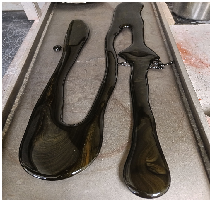
Figure A.2. Photo of Glass HAIG-02 Morphology of Third Melt at 1250 °C for 1 h
