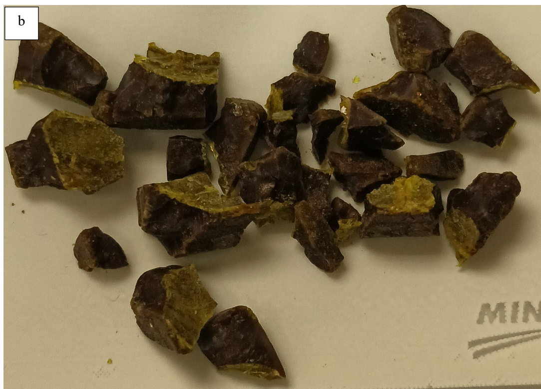
Figure H.10. Glass HAIG-11 after CF Heat Treatment at a) 950 °C for 24 h and b) 850 °C for 48 h
