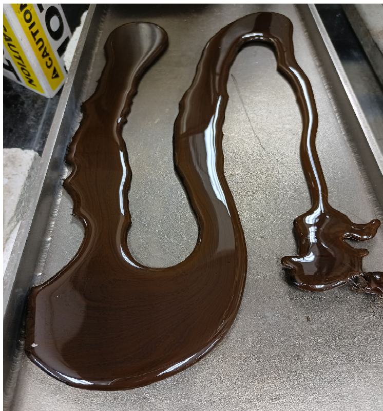
Figure A.13. Photo of Glass HAIG-13 Morphology of Second Melt at 1400 °C for 1 h
