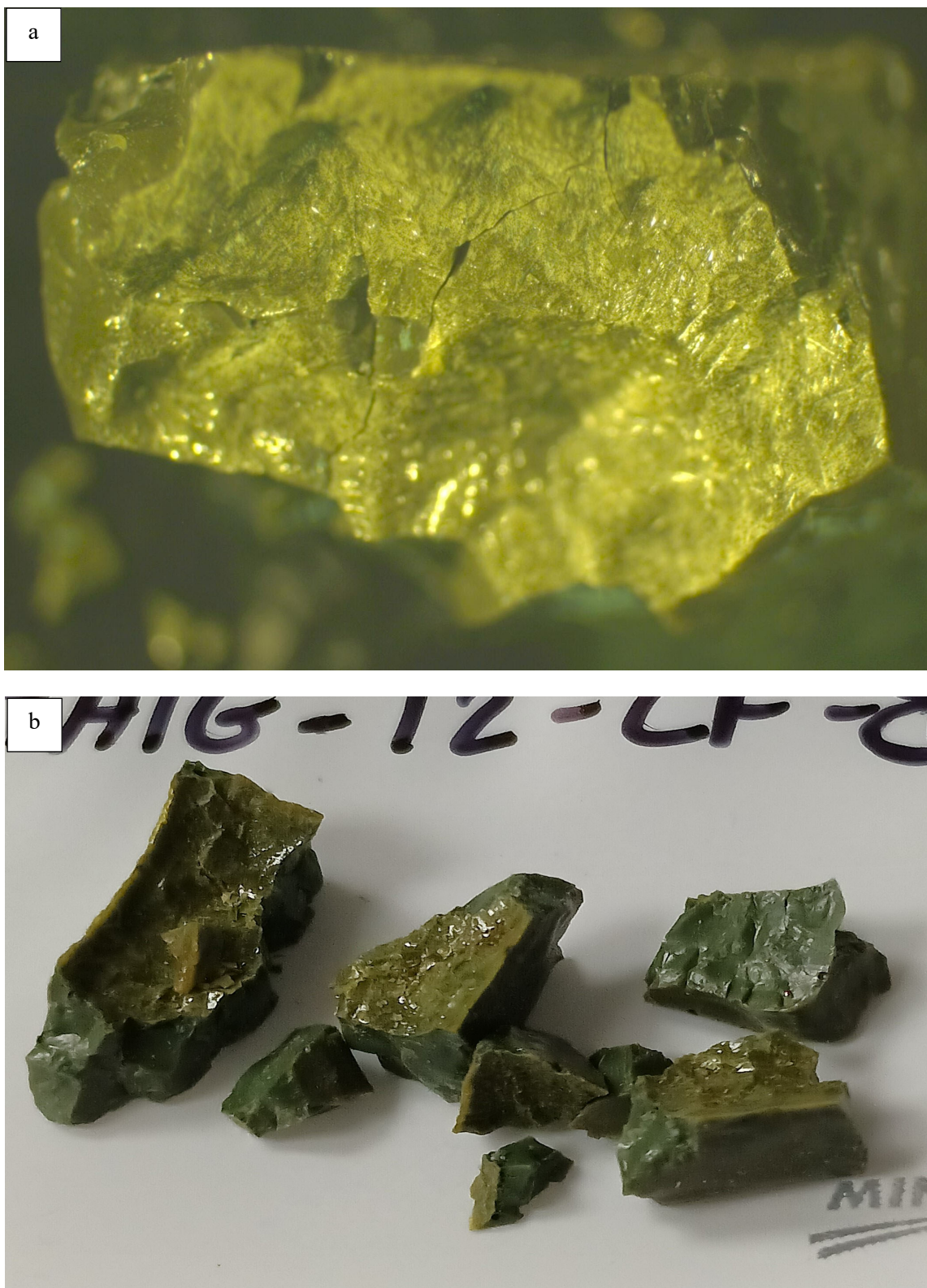
Figure H.11. Glass HAIG-12 after CF Heat Treatment at a) 950 °C for 24 h under the microscope and b) 850 °C for 48 h
