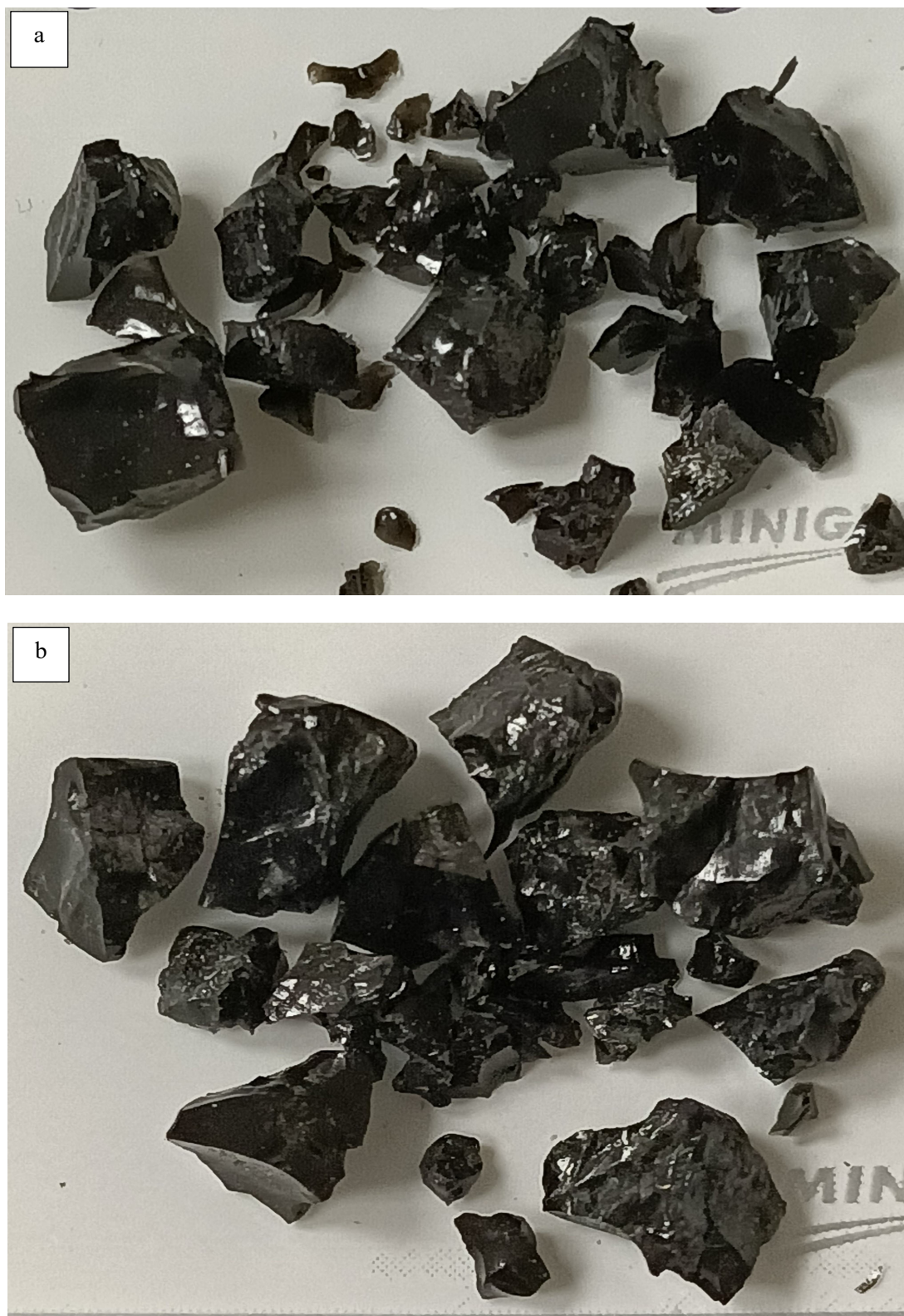
Figure H.23. Glass HAIG-24 after CF Heat Treatment at a) 950 °C for 24 h and b) 850 °C for 48 h
