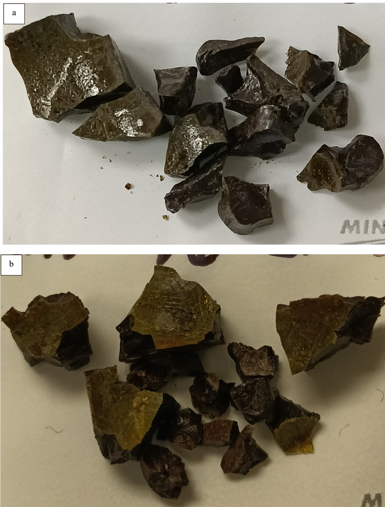
Figure H.15. Glass HAIG-16 after CF Heat Treatment at a) 950 °C for 24 h and b) 850 °C for 48 h
