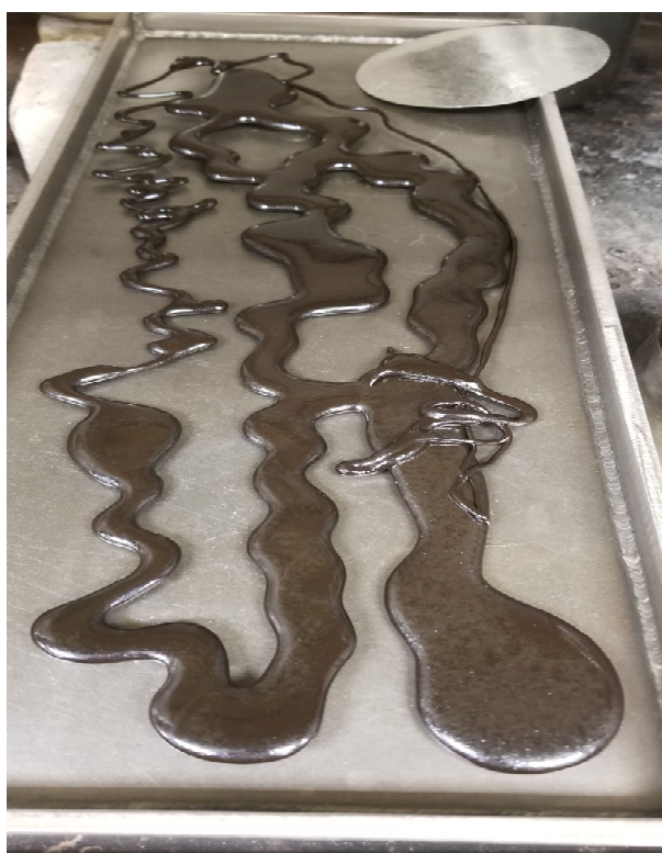
Figure A.15. Photo of Glass HAIG-15 Morphology of Second Melt at 1150 °C for 1 h
