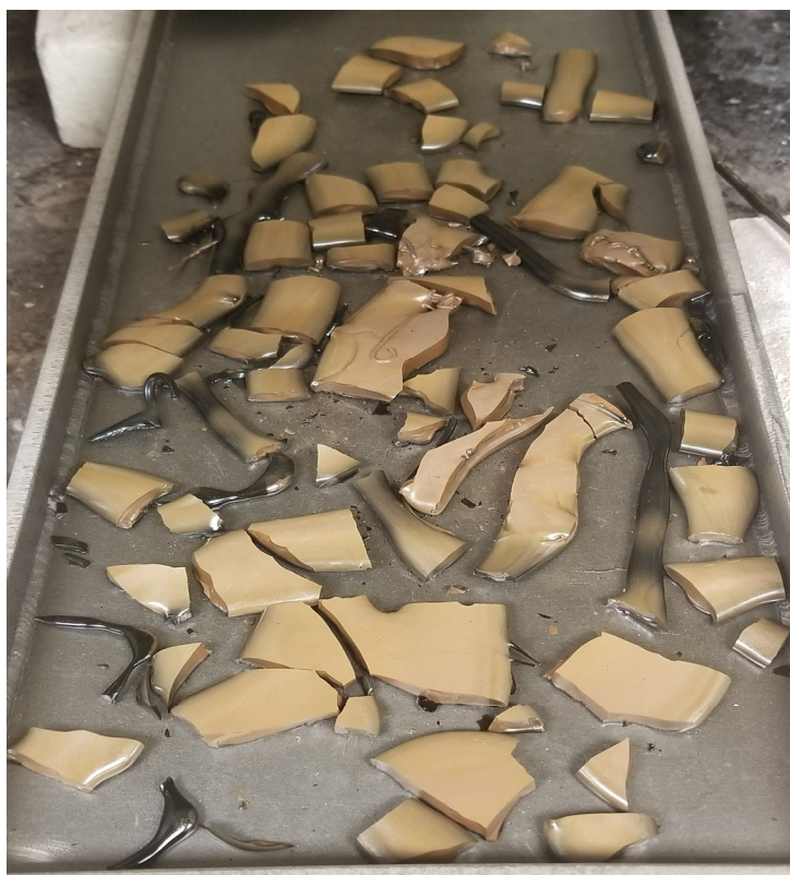
Figure A.21. Photo of Glass HALG-21 Morphology of Second Melt at 1150 °C for 1 h
