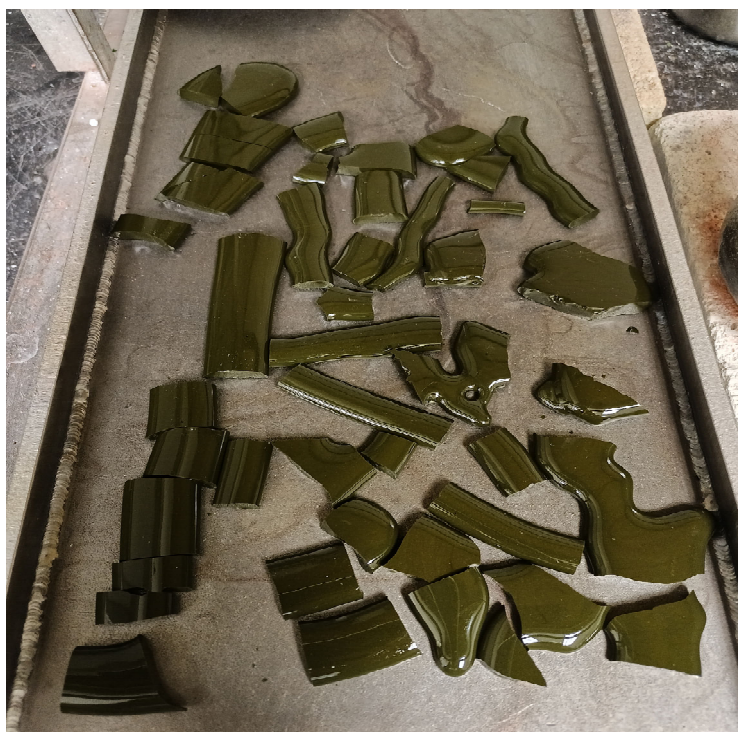
Figure A.6. Photo of Glass HAIG-06 Morphology of Second Melt at 1150 °C for 1 h
