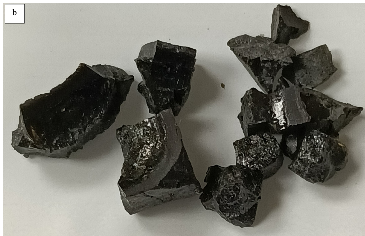
Figure H.20. Glass HAIG-21 after CF Heat Treatment at a) 950 °C for 24 h and b) 850 °C for 48 h
