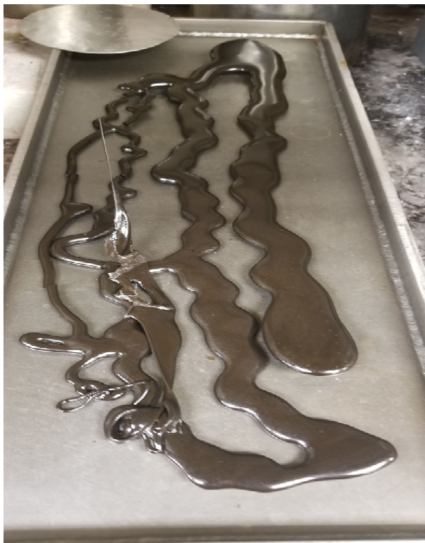
Figure A.22. Photo of Glass HAIG-22 Morphology of Third Melt at 1150 °C for 1 h
