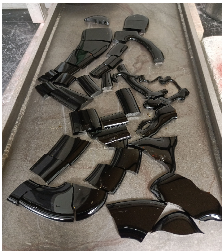
Figure A.3. Photo of Glass HAIG-03 Morphology of Fourth Melt at 1250 °C for 1 h
