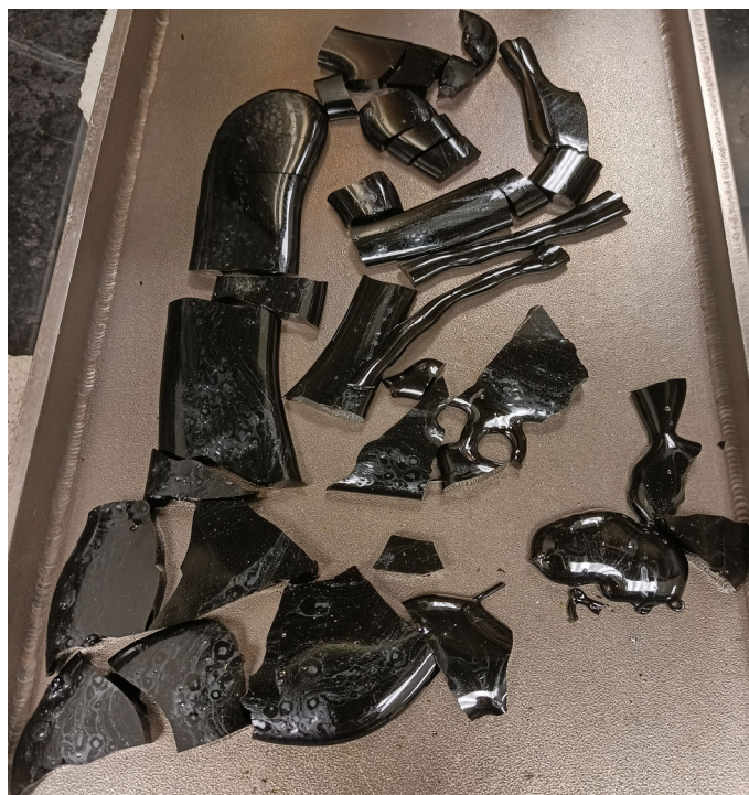
Figure A.7. Photo of Glass HAIG-07-1 Morphology of Fourth Melt at 1200 °C for 1 h
