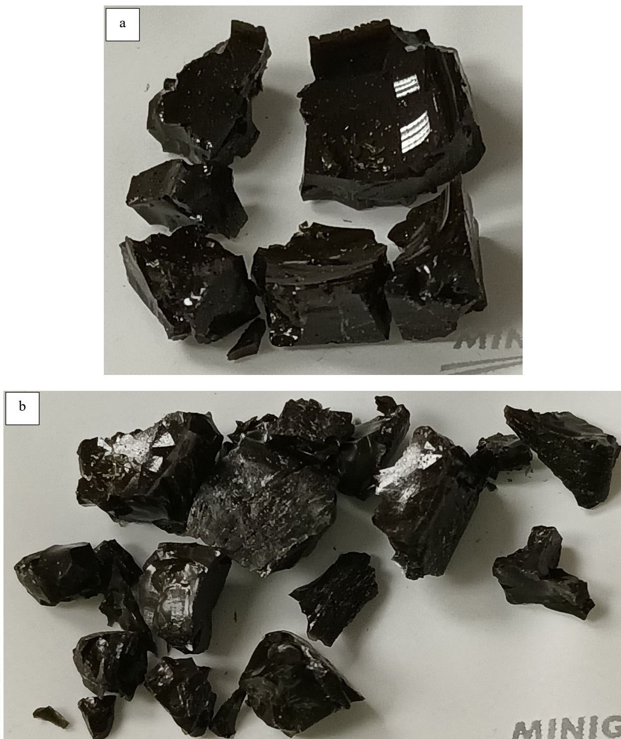
Figure H.6. Glass HAIG-06 after CF Heat Treatment at a) 950 °C for 24 h and b) 850 °C for 48 h
