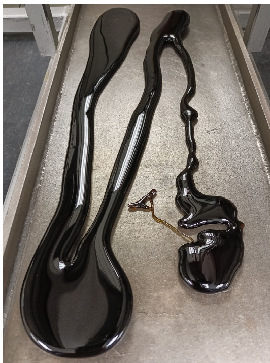
Figure A.17. Photo of Glass HAIG-17 Morphology of Third Melt at 1200 °C for 1 h
