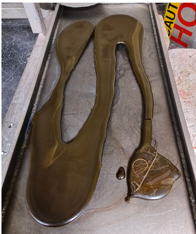
Figure A.11. Photo of Glass HAIG-11 Morphology of Third Melt at 1350 °C for 1 h
