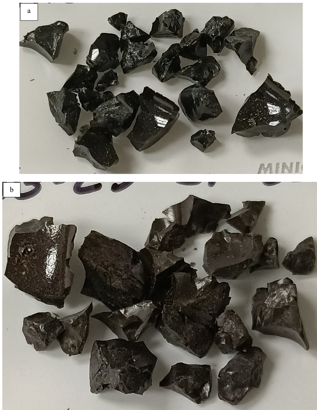
Figure H.24. Glass HAIG-25 after CF Heat Treatment at a) 950 °C for 24 h and b) 850 °C for 48 h
