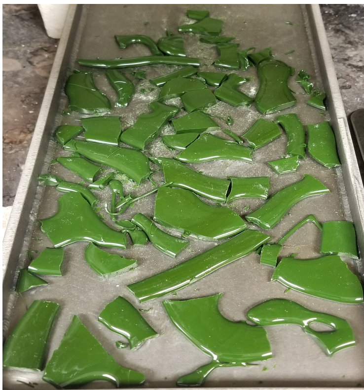
Figure A.23. Photo of Glass HAIG-23 Morphology of Second Melt at 1150 °C for 1 h
