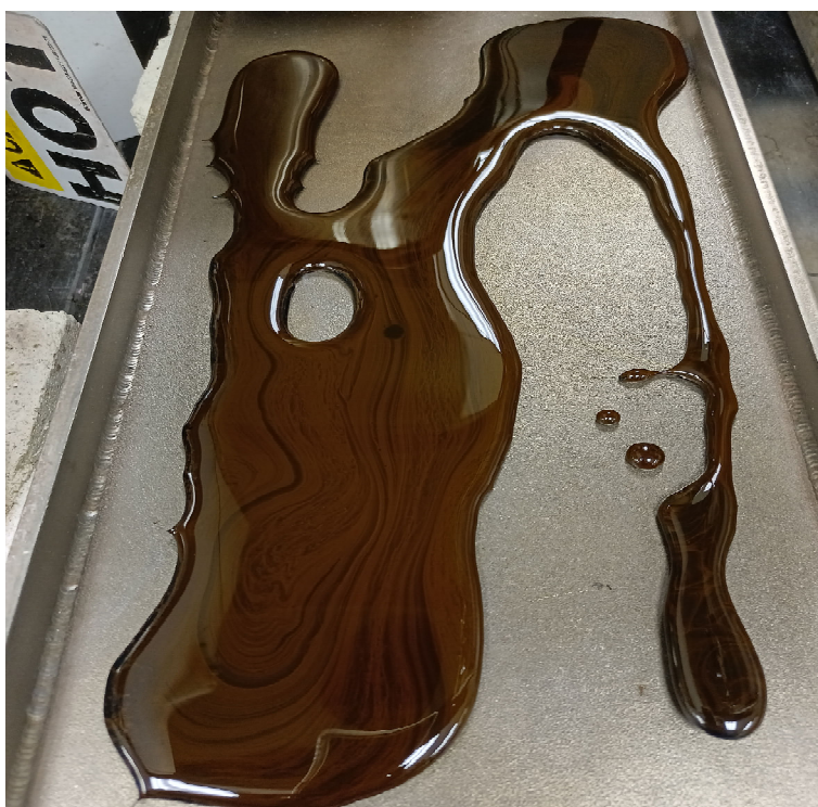
Figure A.9. Photo of Glass HAIG-09 Morphology of Fourth Melt at 1400 °C for 1 h
