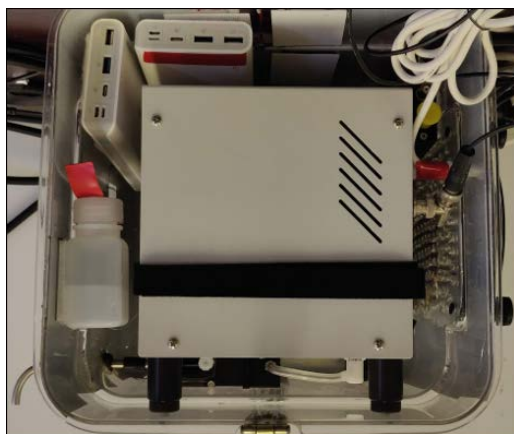
Figure 22. Enclosure with MAGIC CPC and system peripherals installed.
