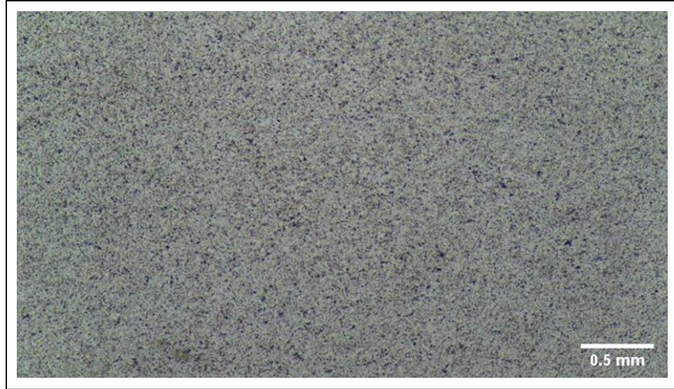
Figure 29: High magnification image of the dried micromodel surface after Illite-clay coating
