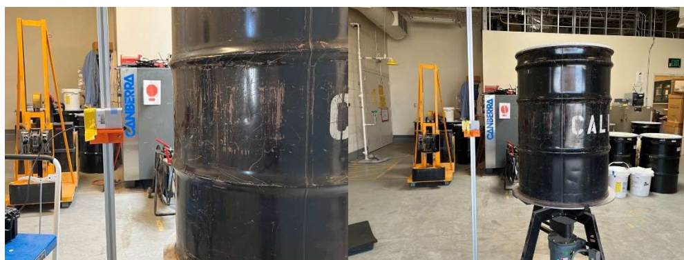
Figure 17. Fiberboard rotating drum measurement setup using the H3D M400 at a distance of 25 cm from the skin of the drum.
