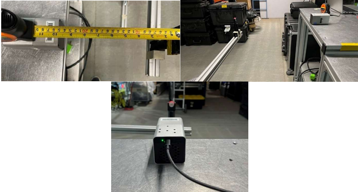
Figure 24. Measurement setup for M400 DRF generation at 25 cm.
