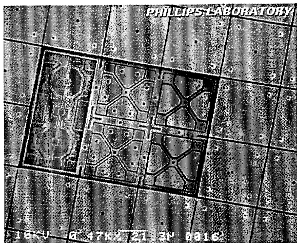
Figure 4. SEM image of an Axial-Rotation Micromirror Device where six mirror elements are shown with the upper layers removed to illustrate the design by process layers. Surrounding the six uncovered elements is the normal field of individually addressable micromirror devices which illustrates the current fill-factor ( >98\% ). (Courtesy of USAF Phillips Laboratory)
