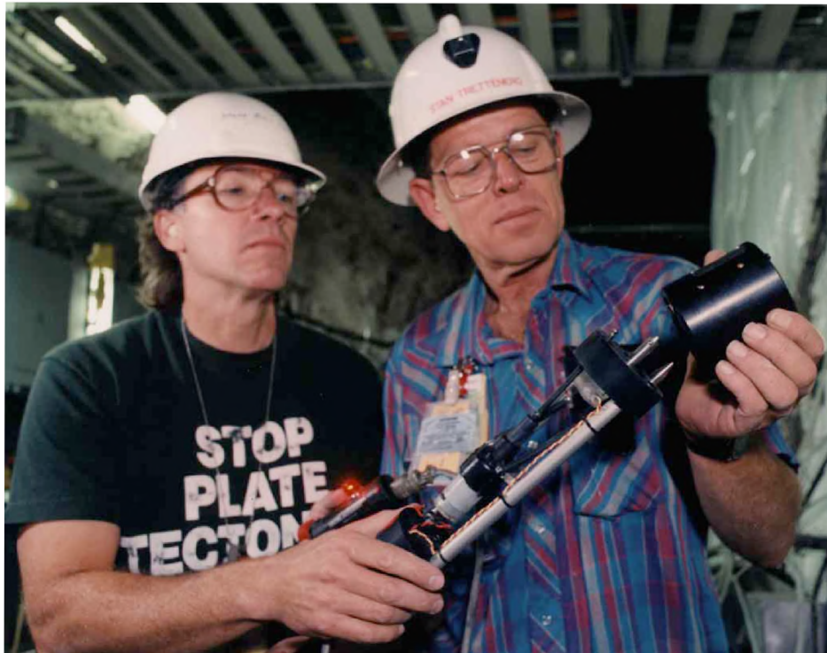
Figure 5-5. Borehole anchor and installation tool prior to installation in the SHT
