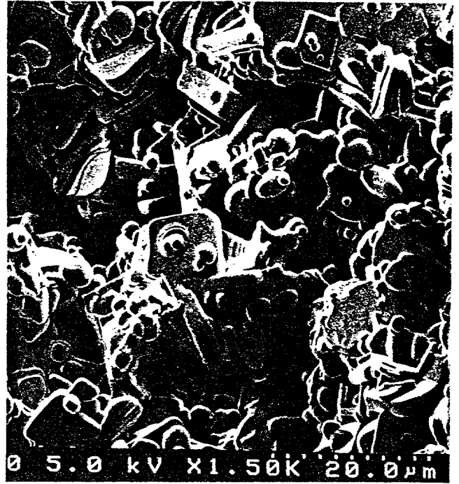
Fig. 5. SEM micrograph of the TI-2223 superconductor illustrating the platelet formation.
