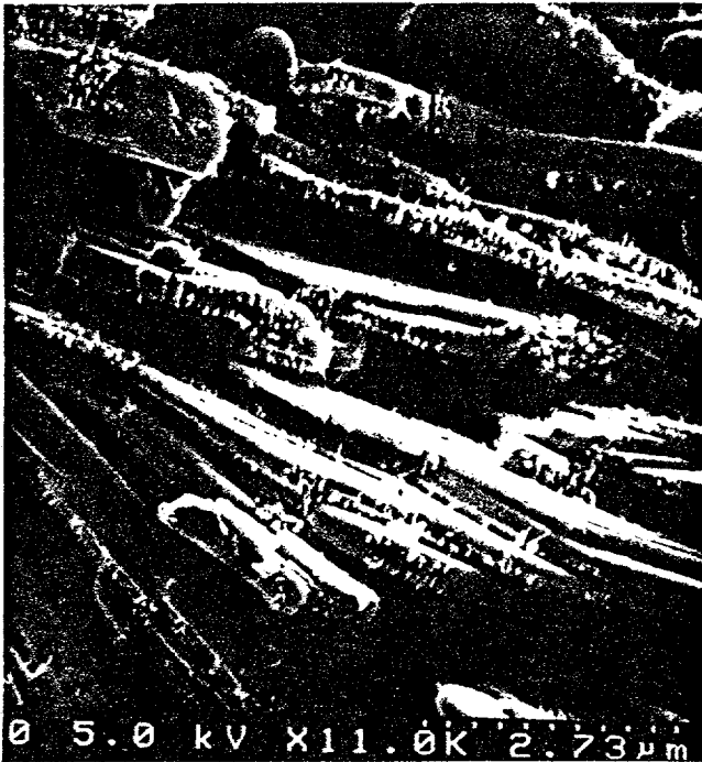
Fig. 3. SEM micrograph of the mixture of TI-1212 and TI-1223 superconductors.
