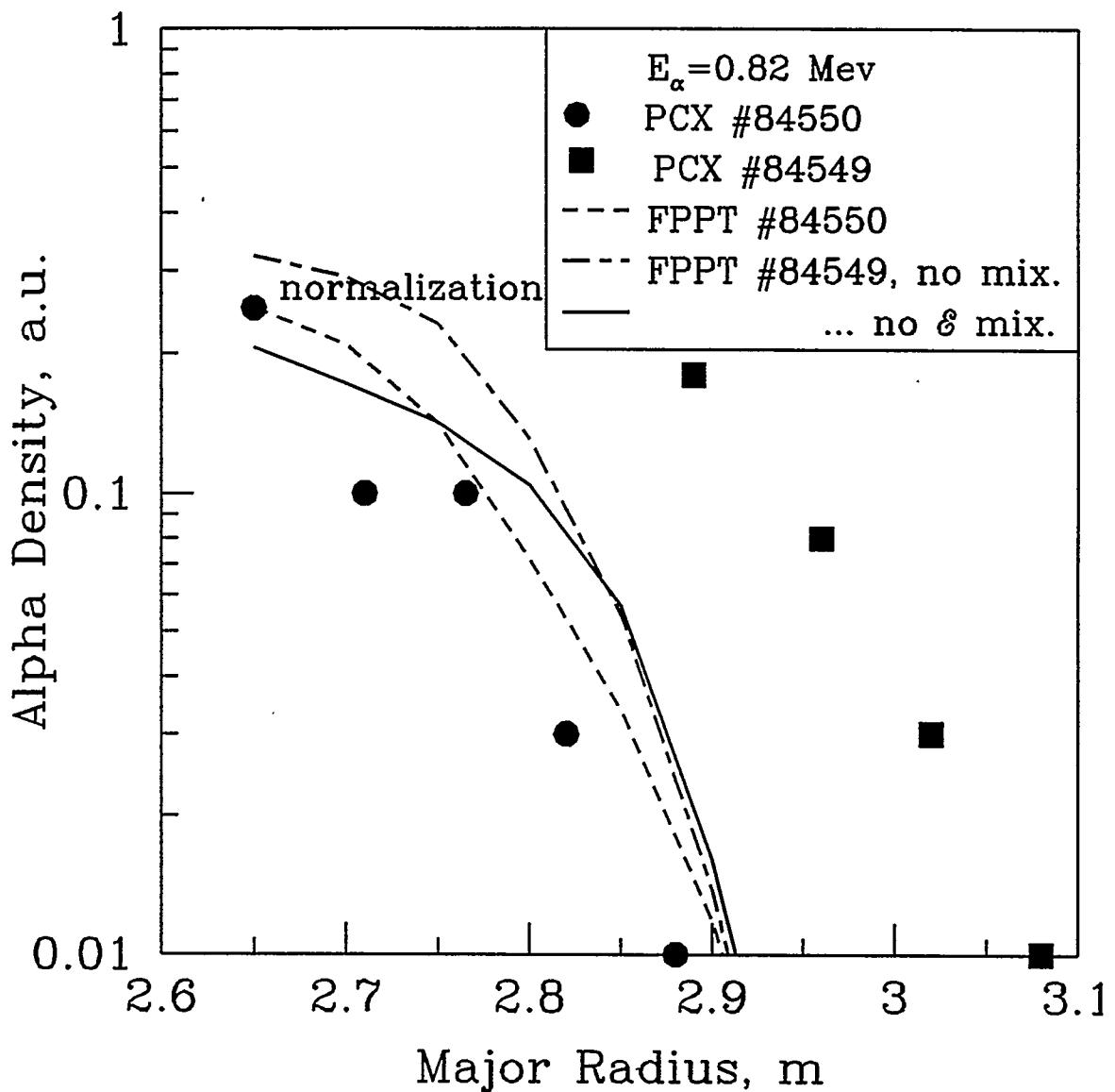
Figure 7: Alpha particle radial density profiles for  $E_\alpha = 0.82 \text{ MeV}$  from PCX data for a sawtooth free discharge # 84550 and a sawtooth discharge # 84549. Shown also are the results of FPPT modeling.
