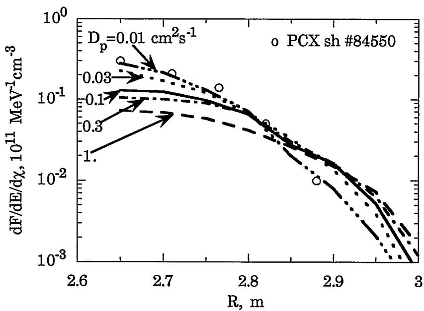
Figure 6: Simulation of  $\alpha$ -particle distribution function profiles for different diffusion coefficients of the banana tip  $p$  diffusion. PCX measured data are also shown.
