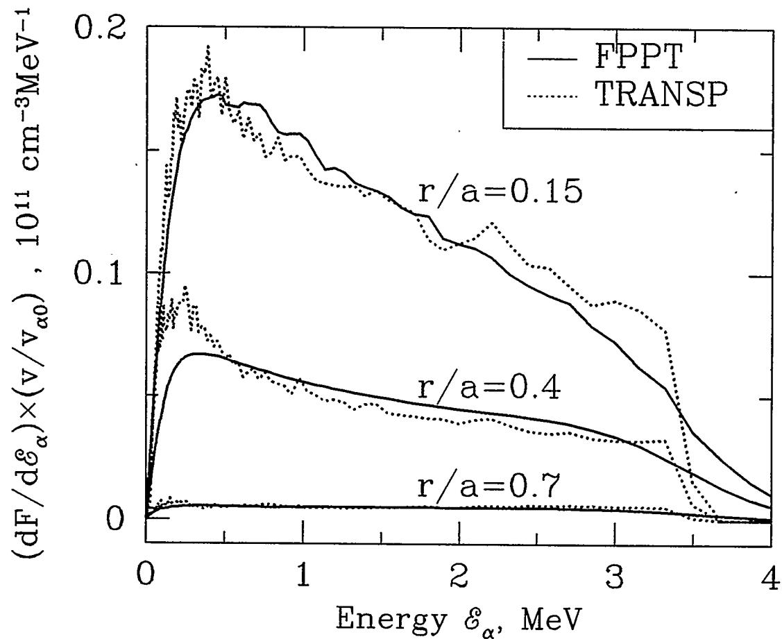
Figure 2: Comparison of FPPT and TRANSP Monte-Carlo calculations of  $\alpha$ -particle distribution functions versus energy. Spectra are averaged over the pitch angle and taken at different plasma minor radius in the equatorial plane at the low magnetic field side. The results are for TFTR shot #86644 at 4.15 sec, i.e. 0.15 sec after NBI.
