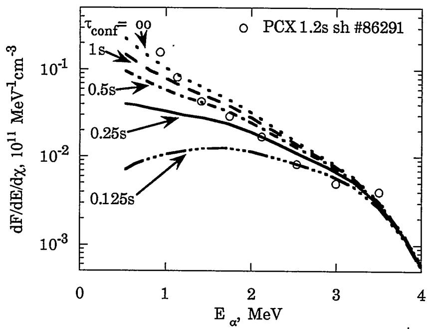
Figure 5: Comparison of PCX measurements with FPPT calculated spectra with different confinement times.
