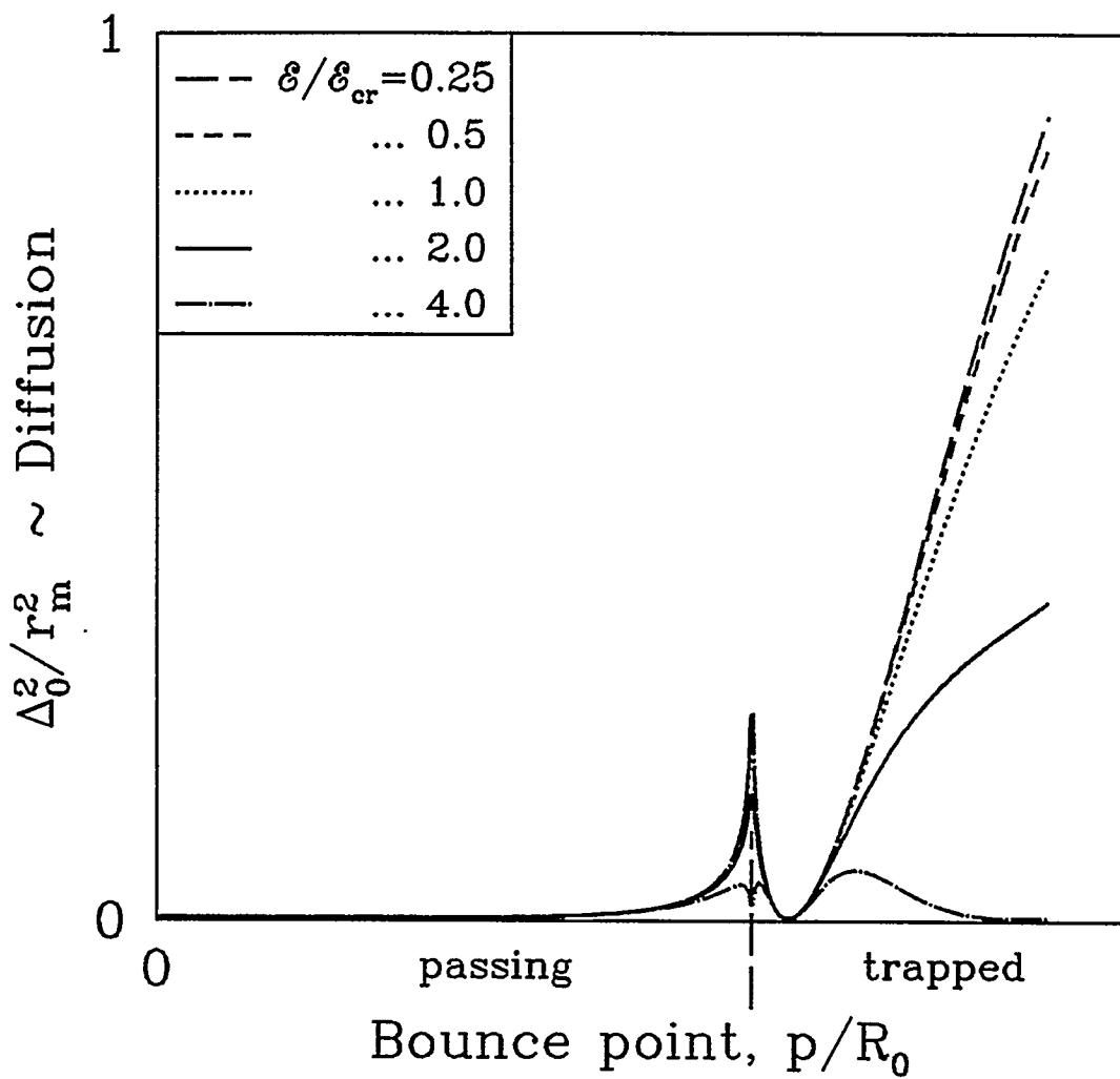
Figure 1: Fast particle bounce point displacement  $\Delta_0^2/r_m^2$  (see Eq.(21)) versus the position of the bounce point  $p/R_0$  at  $\epsilon = .2$ ,  $\mathcal{E}/\mathcal{E}_{cr} = 1/4, 1/2, 1, 2, 4$ , respectively.
