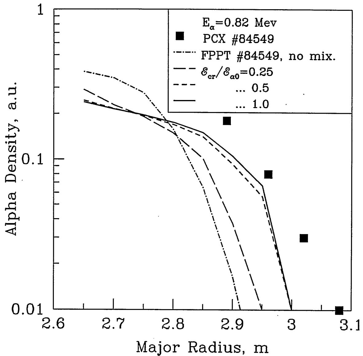
Figure 9: Alpha particle radial density profile for  $E_\alpha = 0.82 \text{ MeV}$  from PCX data for the discharge with a sawtooth #84549. Shown also are the results of FPPT modeling of trapped particle profiles for different critical energies.
