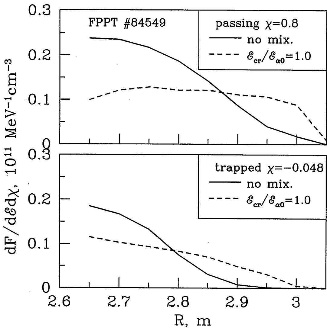
Figure 10: Passing (midplane pitch angle  $\chi_{mid} = 0.8$ ) and trapped ( $\chi_{mid} = -0.048$ )  $\alpha$ -particle profiles for  $\mathcal{E}_\alpha = 0.82$  MeV from FPPT calculations for the discharge #84549 with a sawtooth.
