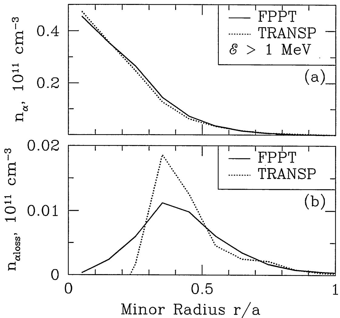
Figure 3: FPPT and TRANSP calculated energetic ( $\mathcal{E}_\alpha > 1$  MeV)  $\alpha$ -particle profiles of the (a) density and (b) stochastic loss due to the magnetic field ripples for the same shot as in the Fig. 2.
