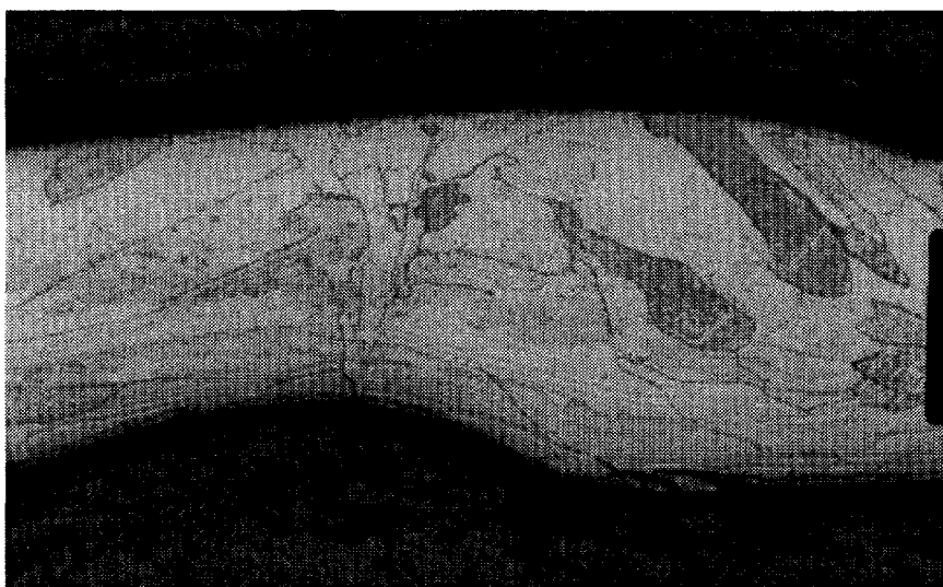
Figure 22. Bulge in weld overlap area, etched, at 50 \times magnification. (NMT-9 Neg 945-16)
