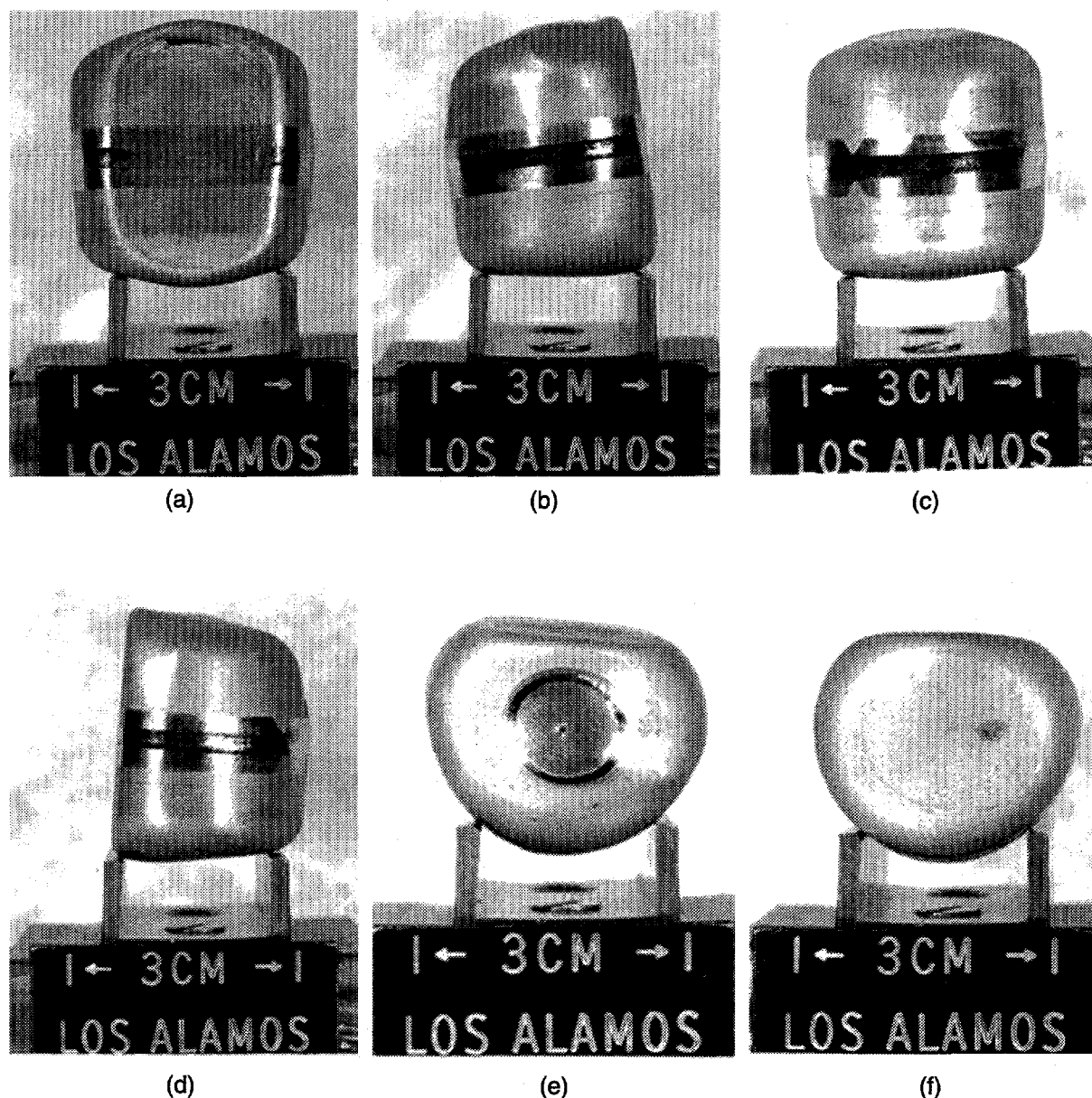
Figure 12. Capsule SC0017 was breached by a transverse and an axial crack on the impact face. (a) impact face, (b) profile, (c) trailing face, (d) opposite profile, (e) vent end, (f) blind end. (NMT-9 Negs 931-22, 931-25, 931-24, 931-23, 931-26, 931-28)
