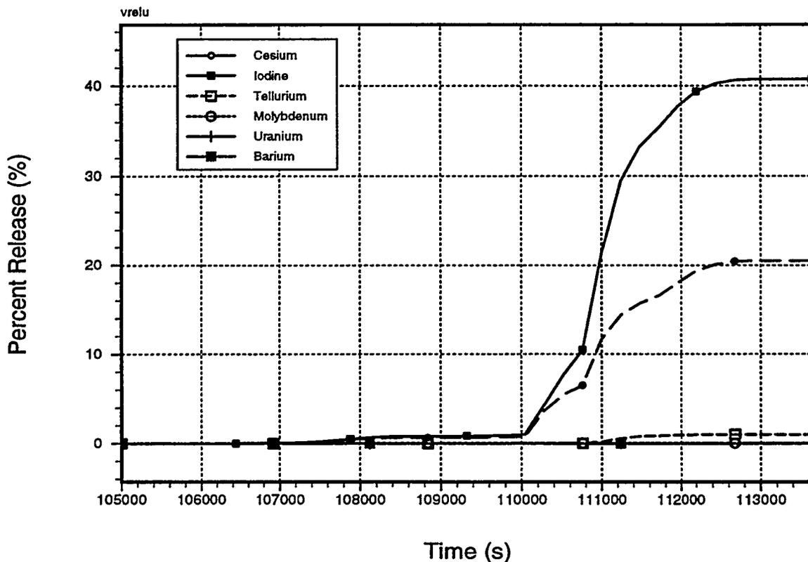
Figure 4. Release histories, as a percent of fuel inventory, for cesium, iodine, tellurium, molybdenum, uranium, and barium.
