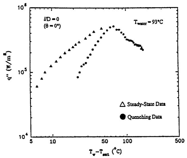
Figure 9. Comparison of the Steady-State and Transient Quenching Data for Water at 93°C.
