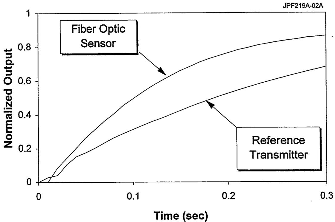
Figure 5.7 Results of an Increasing Pressure Ramp Showing the Faster Dynamic Response of the Fiber Optic Pressure Sensor versus the Reference Sensor
