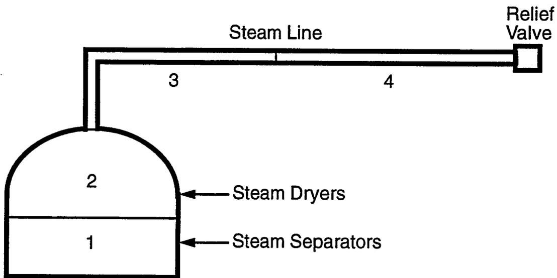
Figure 3. Schematic of the VICTORIA nodalization of the steam generator secondary and steam line.
