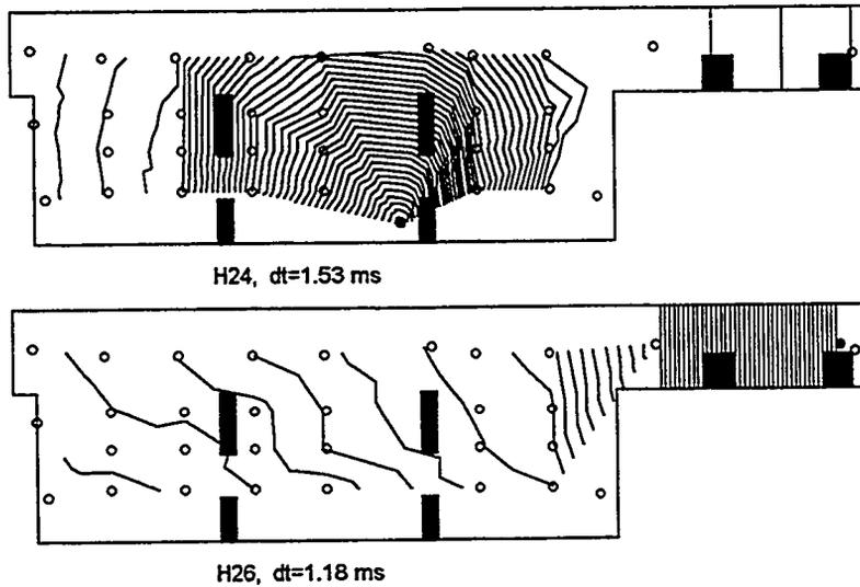
Figure 3. Flame positions as a function of time for tests 24 (upper) and 26 (lower).
