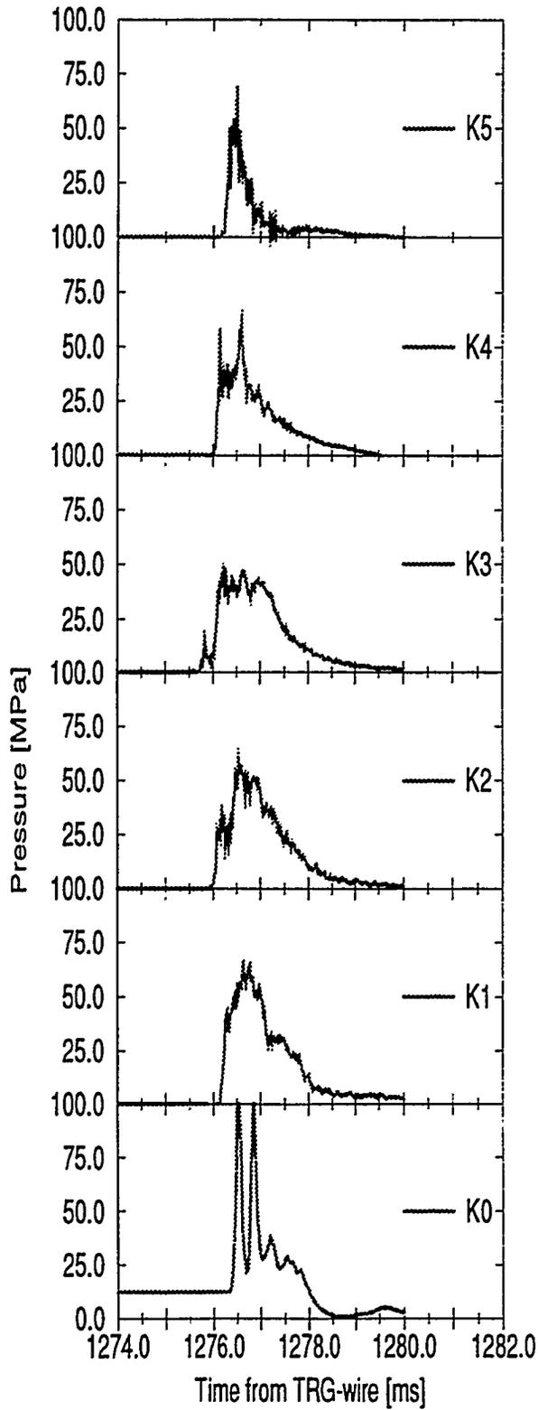
Fig. 2.3 Dynamic Pressures in the Test Section, KROTOS 38
