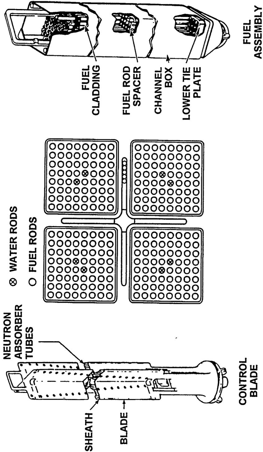
Figure 1. Sketch of typical BWR control blade and fuel assembly.
