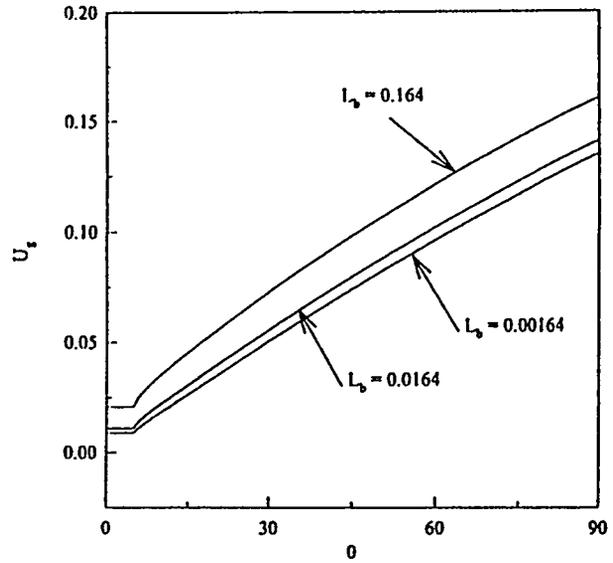
Figure 13. Predicted Variation of the Dimensionless Local Vapor Velocity.
