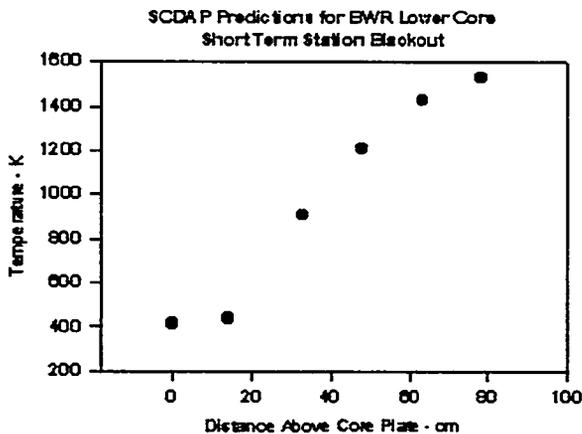
**Figure 7: Target conditions for axial thermal gradient in the lower BWR core for Dry-Core (Station Blackout with depressurization).**
