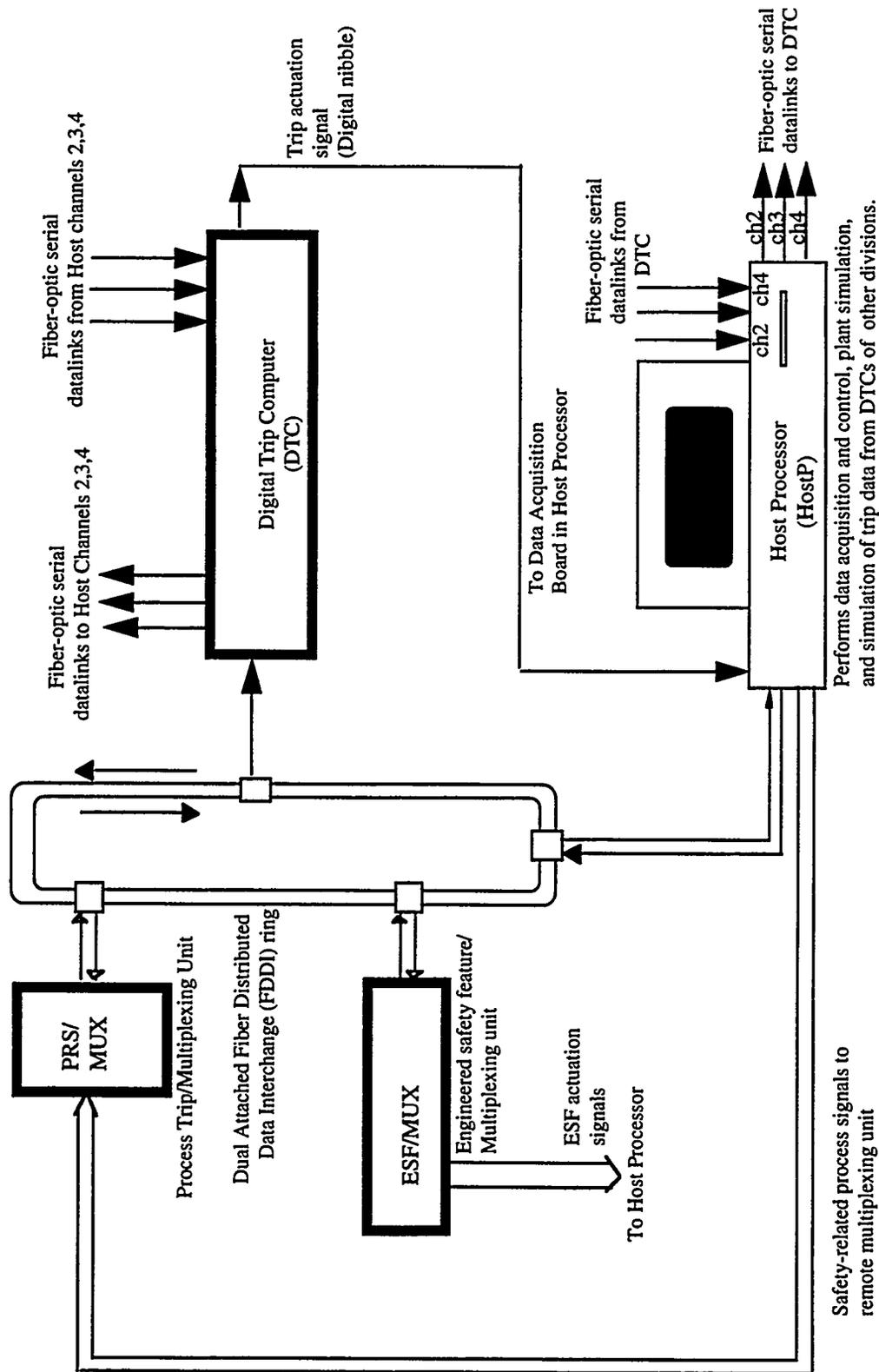
Figure 2. Block diagram of the experimental digital safety channel.
