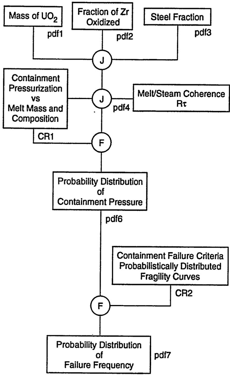
**Figure 2.** The probabilistic framework for containment failure under direct containment heating scenarios. The (J) and (F) are the “joint” and “function” operations, respectively, as described in the text.
