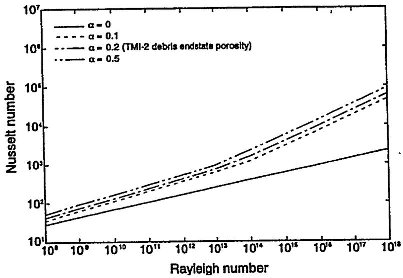
Figure 13. Comparison of the molten pool natural circulation heat transfer for different vapor void fractions in the melt.
