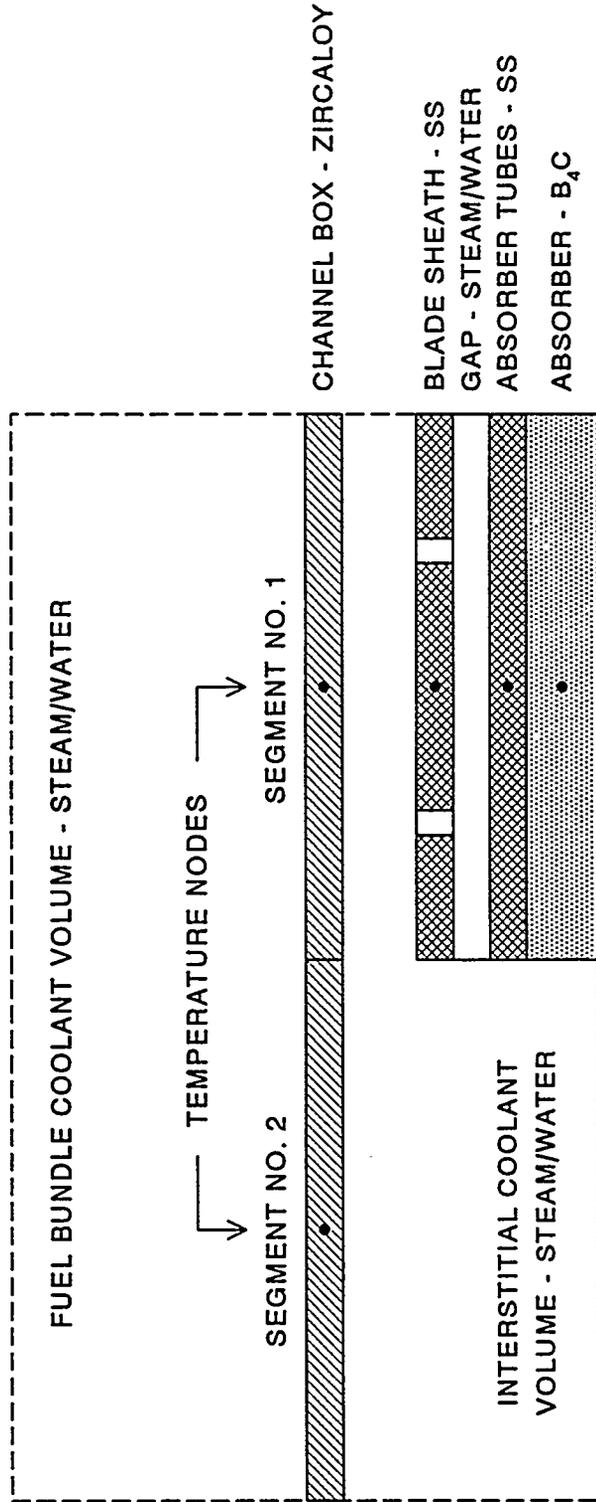
**Figure 2. BWR control blade/channel box model with equivalent slab geometry and five temperature nodes at each axial elevation.**
