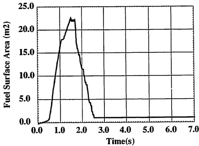
FIG. 1.9 - Variation of Fuel Surface Area for TEXAS-IV Calculation L-19
