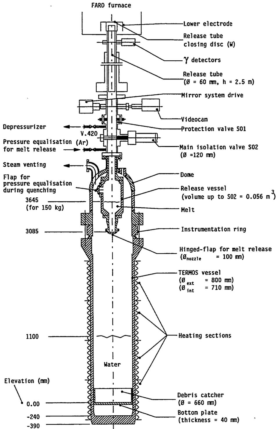
Fig. 1.1 - Experimental arrangement for FARO Test L-19
