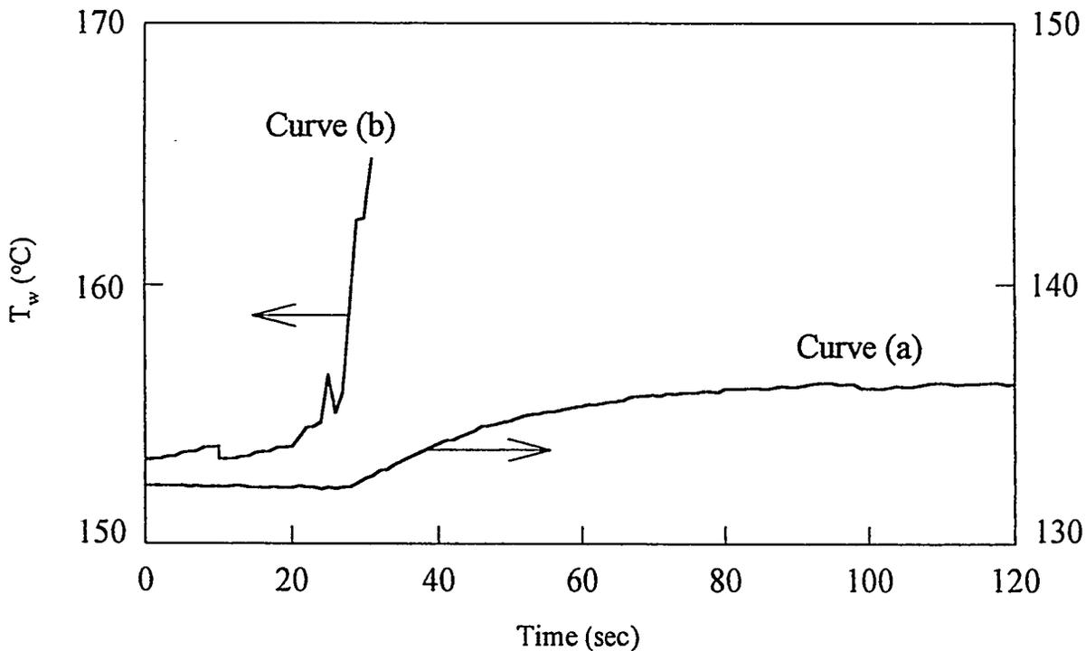
Figure 4. Typical Time Responses of the Local Wall Temperature Following a Step Increase in the Wall Heat Flux.
