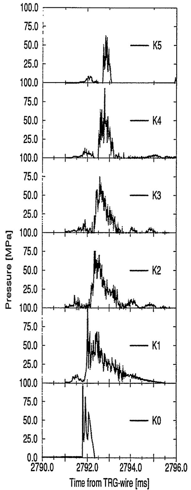
Fig. 2.6 Dynamic Pressures in the Test Section, KROTOS 43
