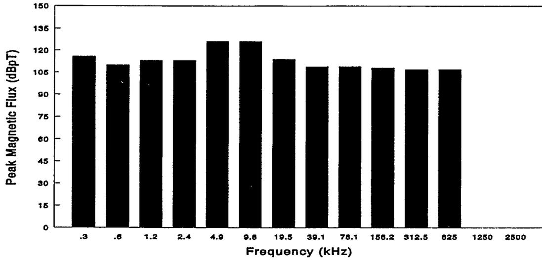
**Fig. 2 Highest observed magnetic flux**
