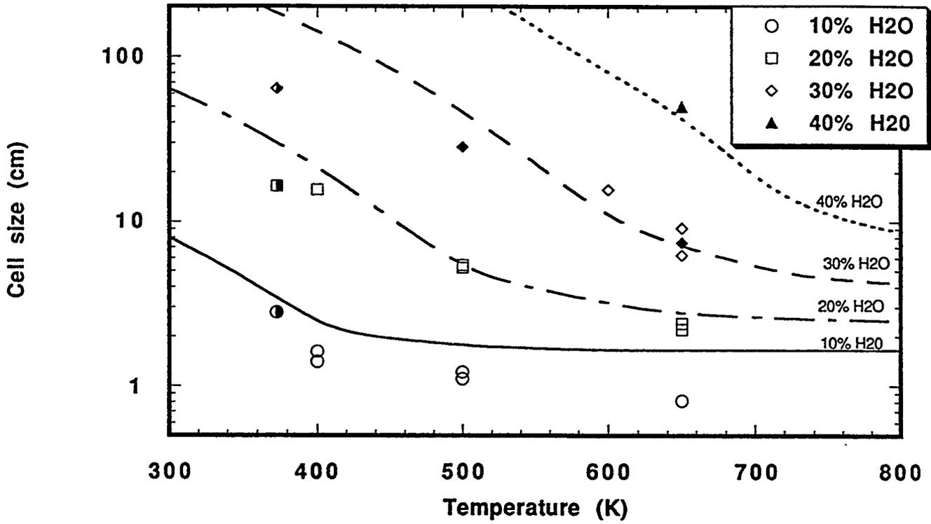
Figure 6: Detonation cell size as a function of temperature for stoichiometric hydrogen-air and steam mixtures at 0.1 MPa
