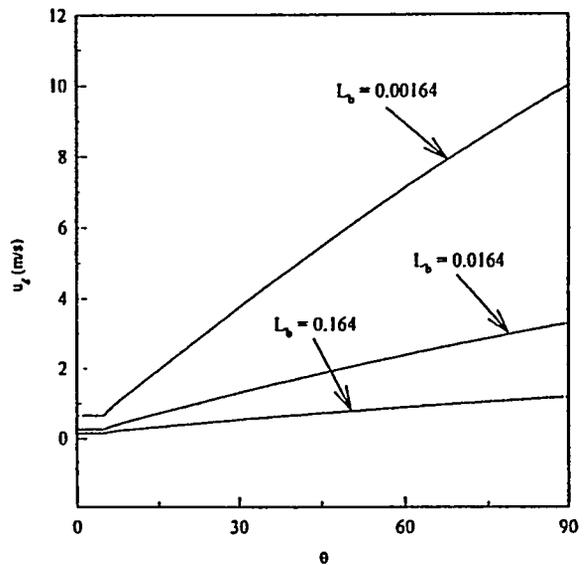
Figure 14. Predicted Variation of the Actual Local Vapor Velocity.
