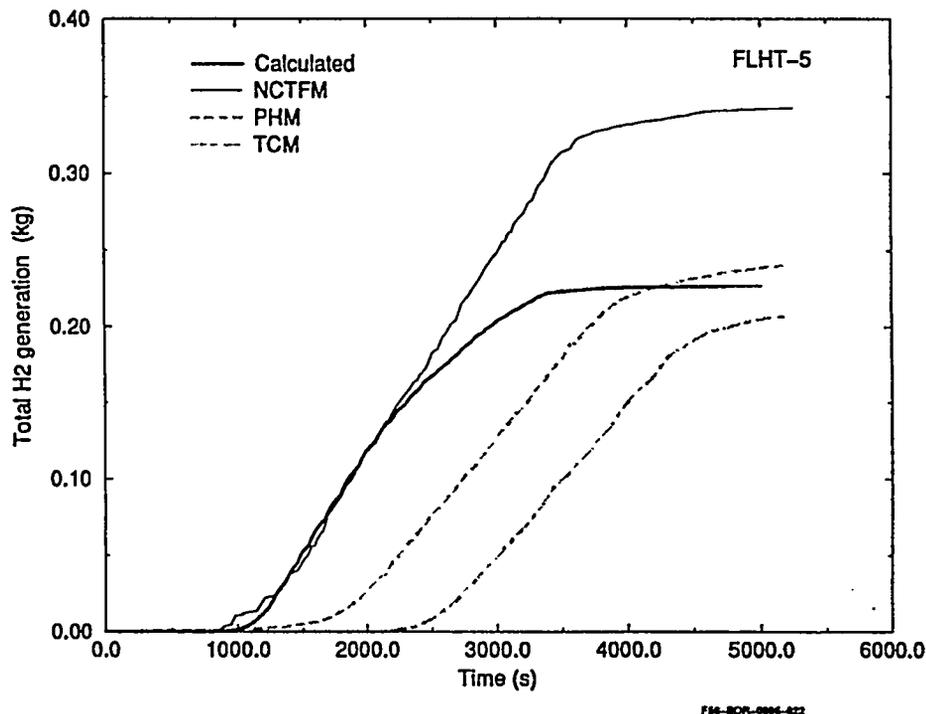
Figure 6 - Comparison of calculated and measured integrated hydrogen production for the FLHT-5 experiment.
