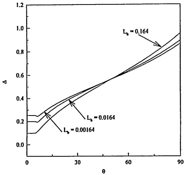
Figure 11. Predicted Variation of the Dimensionless Local Boundary Layer Thickness.
