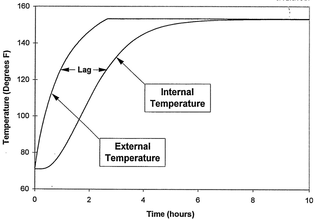
Figure 5.3 Temperature Lag Between the External and Internal Temperature Seen by the Fiber Optic Pressure Transducer
