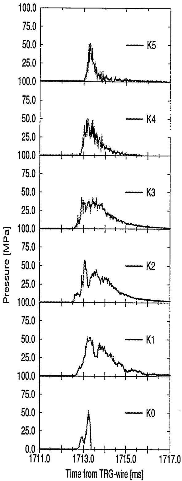
Fig. 2.5 Dynamic Pressures in the Test Section, KROTOS 42
