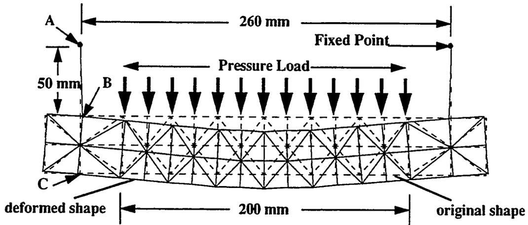
FIG. 2.10 - Pressure Loading of the KROTOS Test Section Base Plate - KROTOS 43
