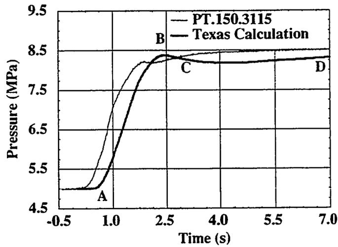
FIG. 1.8 - Comparison between TEXAS-IV and Experiment - FARO Test L-19
