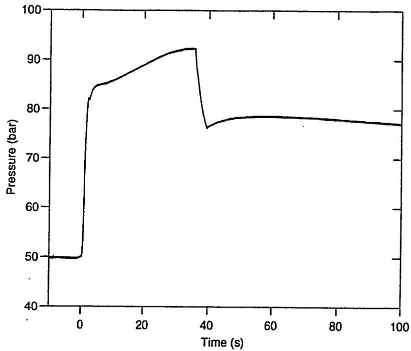
Fig 1.2 - FARO L-19 vessel pressure up to 100 s
