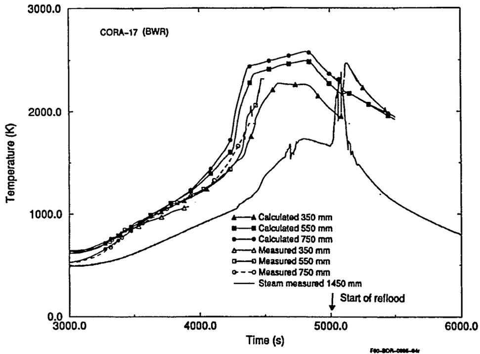
Figure 2 - Calculated and measured bundle temperatures for the CORA-17 BWR experiment.
