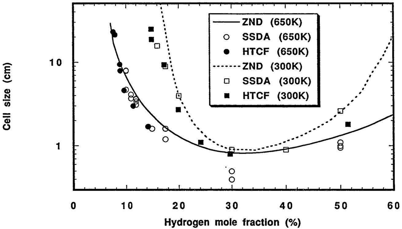
Figure 5: Comparison of detonation cell size for hydrogen-air mixtures at 300K and 650K at 0.1 MPa
