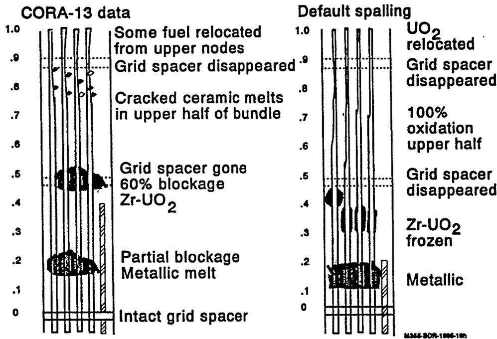
Figure 7 - Comparison of calculated and observed bundle end states for the CORA-13 PWR experiment with reflow.
