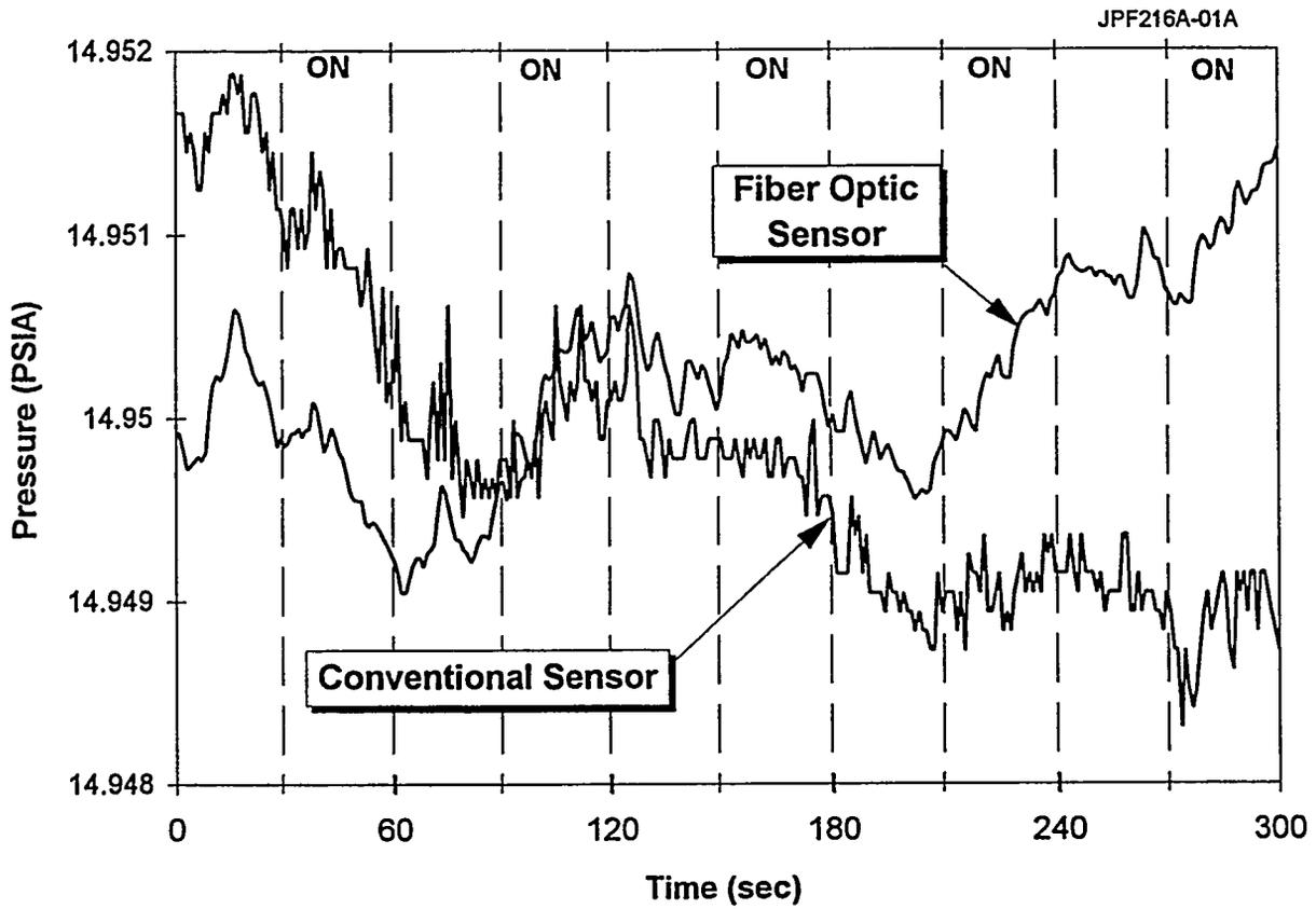
Figure 5.5 Results of One Series of Vibration Tests Showing no Visible Effect on the Fiber Optic Sensor Output as the Vibration Beam Motor was Cycled On and Off
