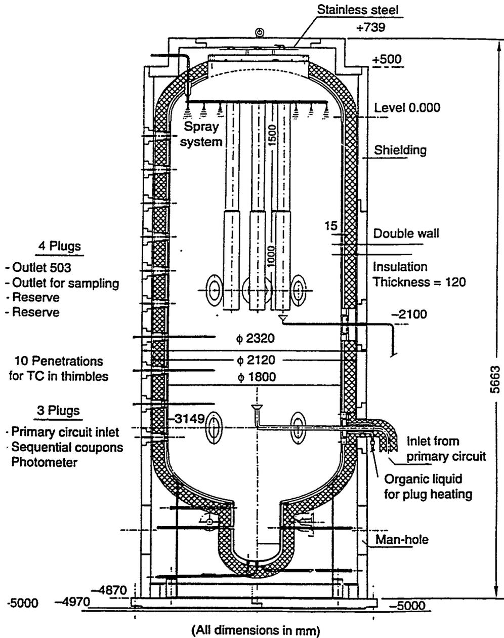
Figure 4 - Phebus FP REPF 502 containment vessel
