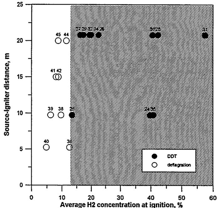
Figure 7. Range of parameters for DDT in dynamic injection/ignition experiments.
