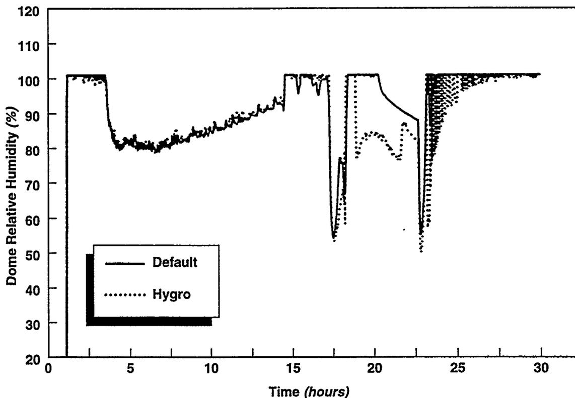
Figure 1. Relative humidity in the dome as predicted by MELCOR.
