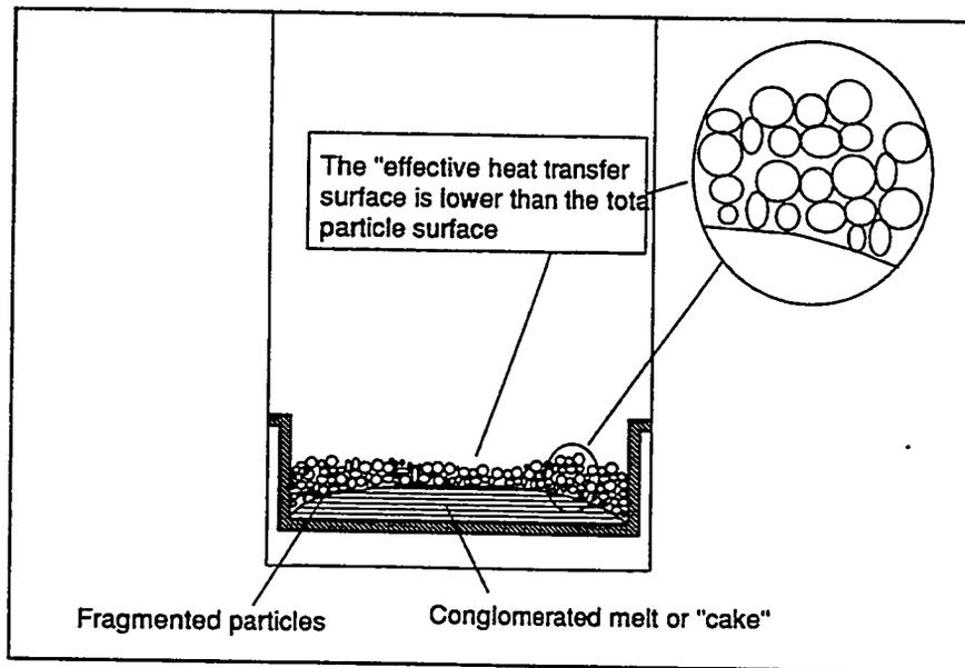
Fig. 1.12 - Representation of the debris bed configuration
