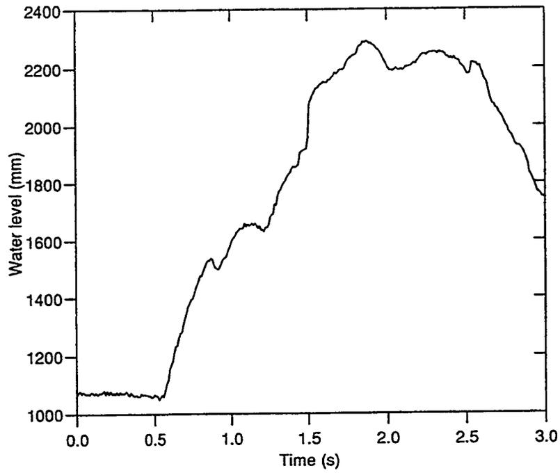
Fig. 1.4 - Water level in FARO Test L-19
