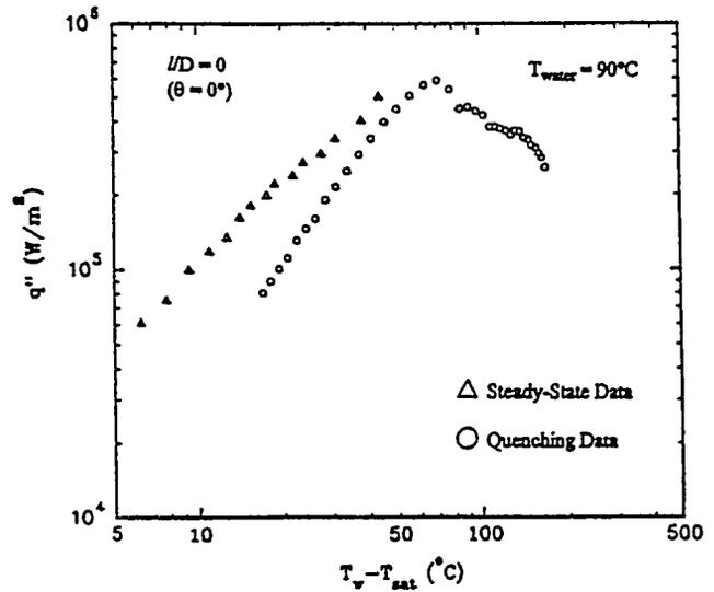
Figure 10. Comparison of the Steady-State and Transient Quenching Data for Water at 90°C.
