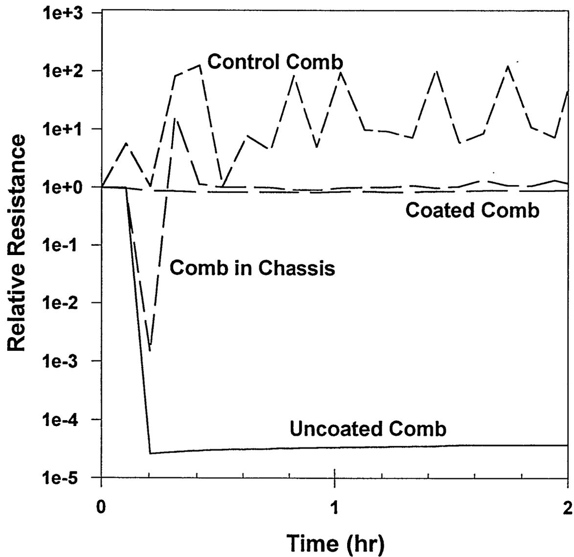
Figure 5. Circuit Bridging Test on 160 V Comb pattern.
