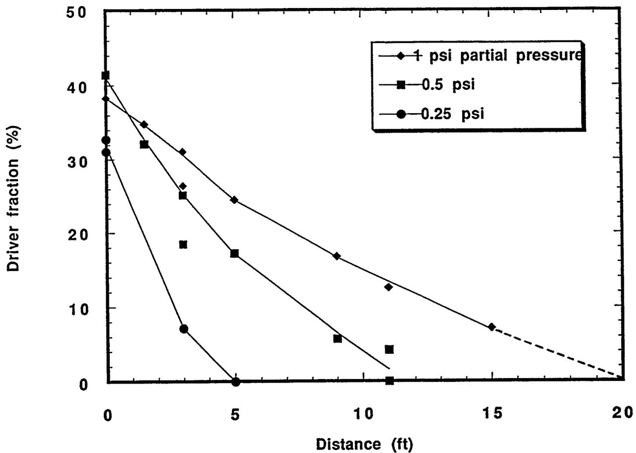
Figure 2: Experimentally measured driver-gas (C<sub>2</sub>H<sub>2</sub> + O<sub>2</sub>) axial distribution in the test vessel at 1 second after driver-gas injection
