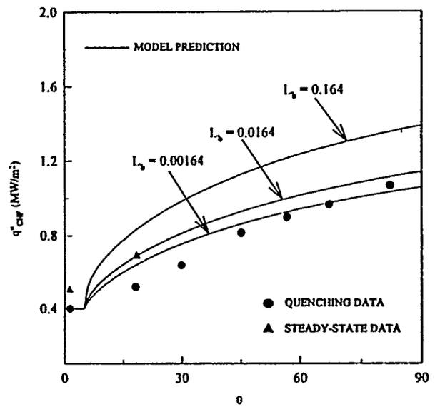
Figure 18. Predicted Variation of the Local Critical Heat Flux: Comparison with Experiments
