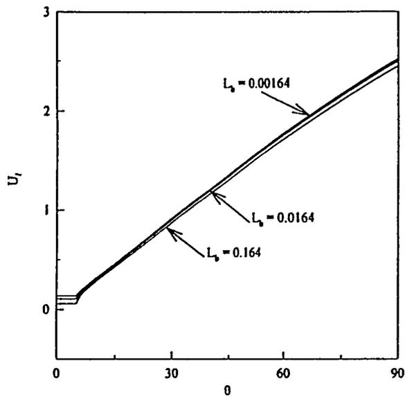
Figure 15. Predicted Variation of the Dimensionless Local Liquid Velocity.
