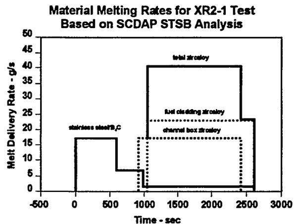
**Figure 8: Target conditions for flow rate of molten metallic materials from upper core into lower core.**
