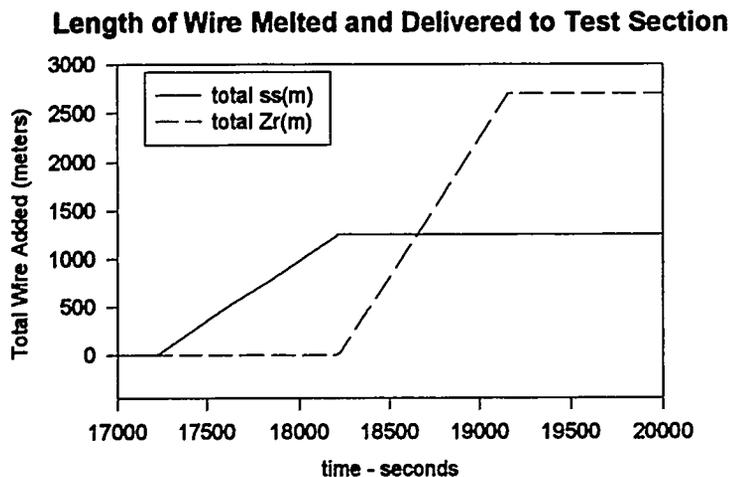
Figure 9. Wire feed history for the XR2-1 test.
