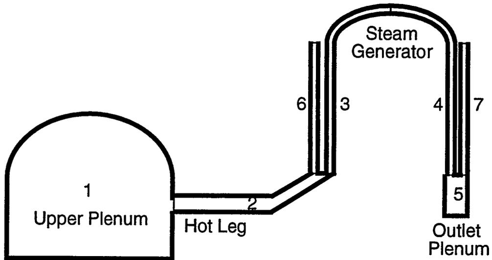
Figure 2. Schematic of the VICTORIA nodalization of the upper plenum and primary circuit.
