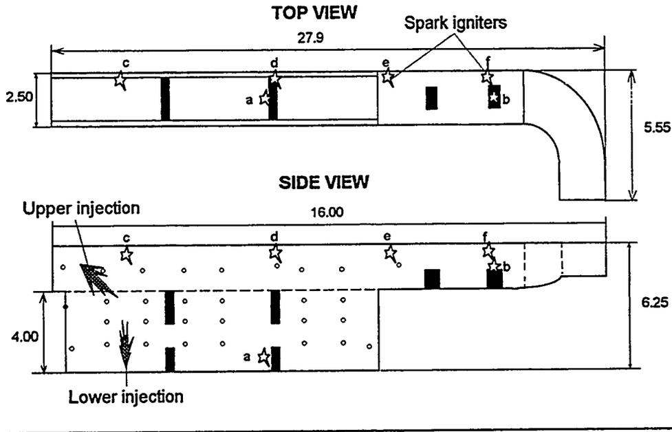
Figure 2. Scheme of RUT facility
