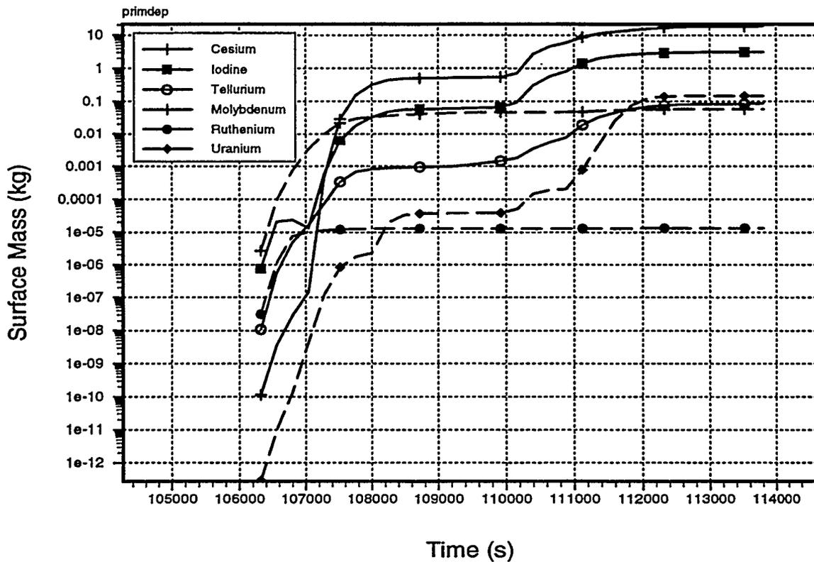
Figure 5. VICTORIA-predicted retention histories in the reactor coolant system.
