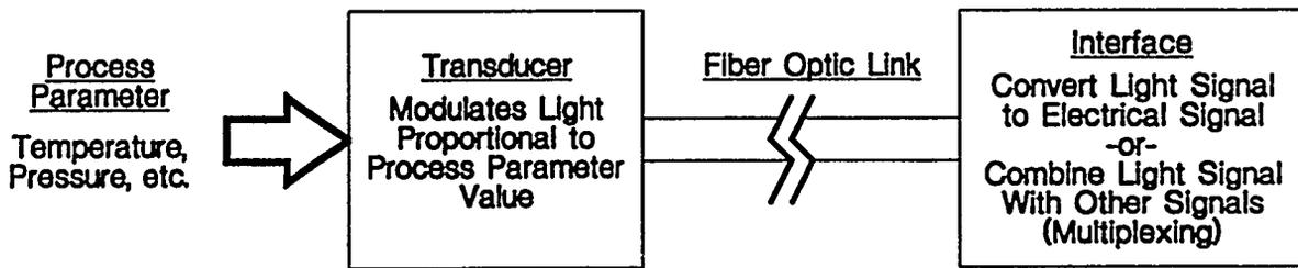
Figure 2.1 Illustration of the Basic Components of a Fiber Optic Sensing System
