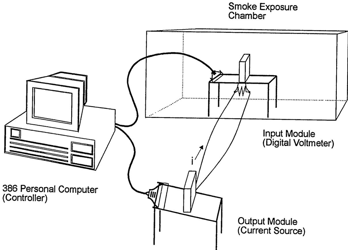
Figure 1. Multiplexer Test Setup.
