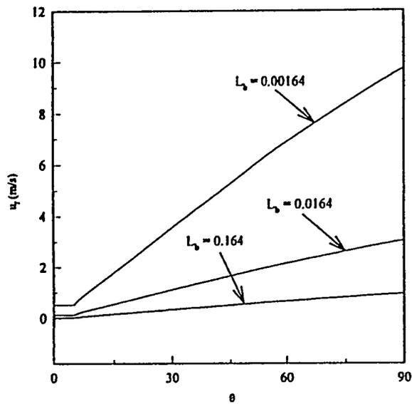
Figure 16. Predicted Variation of the Actual Local Liquid Velocity.
