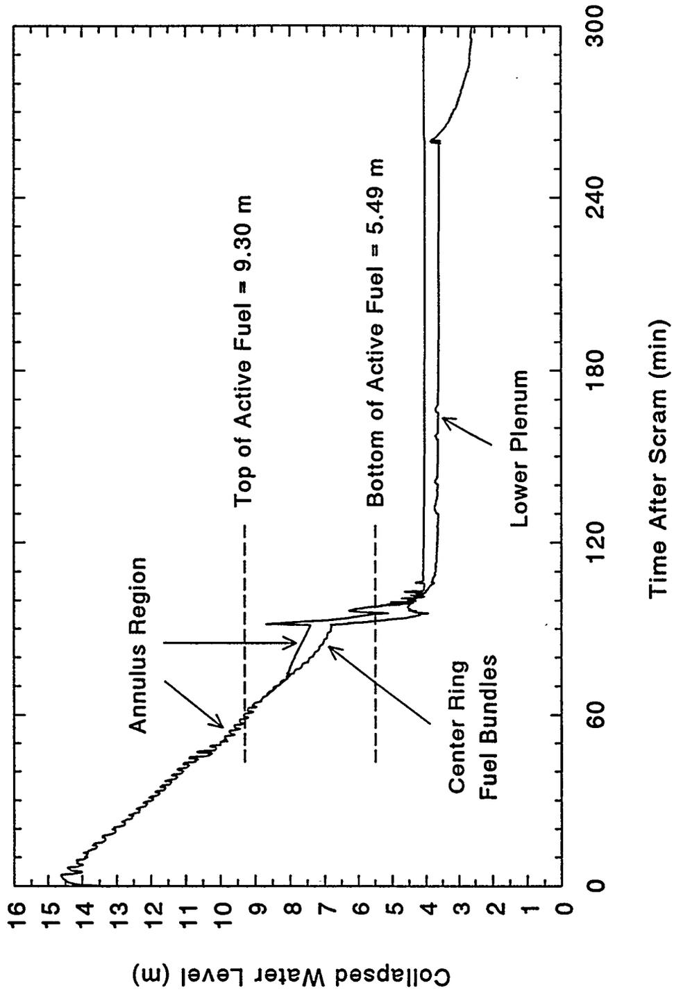
Figure 8. Calculated vessel water levels for Browns Ferry STSB accident.
