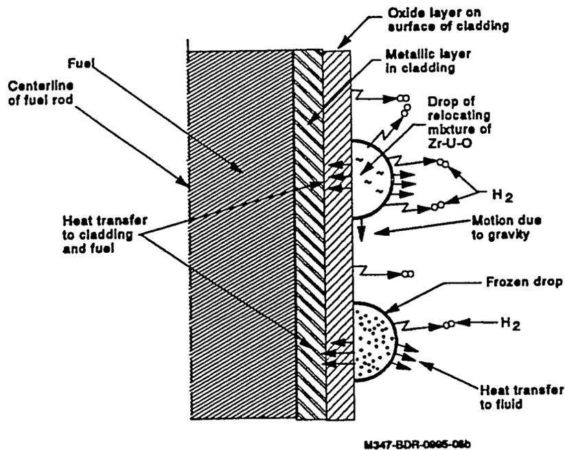
Figure 1 - MOD3.1e U-Zr-O droplet oxidation model.
