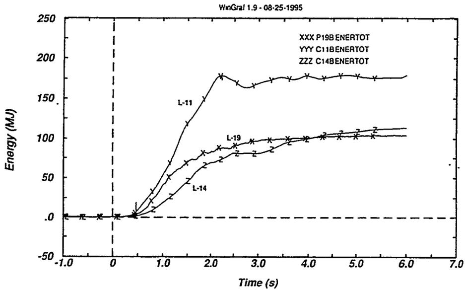
Fig. 1.6 - Comparison of energy released to the water in tests L-11, L-14 and L-19
