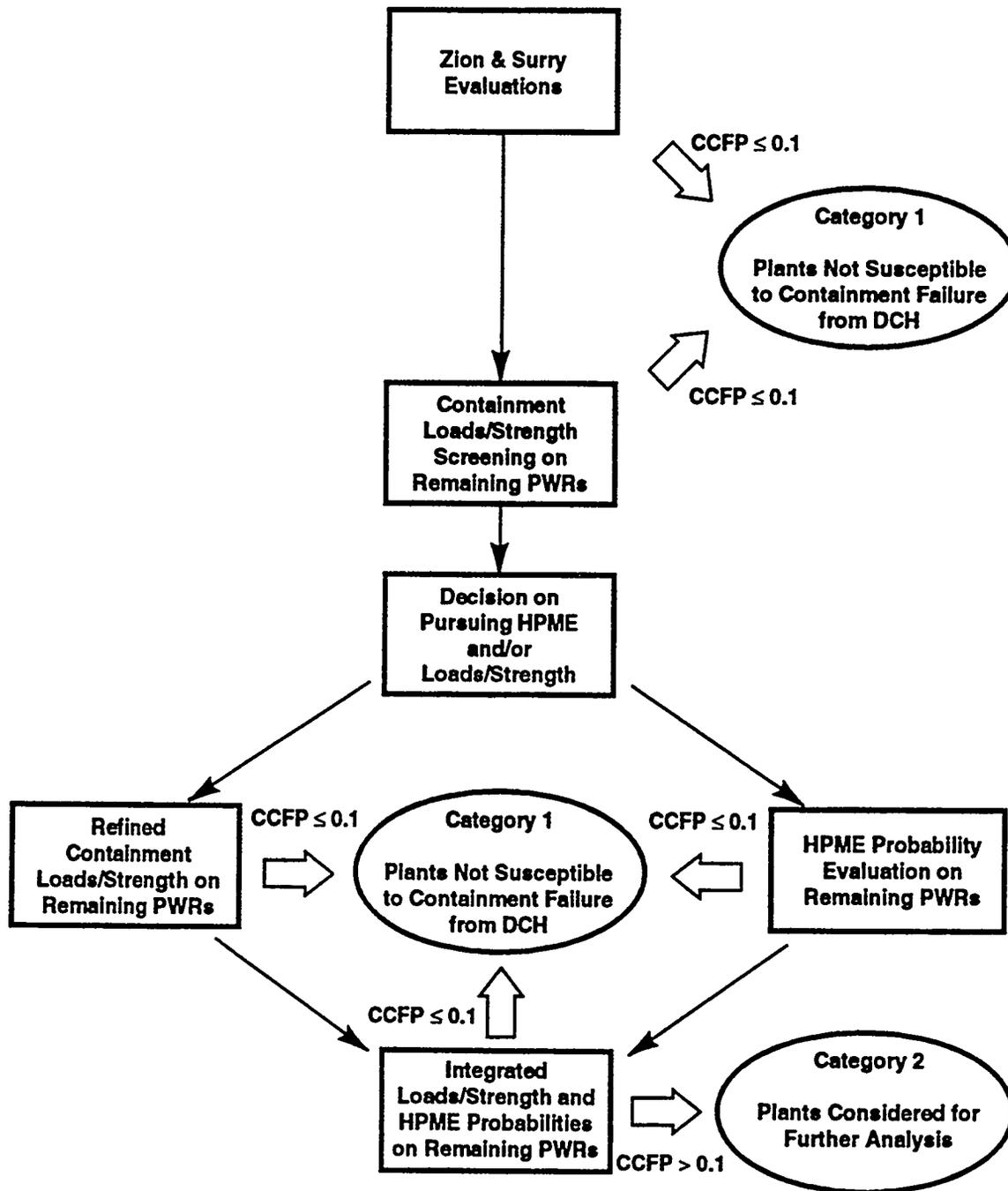
Figure 1. Methodology for resolution of the DCH issue for all PWRs.
