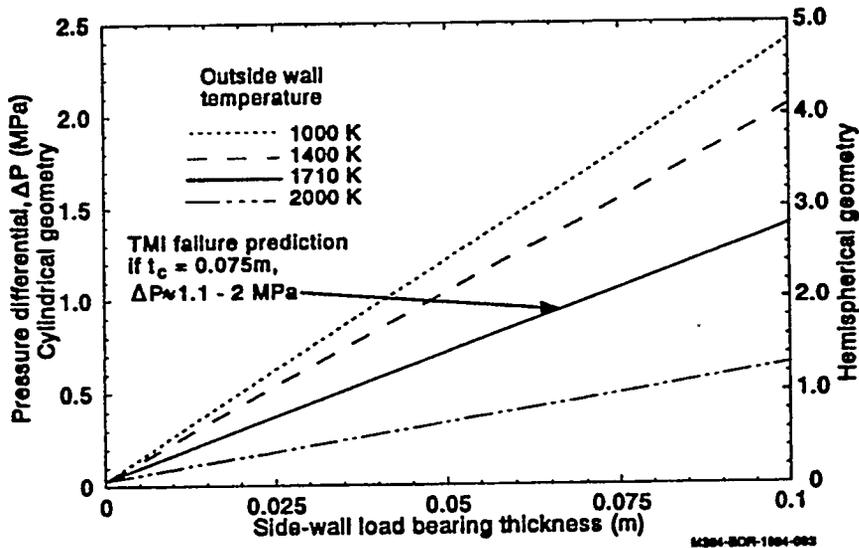
Figure 14. Side-wall failure map for a closed crucible with molten interior and linear through-wall temperature distribution.
