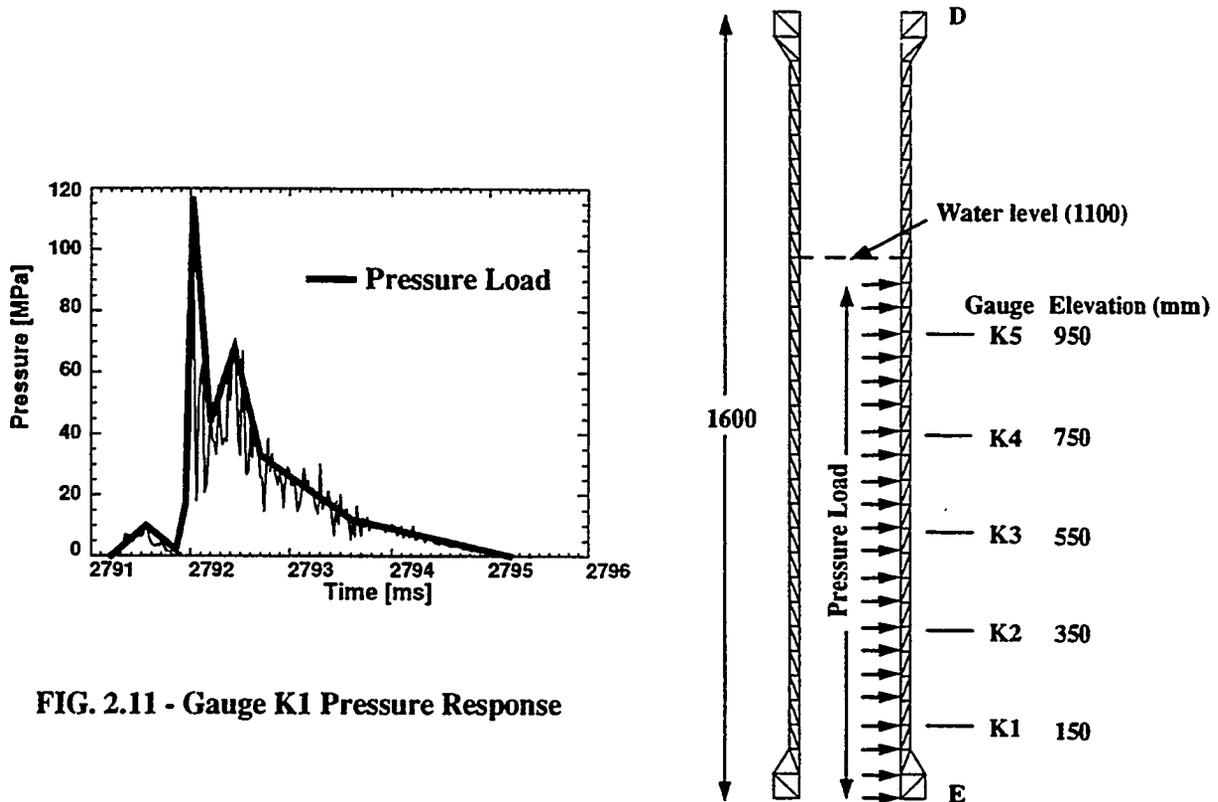
FIG. 2.11 - Gauge K1 Pressure Response
