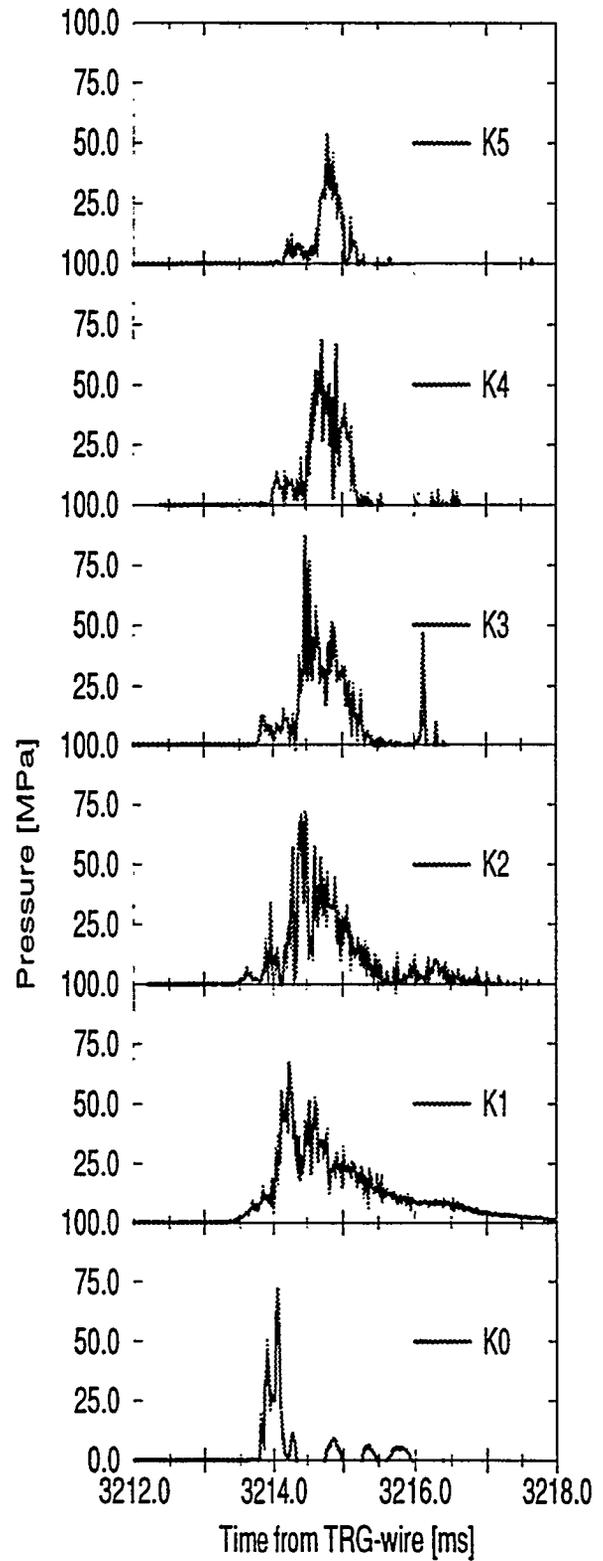
Fig. 2.4 Dynamic Pressures in the Test Section, KROTOS 40
