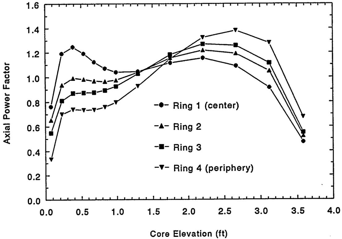
Figure 6. Browns Ferry power profiles for 13 axial nodes.
