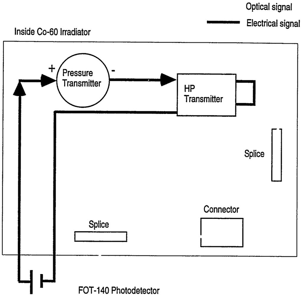
In the test channel shown in Figure 2, a conventional capacitive differential pressure sensor produces a current signal proportional to pressure. A constant amount of pressure is applied to the pressure sensor, which generates a constant current. This current drives the transmitter, which produces a light signal. The output light signal of the transmitter is routed through the components shown before detection.
