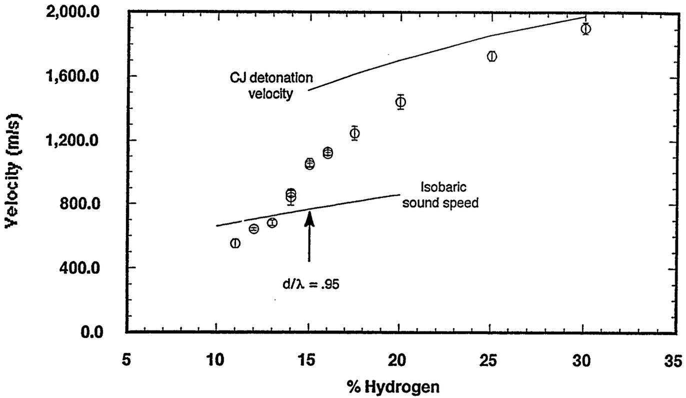
Figure 7: Measured flame velocity vs. gas composition for tests conducted at 300K
