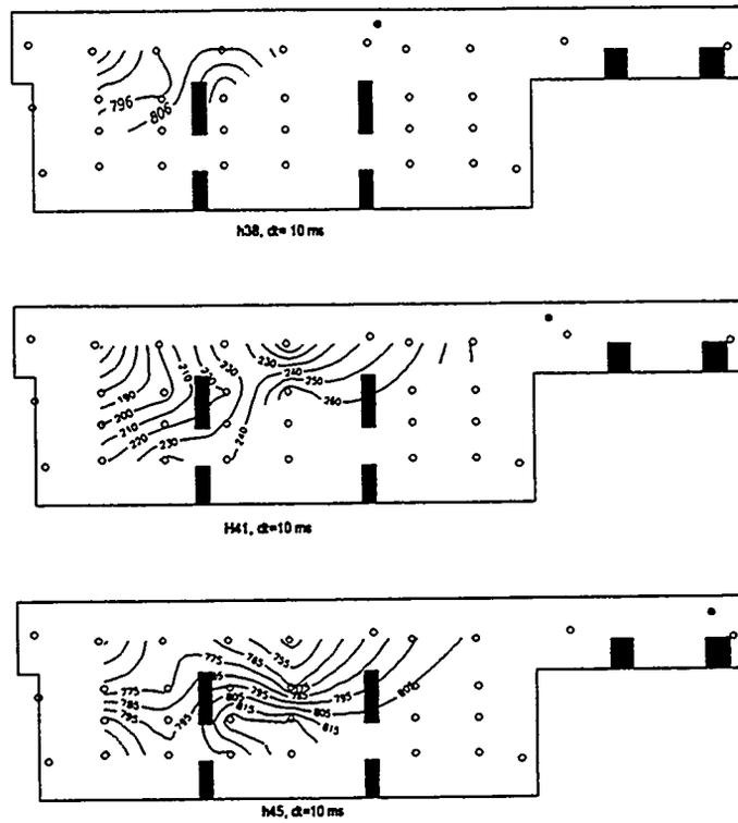
Figure 5. Flame shape as a function of time for tests 38, 41, and 45. dt is time step.
