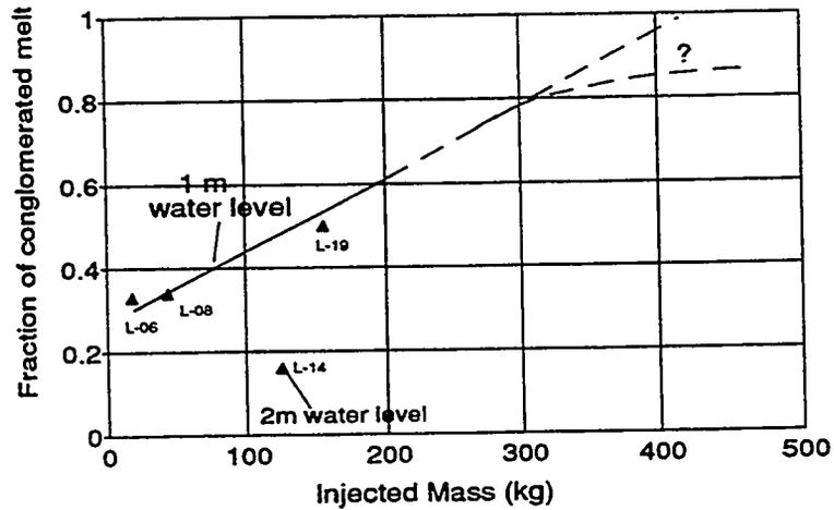
Fig. 1.15 - Fraction of conglomerate debris as a function of the melt quantities used in FARO and possible evolutions
