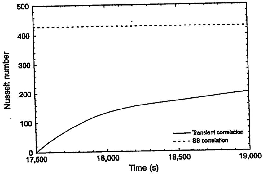
Figure 12. Comparison of steady-state and transient molten pool natural circulation heat transfer for a reactor scale pool.
