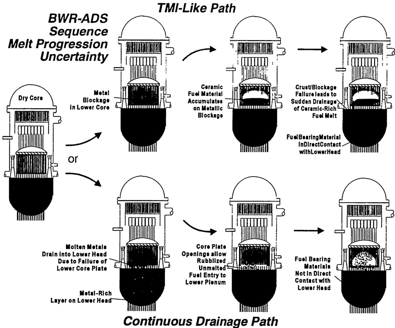
Figure 1. Illustration of the melt progression branchpoint uncertainty for "dry core" and "wet core" scenarios.
