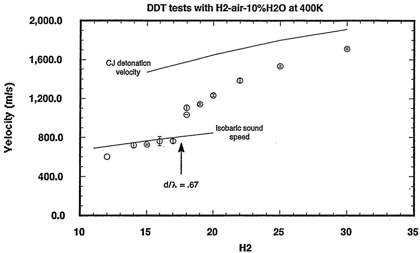
Figure 9: Measured flame velocity vs. gas composition for tests conducted at 400K and 10 percent steam
