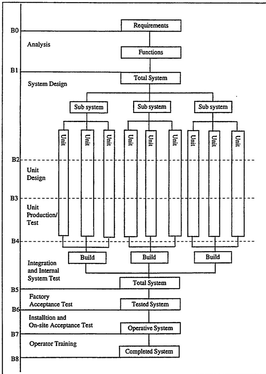
Figure 2. Configuration phases and baselines
