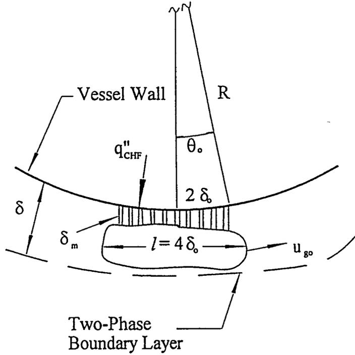
Figure 3. The Micro-Layer and the Vapor Slug at the Bottom Center of the Vessel.
