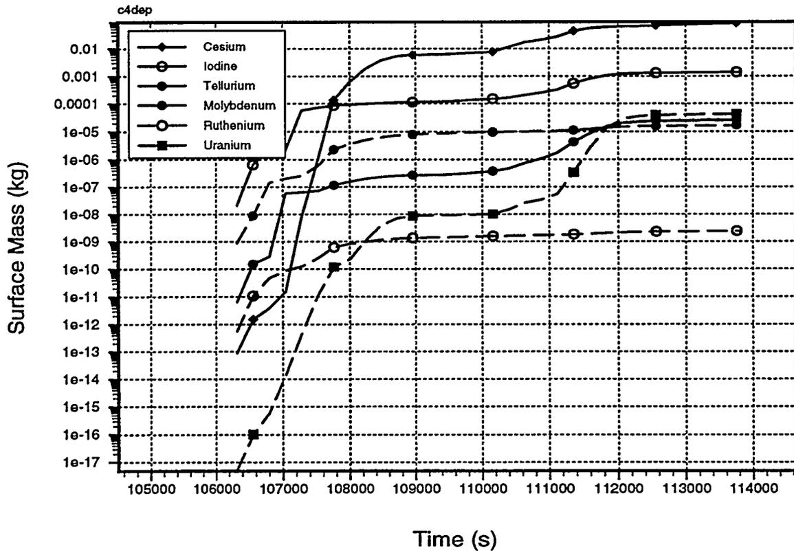
Figure 6. VICTORIA-predicted retention histories in the secondary circuit.
