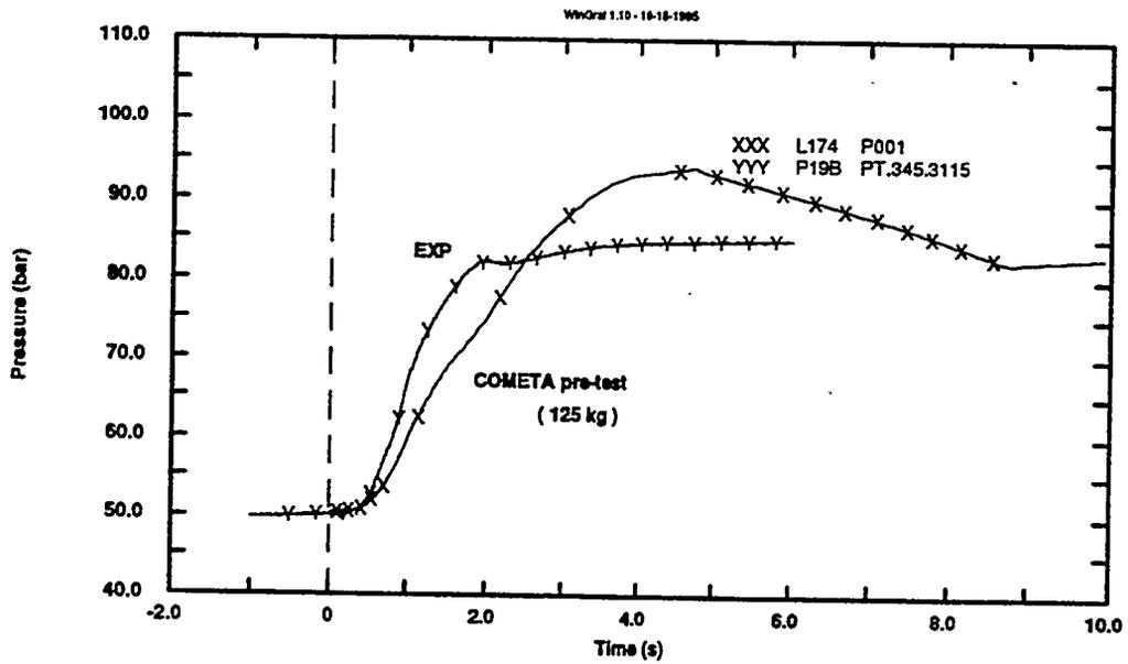
Fig. 1.11 - Pre Test prediction by COMETA code: Pressure
