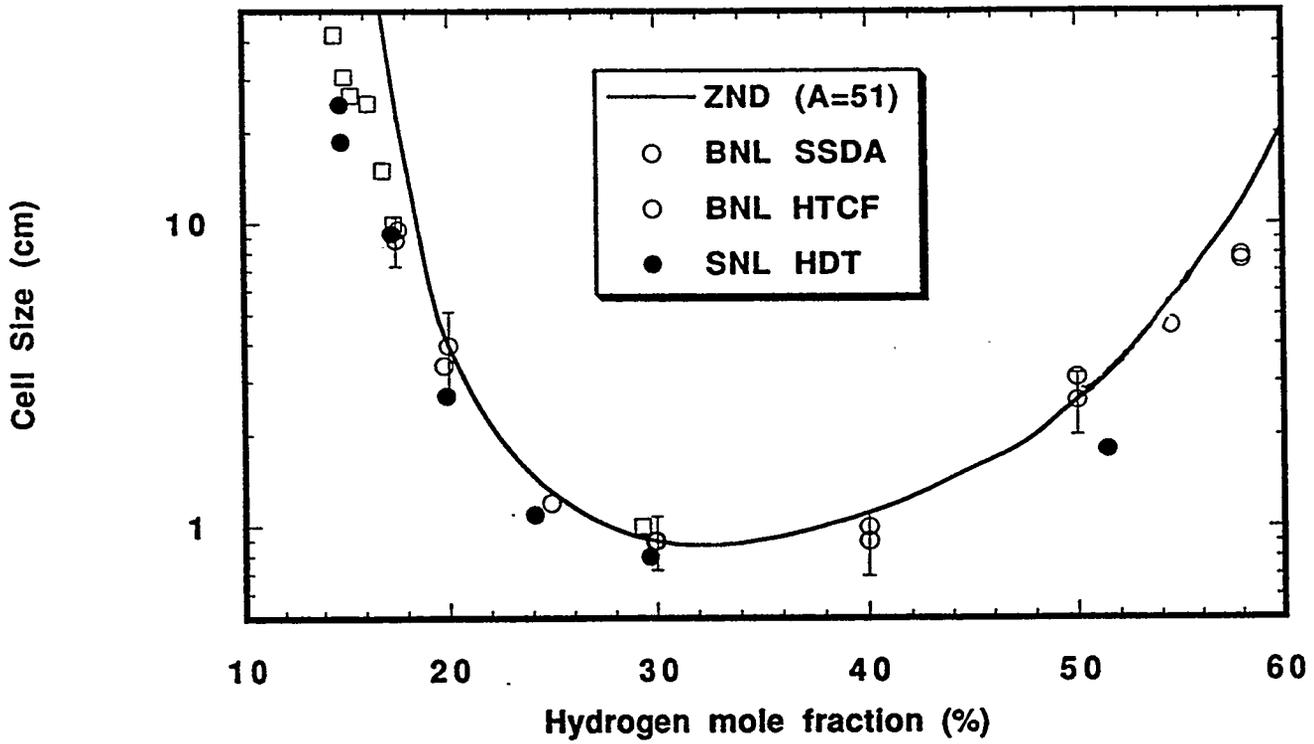
Figure 4: Detonation cell size for hydrogen-air mixtures at 300K and 0.1 MPa
