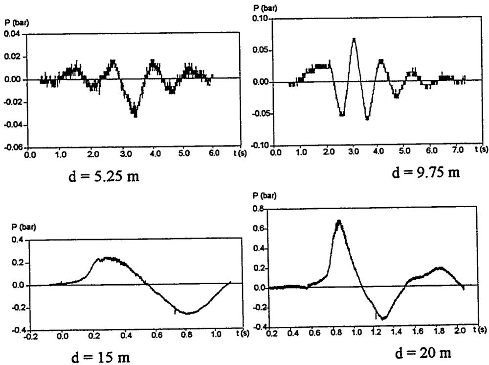
Figure 6. Pressure records for lower injection location (d - distance from igniter to injection point).
