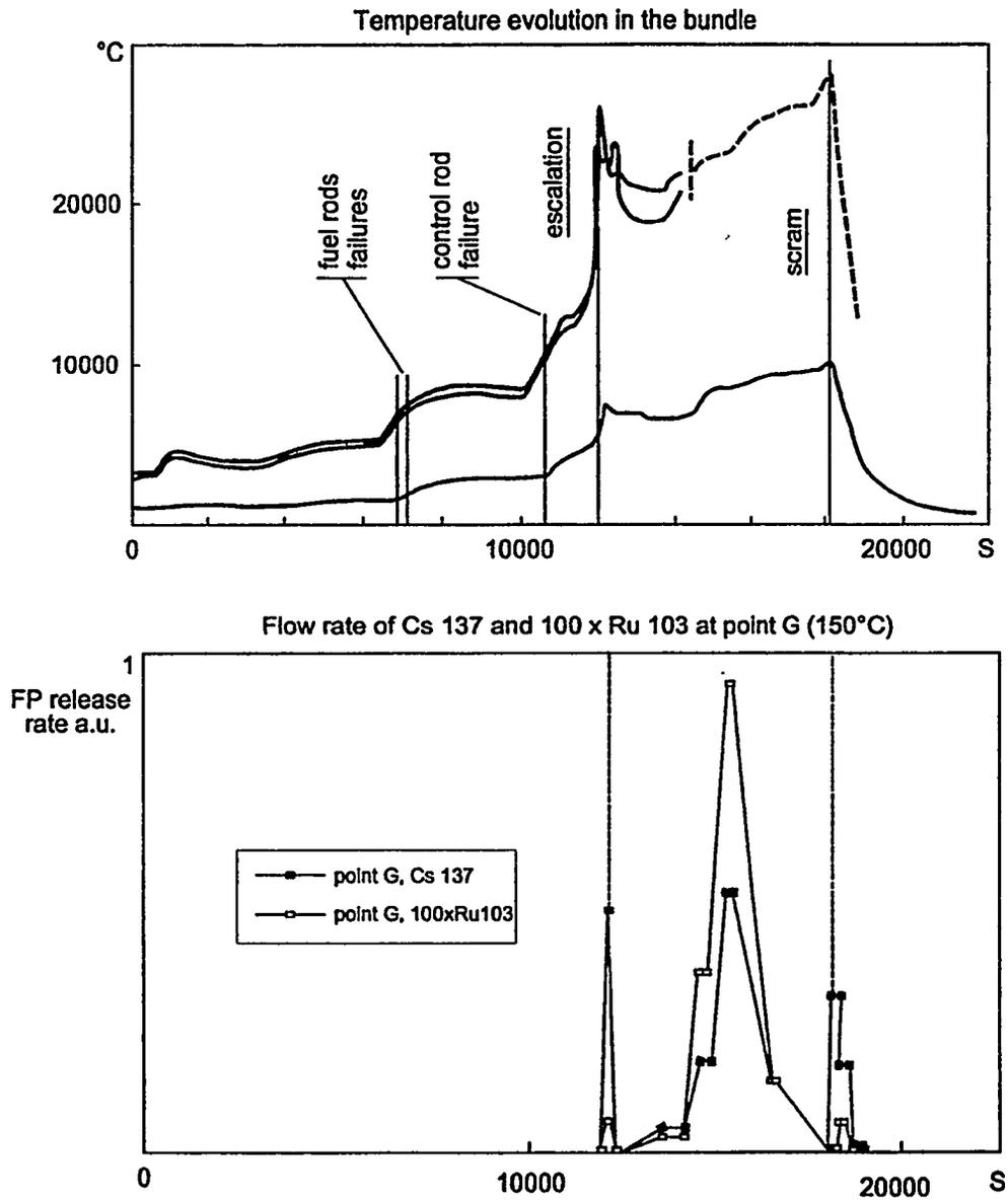
Figure 7 - FPTO FP release correlated to bundle degradation events.
