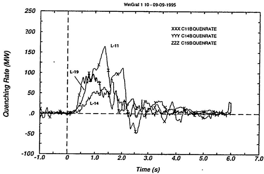
Fig. 1.7 - Comparison of quenching rates in tests L-11, L-14 and L-19
