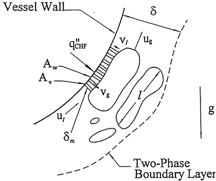
Figure 1. Schematic of the Micro-Layer Underneath an Elongated Vapor Slug.
