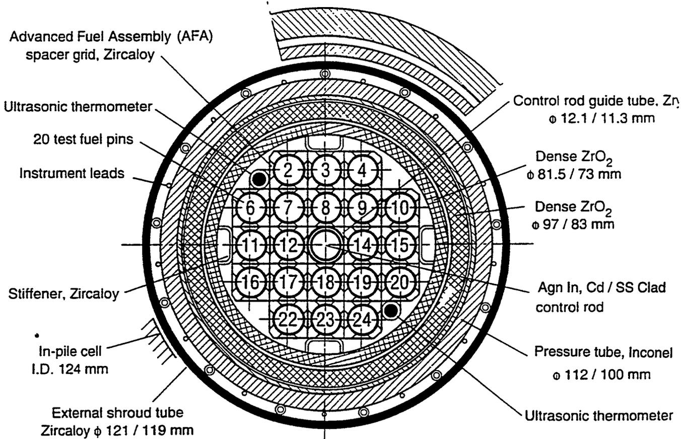
Figure 2 - FPT0 in-pile test section, horizontal section
