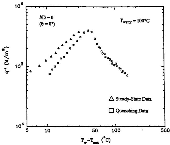
Figure 7. Comparison of the Steady-State and Transient Quenching Data for Water at 100°C.
