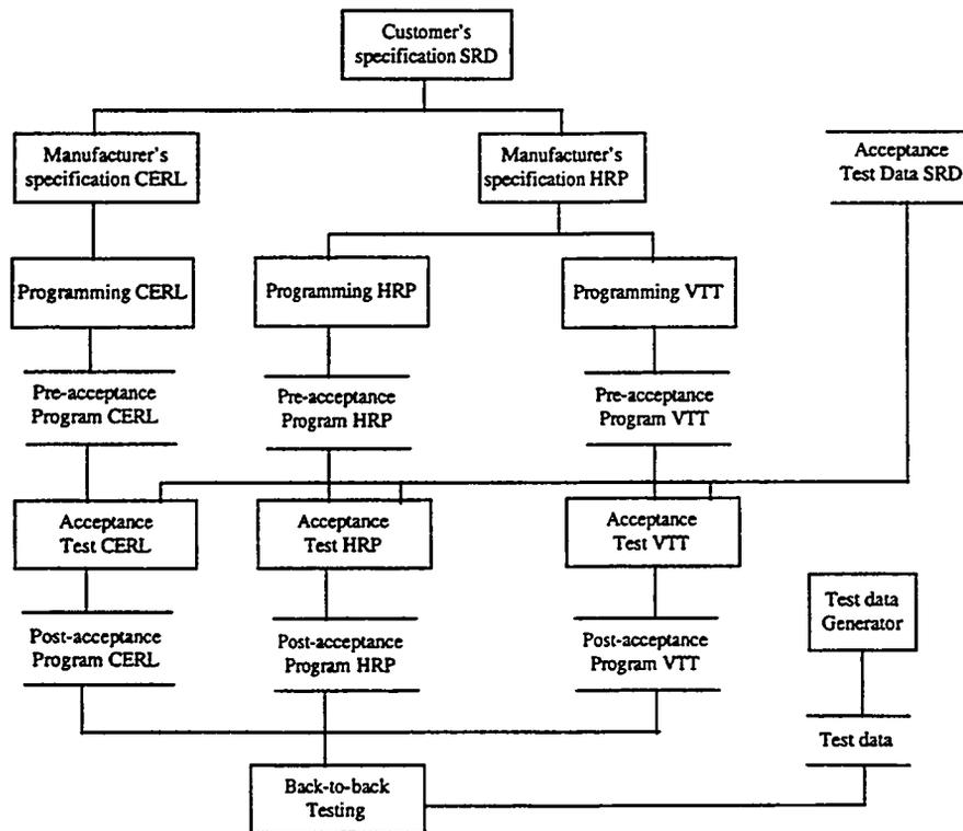
Figure 5. Experimental set-up for first back-to-back test
