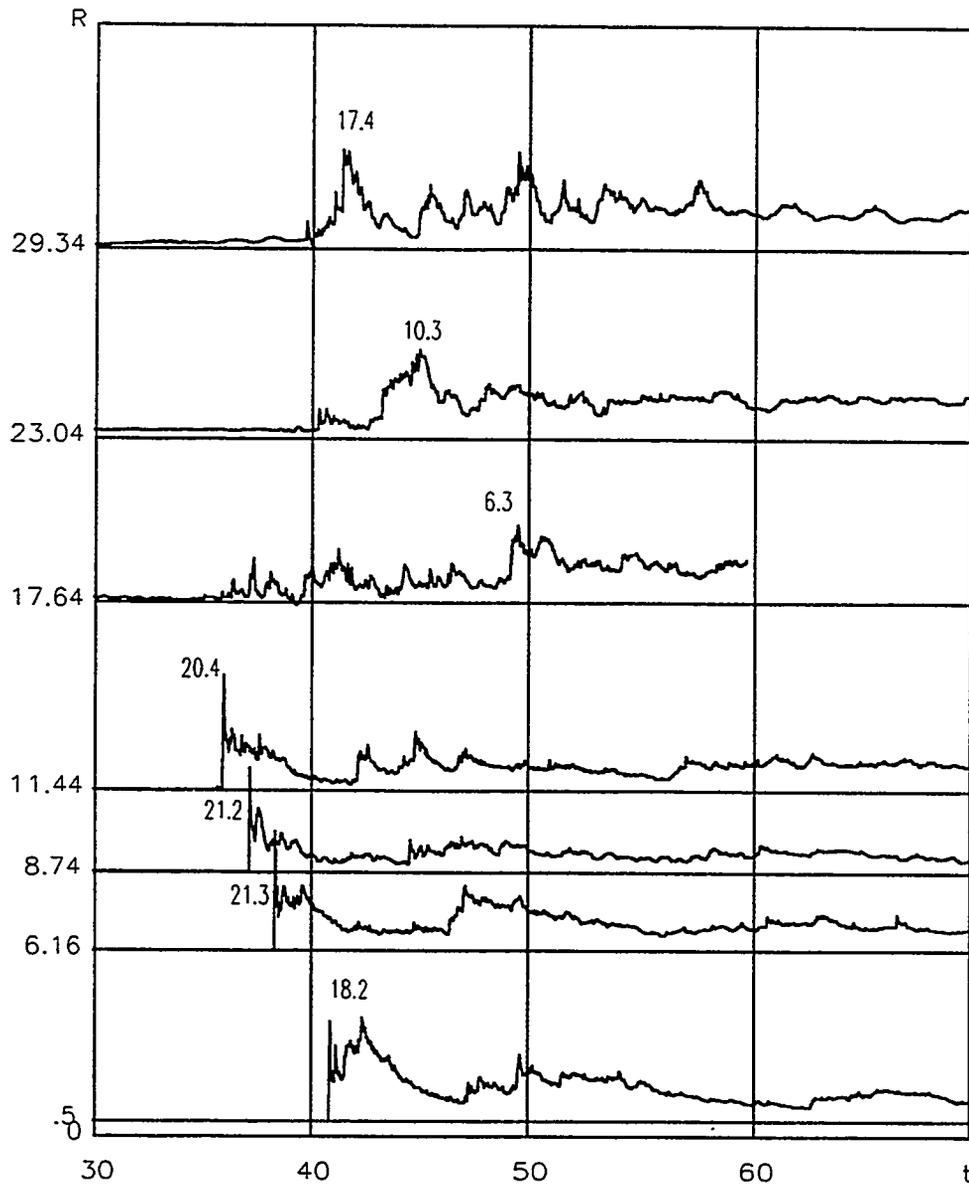
**Figure 4.** (R -- t) - diagram of pressure waves in test 28. R in meters, t in ms. Maximum overpressures (bar) are shown in the plot.
