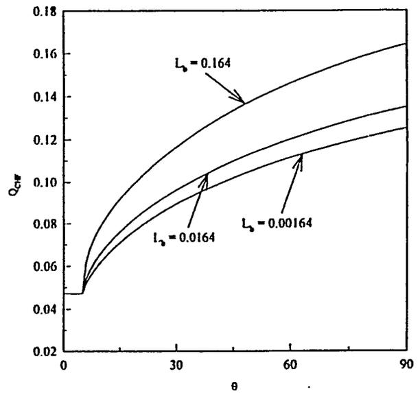
Figure 17. Predicted Variation of the Dimensionless Local Critical Heat Flux.
