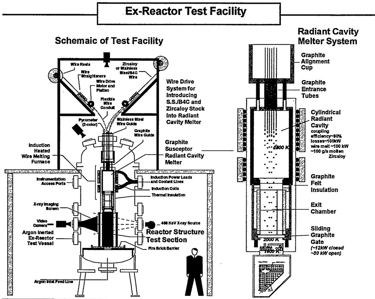
Figure 4: Facility for conducting the Ex-Reactor experiments.
