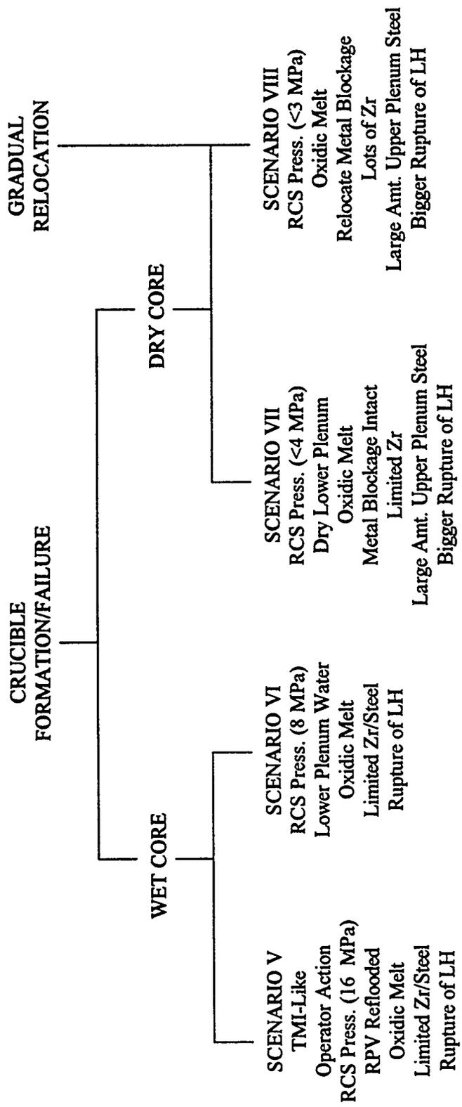
Figure 3. Splinter DCH scenarios reflecting working group recommendations.
