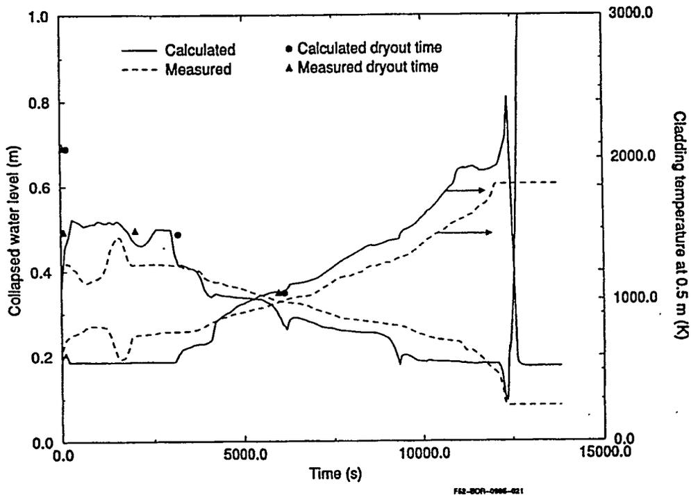
Figure 5 - Calculated and measured water levels and dryout times for the SFD-ST experiment.
