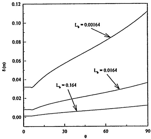
Figure 12. Predicted Variation of the Actual Local Boundary Layer Thickness.
