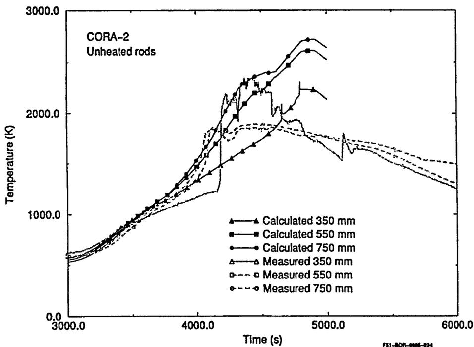
Figure 4 - Calculated and measured bundle temperatures for the CORA-2 experiment.
