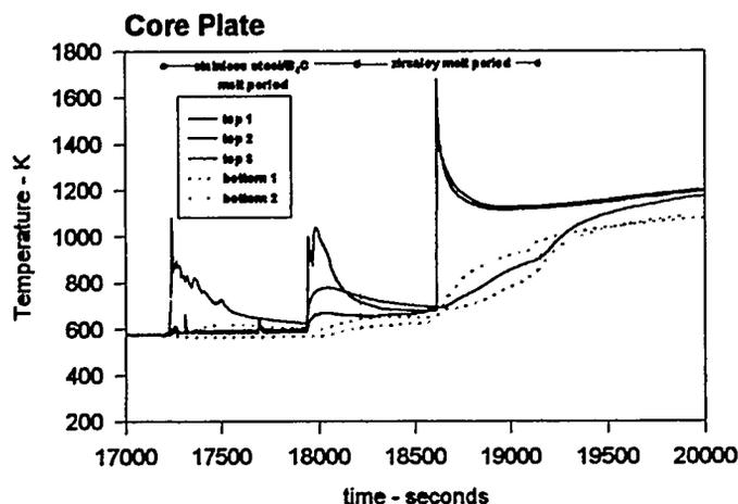
Figure 10. Thermal response of the XR2-1 core plate structure.
