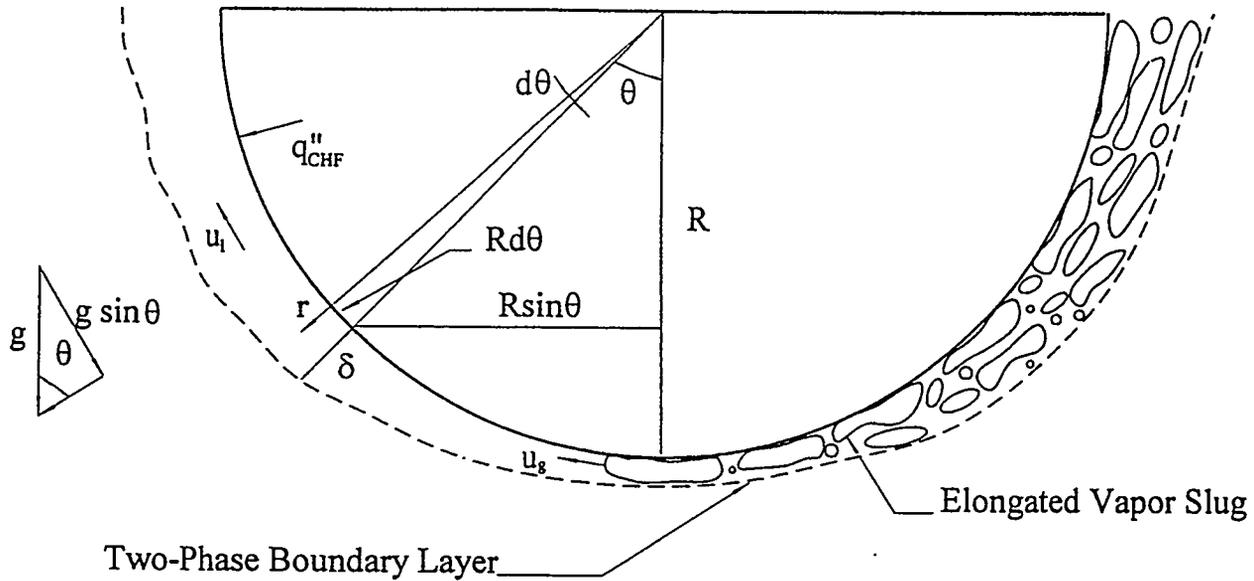
Figure 2. Configuration of the Two-Phase Boundary Layer on the Outer Surface of a Heated Hemispherical Vessel.
