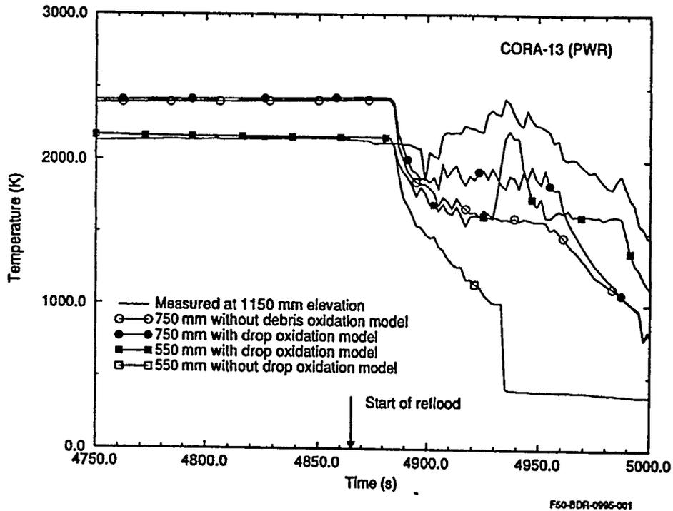
Figure 3 - Calculated and measured bundle temperatures during the reflood phase of the CORA-13 PWR experiment.
