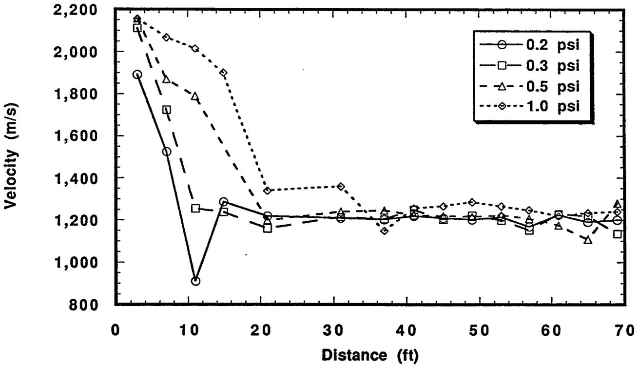
Figure 3: Effect of driver partial pressure (or length) on detonation transmission in an 8 percent hydrogen and 92 percent air mixture at 650K and 0.1 MPa
