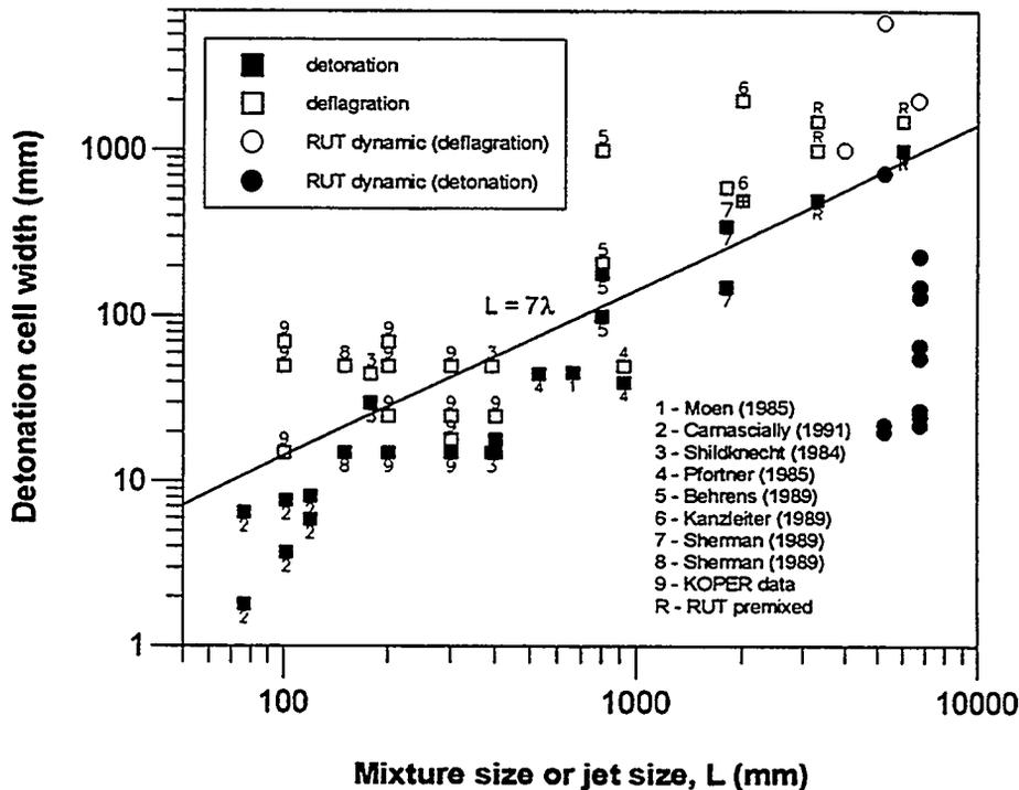
Figure 1. Experimental data on turbulent jet initiation and DDT in large confined volumes
