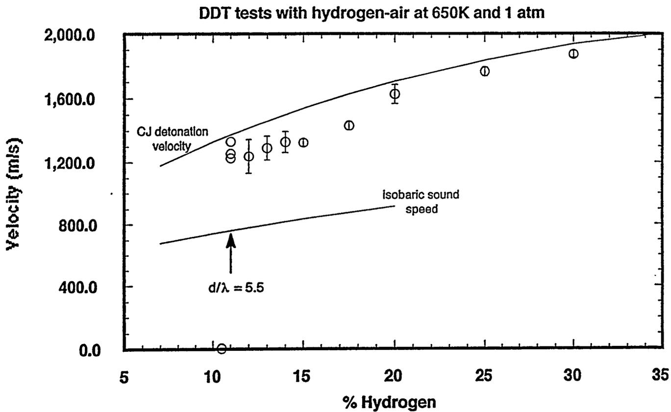
Figure 8: Measured flame velocity vs. gas composition for tests conducted at 650K
