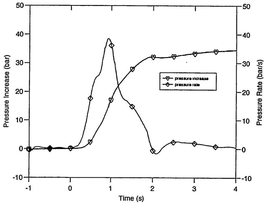
Fig. 1.3 - FARO L-19 pressure increase and rate during the first 4 s
