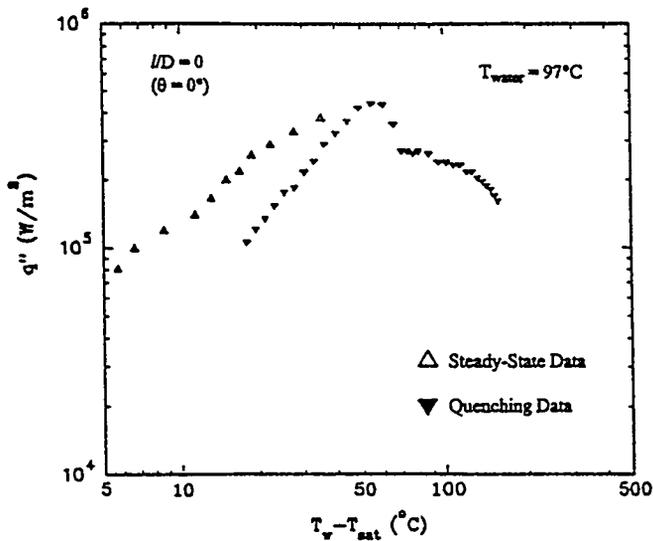
Figure 8. Comparison of the Steady-State and Transient Quenching Data for Water at 97°C.
