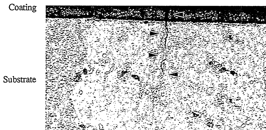
Figure 14. Light micrograph showing crack penetration through aluminide coating, inter-diffusion zone and substrate. \Delta\epsilon_{\text{mech}}=0.5\% , O.P. TMF, \Delta T=900-1600^\circ\text{F} , N_i=360 . Crack length=7.6 mil (193 \mu\text{m} ). (170 X)
