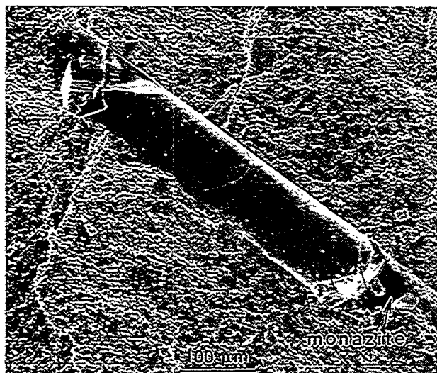
Figure 2: Fracture surface of the RBMO/sapphire-fiber composite.
