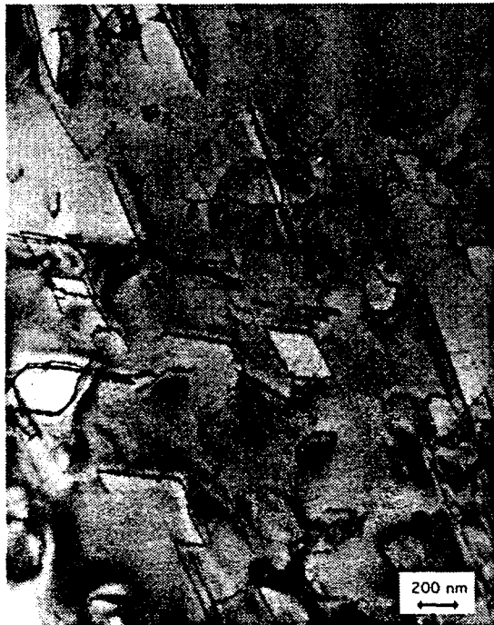
Fig. 7. Higher magnification TEM micrograph of dislocation loops visible in Fig. 5.
