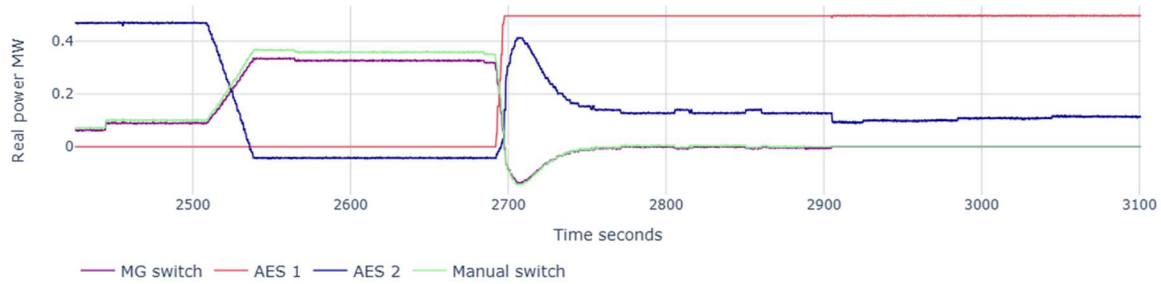
Figure 14. Inverter output powers and the power flow through the breakers feeding the 12-kV bus during planned islanding without the ultracapacitor under night loading conditions.
