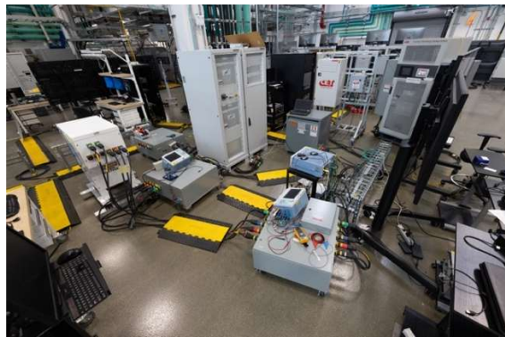
Figure 2. PHIL experimental setup with the inverter on the right (to the left of the large computer screens), the AC source in the center, and the power inductor on the left. Photo by NREL.
