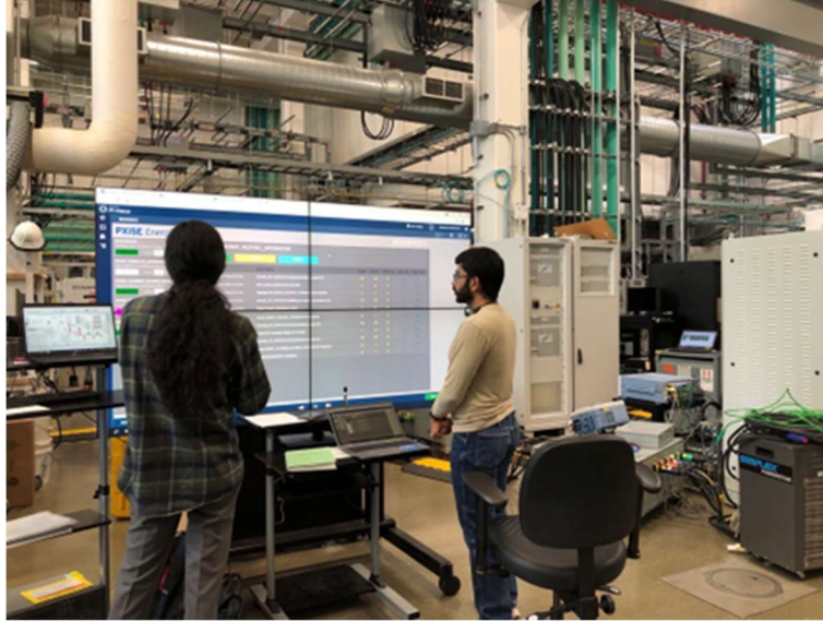
Figure 34: HIL setup operating with CHIL devices and inverter PHIL integration.
