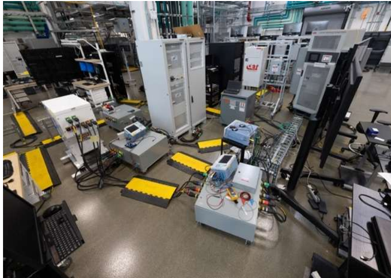
Figure 20: PHIL experimental setup with the inverter on the right (to the left of the large computer screens), the AC source in the center, and the power inductor on the left. Photo by NREL.
