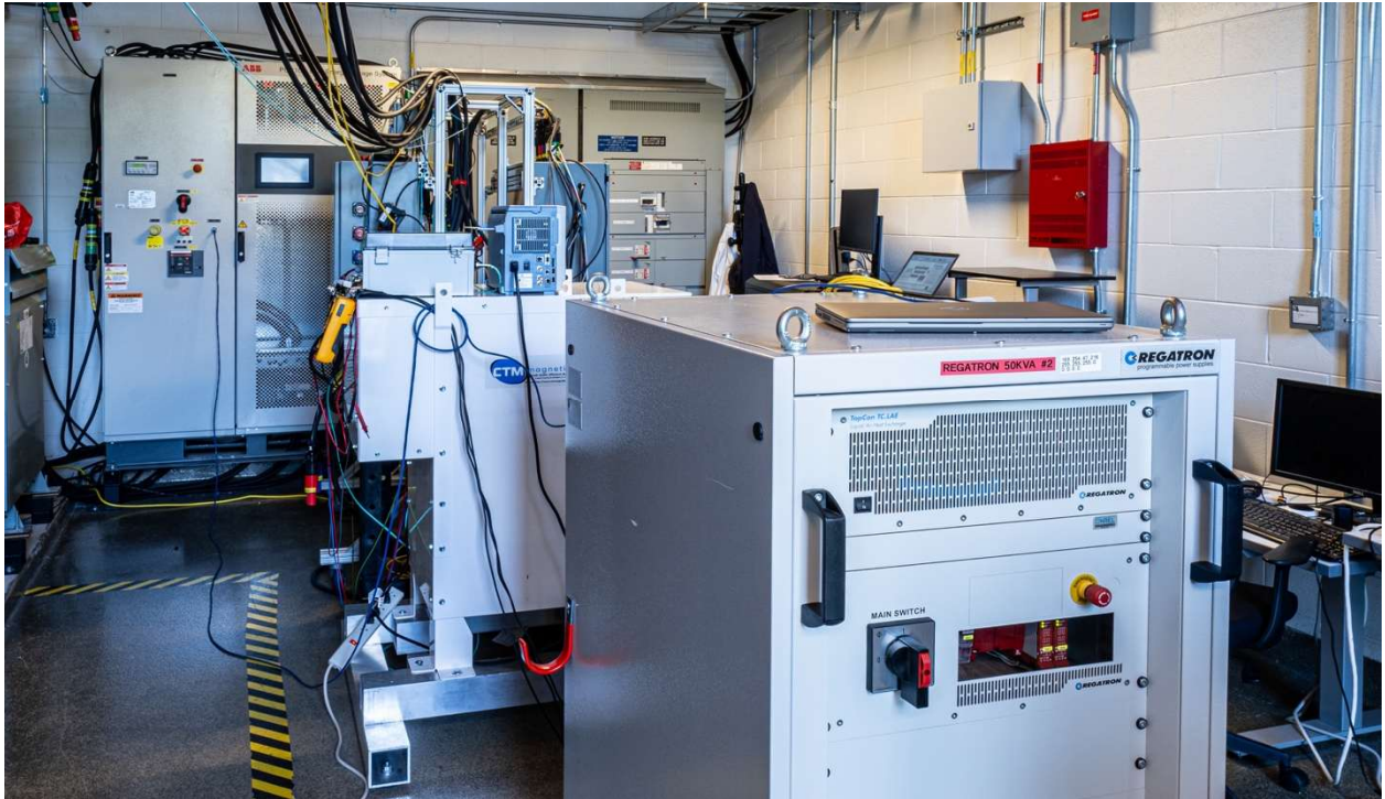
Figure 5. Experimental setup of voltage amplifier interface method. The inverter is in the back on the left, the amplifier is in the front on the right, and the power inductor is between them. Photo by NREL.
