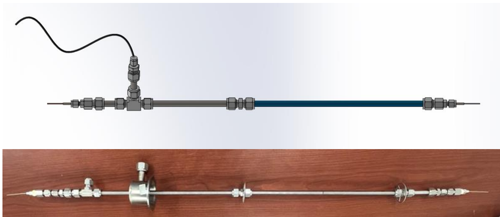
Figure 1. A computer mockup (top) and the first build prototype (bottom) of an internal heater within a 330.2 mm long cladding segment.
