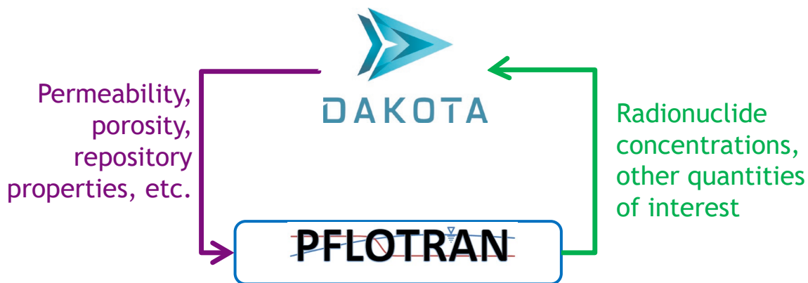
Figure 2-1 Workflow with Dakota driving ensembles of PFLOTRAN simulations
