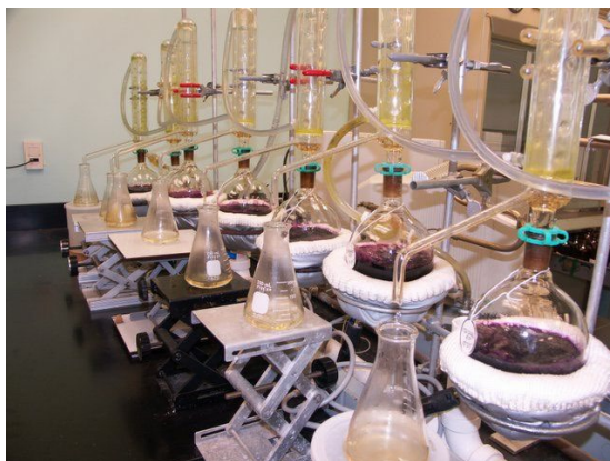
7-2 Distilling Samples for Tritium Analysis Performed at PEARL
