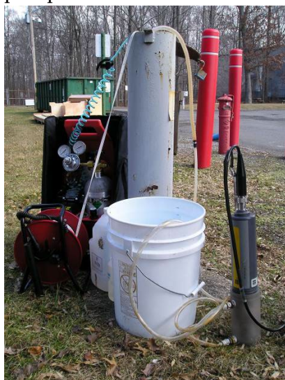
Exhibit 6-5. Well Monitoring Set-Up
