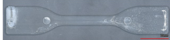
Figure 9. Images of injection molded tensile specimens produced using the (a) mold fabricated by VPP and (b) a metal mold.
