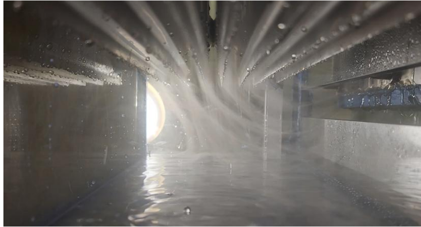
Figure 59: An image of the bottom of the condenser during testing showing air with some moisture content returning to the desorber.
