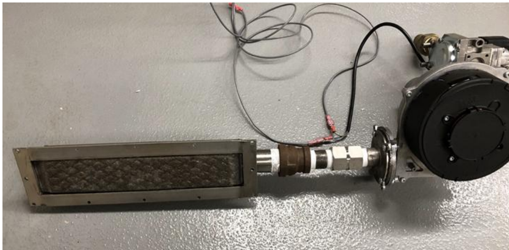
Figure 21: Gas train including sintered metal radiant-style burner.
