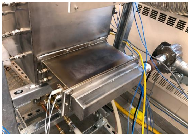
Figure 23: Burner assembly including combustion chamber with flame sensor and hot surface ignitor installed.
