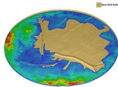
Depth of the waste remaining in AX-102 after 2nd retrieval technology was used
