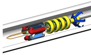
Concept Sketch of modular, low-profile, robotics-enabled inspection system
