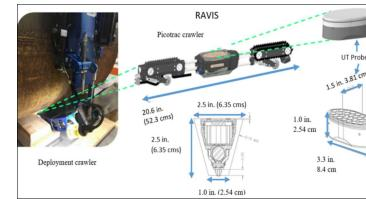
Air-Slot Crawler of the Robotic Air-slot Volumetric Inspection System (RAVIS)
