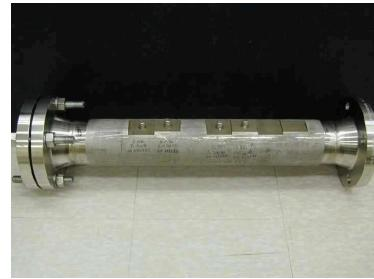
*PNNL-20350: Figure 5.1 PulseEcho Spool Piece with 5-MHz and 10-Mhz Transducers Mounted*
