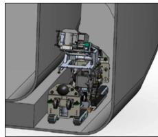
Remote Robotic EMAT Volumetric Inspection System (RREVIS)
