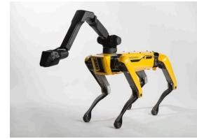
Example Quadruped Robot with a sensor mounted on a manipulator arm
