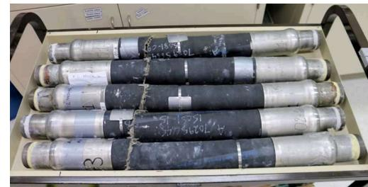
*Inner Hose Specimens post burst test*
