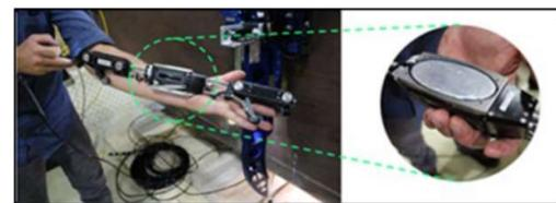
*Guidedwave Phased Array sensor currently in development for under-tank inspection*
