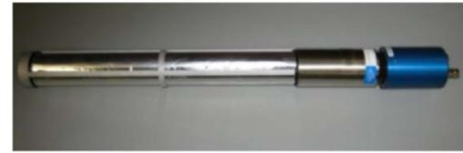
Direct-Push Prototype Beta Detection Probe
