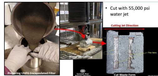
HEPA Filter Waste Form Fabrication and Cross Section Cuts for Characterization
