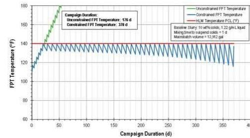
**Campaign Duration vs FPT Temperature for a 1 day Mixing Time to Suspend Solids**
