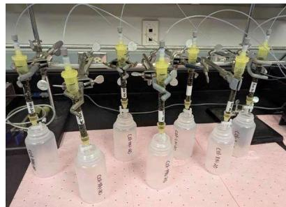
*Columns loaded with IDF soil surrogate for testing of natural abiotic attenuation of nitrate from grout*
