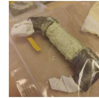
Pipe covered with salt waste simulant for Laser Ablation Testing
