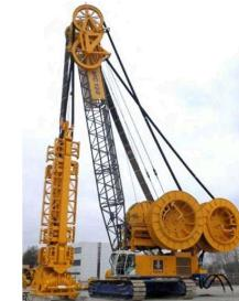
*Cutter Equipment for Vertical Mining Cut-off Walls from Bauer*
