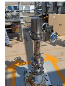
*Shielded Sampler mounted on a mock 4-inch riser at the Cold Test Facility 2021*
