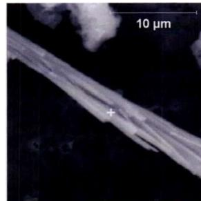
Micrograph of a Pu-Bi Particle.
