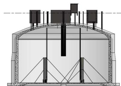
Typical A-Farm Tank Cross-Section Model
