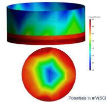
Cylindrical Inert Anode Suspended in Cylindrical Tank
