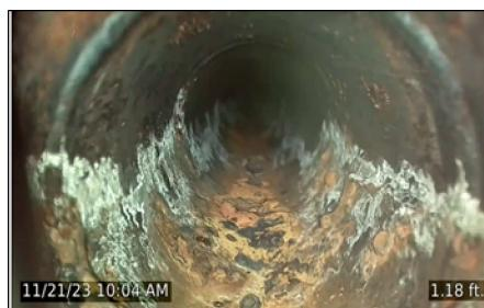
*Transfer Line interior degradation, captured through borescope inspection..*
