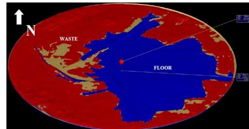
Tank 241-AX-102 Waste Surface Laser Scan (Floor Visible Locations)
