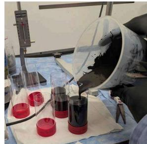
Fresh Grout Poured Into Containers for Curing
