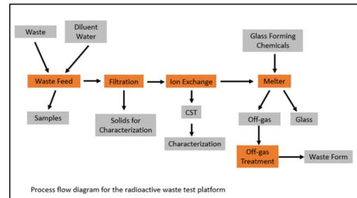
Process Flow Diagram for the Radioactive Waste Test Platform
