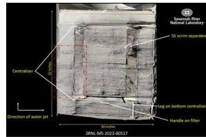
Encapsulated Full-Scale HEPA Filter
