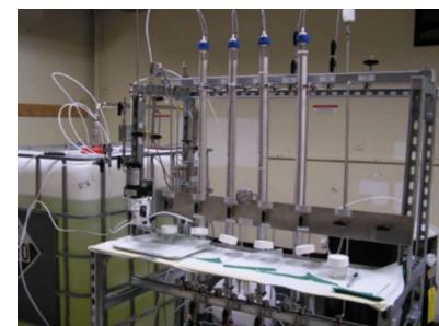
*Packed columns to test removal of COCs from aqueous media*
