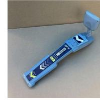
*Radiodetection Device currently used to localize underground wiring***PRELIMINARY COST ESTIMATE AND SCOPE SUMMARY**
