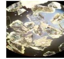
Ground Glass Samples used in Dissolution Rate Tests
