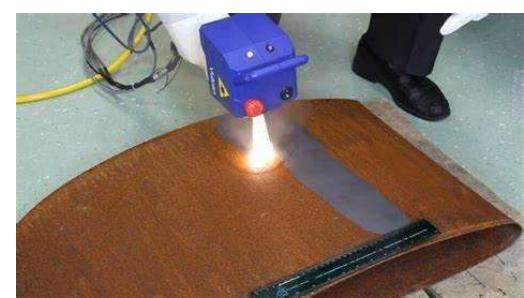
Example cleaning application using Laser Ablation
