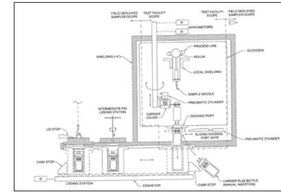
Schematic of the Isolok Sampling System and MSHS Configuration
