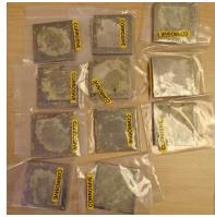
Coupons covered with salt waste simulant for Laser Ablation Testing
