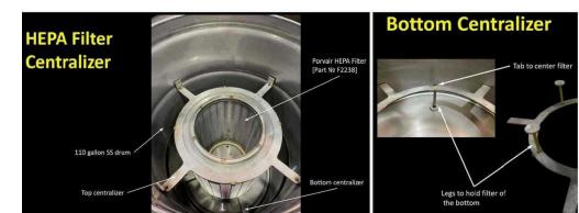
Encapsulation Process of HEPA Filter
