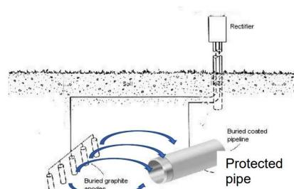
Diagram representing Active Cathodic Protection for Transfer line corrosion prevention.
