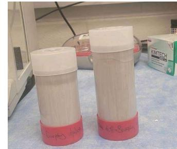
Cured Grout to Undergo Disposal Property Testing
