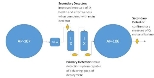
*Multiple Detectors in an Integrated Feedback System*
