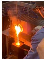
Molten Glass Test Waste Form being Poured
