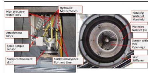
*Early stages of development simulant retrieval with HWEE mounted on X/Y scanner*
