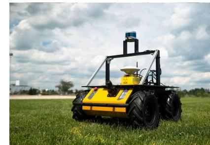
*Husky Autonomous Instrumented Vehicle by Clearpath*
