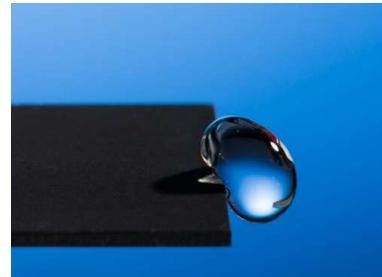
Water repelled by laser treated surface
