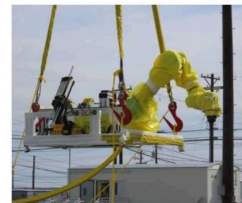
Robotic arm with tooling designed for pit work.
