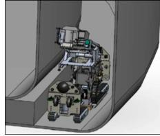
*Rendering of the Remote Robotic EMAT Volumetric Inspection System currently in development*
