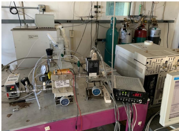
Figure 10: Experimental setup for H 2 crossover measurement using gas chromatography for ex-situ method at LANL
