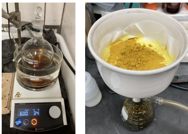
Figure 13. Left: Reaction setup employed for the synthesis of HAH, showing the glassware configuration used during the reaction. Right: Image of the isolated HAH product collected in a Büchner funnel, illustrating its solid, yellow appearance upon filtration.
