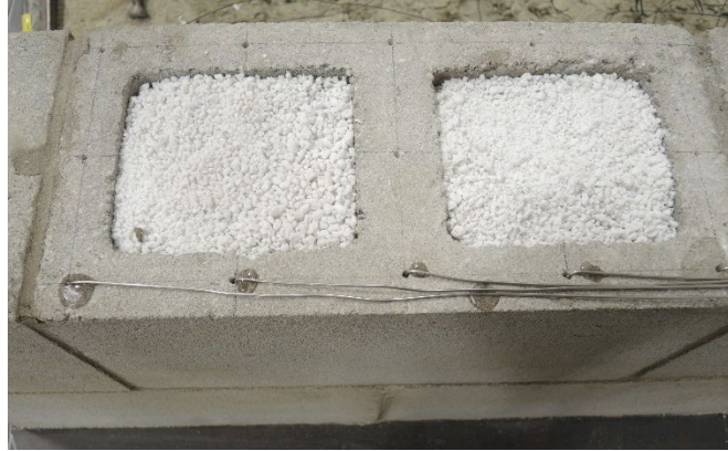
Figure 4-14: Thermocouples inserted into holes drilled in masonry block filled with perlite
