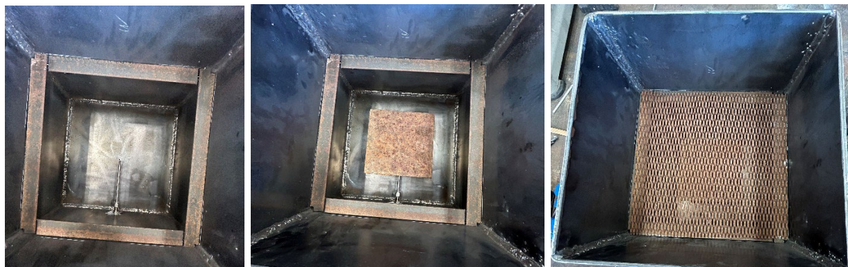
Figure A- 6: Top view of gas burner showing (a) inlet (b) diffuser, and (c) screen to support crushed rock.
