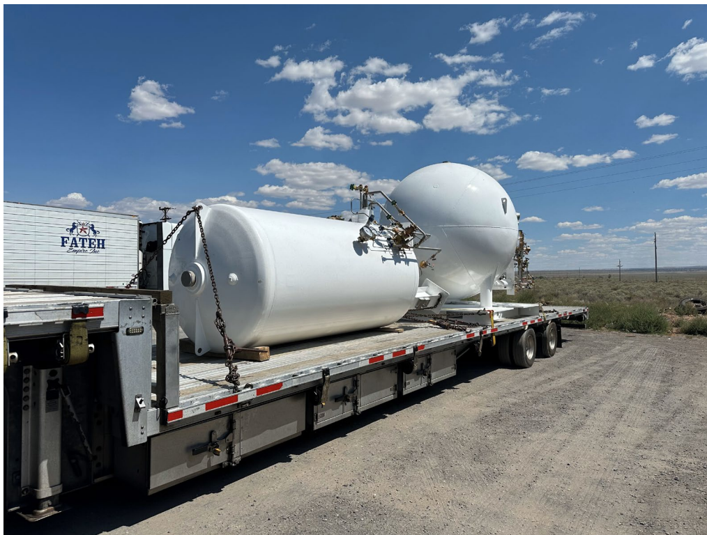
Figure 2-8: Vertical cryogenic tank for fireball experiments and LN 2 tank.
