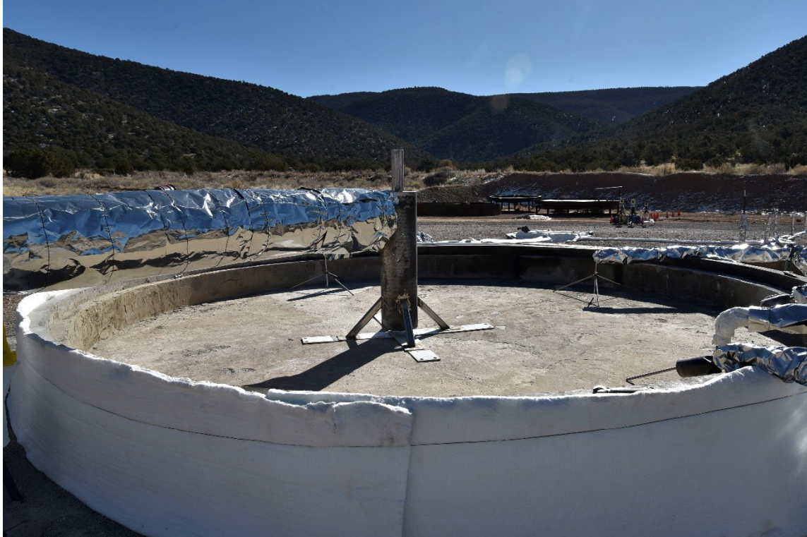
Figure 2-6: Diffuser attached to pipeline for pool fire experiments.
