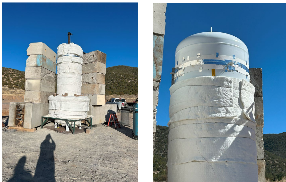
Figure 2-16: Propane tank containing isopentane for fireball experiment: (a) insulated tank and heaters, (b) additional thermal protection at LSC location.
