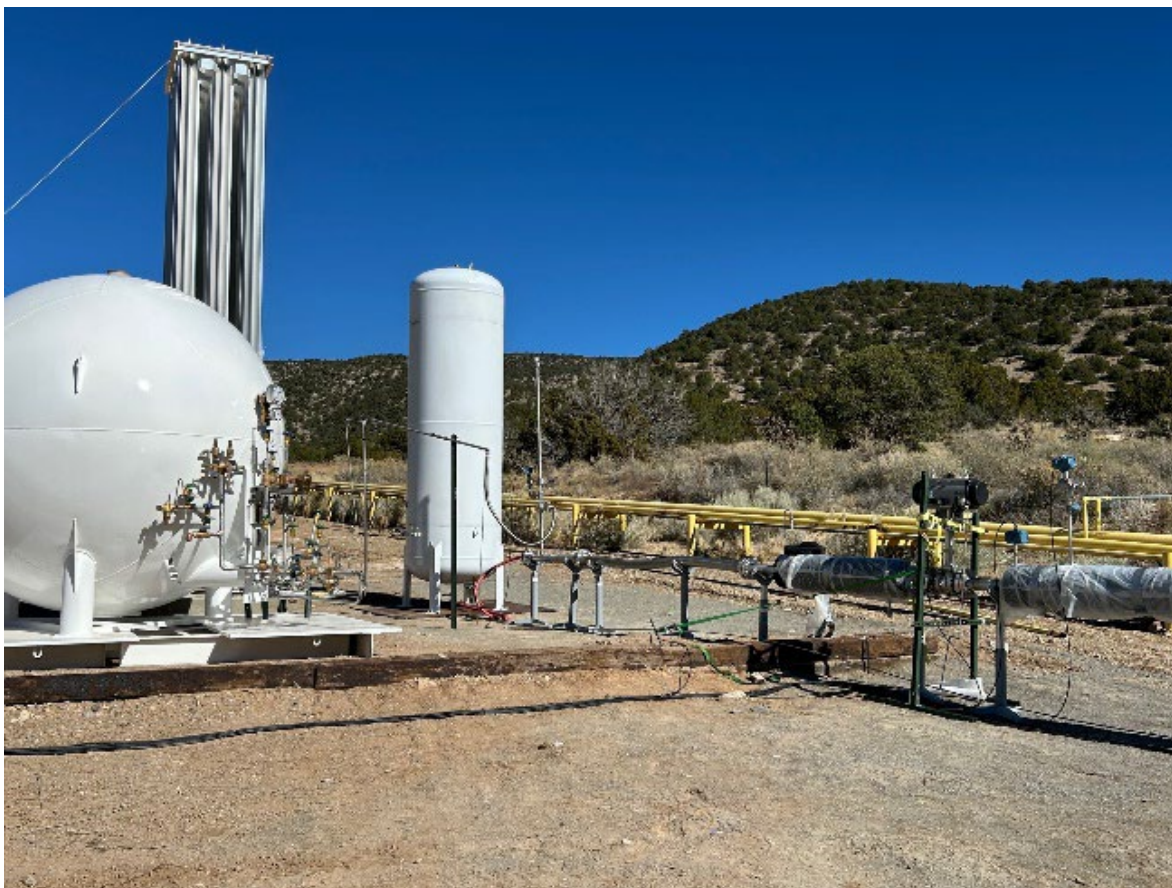
Figure 2-4: Arrangement of iso-pentane jet fire experiment with the 1150-gallon vertical propane tank next to the 1000-gallon spherical LN 2 tank and vaporizer.
