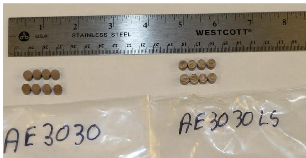
Figure 1. AE3030 and AE3030LS material samples used in this study. Note: samples prepared by Matt Selter (KCNSC).
