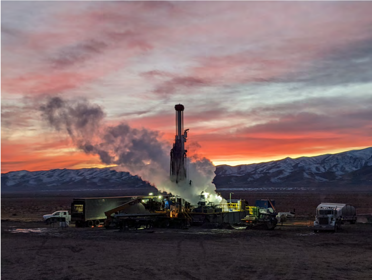
Figure 84. Experimental geothermal injection at San Emidio well 58B-33 flowing at 250 gallons/minute during rig development (Matt Folsom 2020/12/22).
