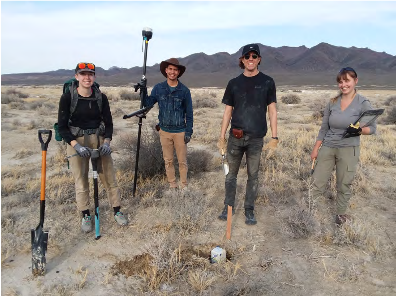
Figure 88. Planting a seismograph, just before filling in the hole to improve coupling between the sensor and the earth, removing the stake to reduce wind noise, and dusting off the top of the instrument to improve the reception of GPS signals. From left to right, Anya Wolterman, DJ Bustos, Ben Jahnke, and Samantha Kleich.
