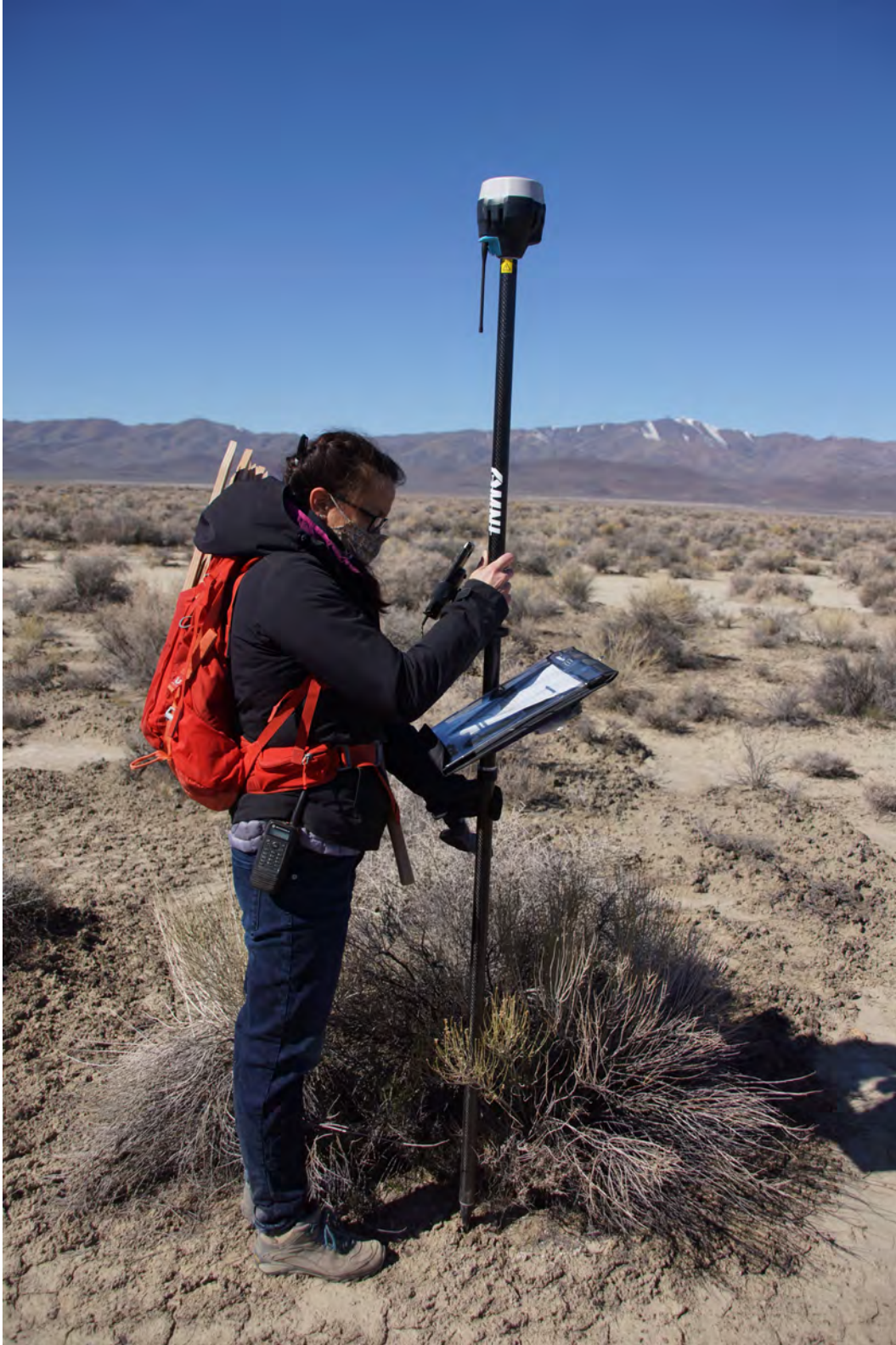
Figure 86. Erin Cunningham staking the location of a seismic station with real-time kinematic GPS in March 2022 (photo Neal Lord).
