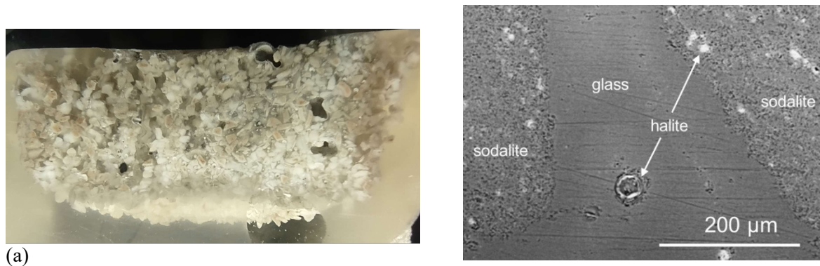
Figure 8. Optical photos and SEM photomicrographs of SCWF materials showing generation of sodalite microencapsulated in glass: (a) SCWF-1, (b) SCWF-2, (c) SCWF-3, and (d) SCWF-4.
