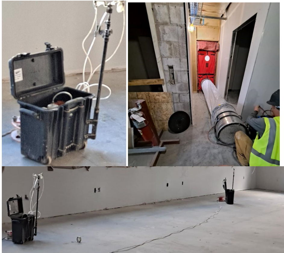
Figure 7. Aerosol sealing station and blower door equipment.
