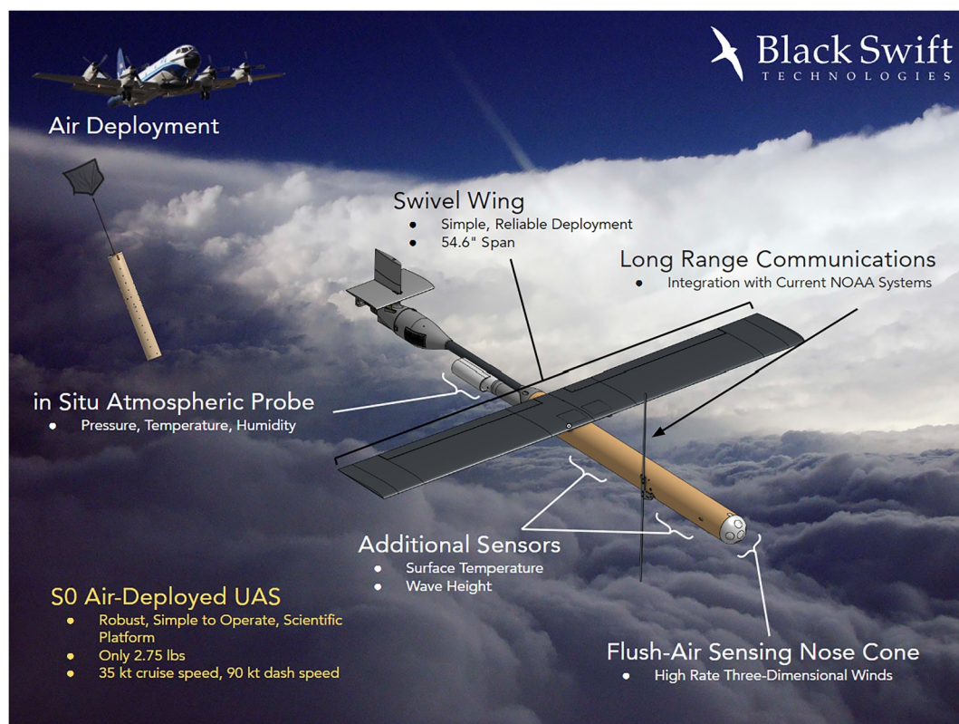
Figure 1. A schematic description of the Black Swift S0 and its deployment from the NOAA P-3.
