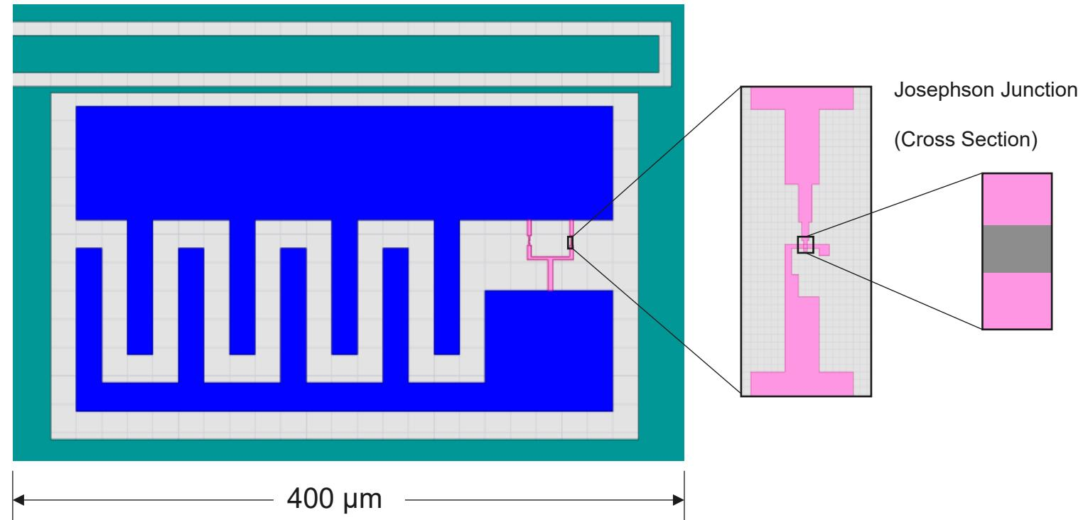
$\hbar\omega_{01} \approx 5 \text{ GHz} = 240 \text{ mK} > 10 \text{ mK}$  (operating temperature)
